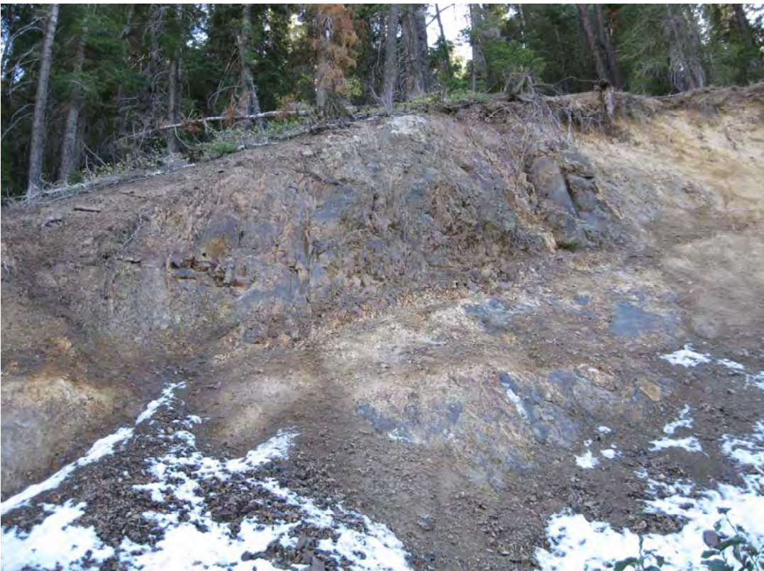
Altered Trachyte in the eastern side of Slope 27. The Trachyte is blocky to massive.
