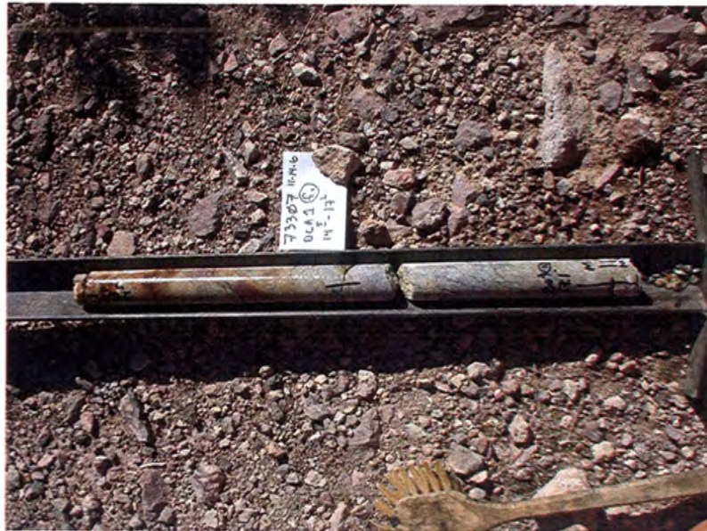
Cored Bedrock from Borehole DCA1 with excellent RQD (90 – 100%)
