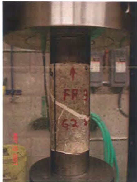
Unconfined Compressive Strength testing of a rock core Core shows gypsum healed joint
