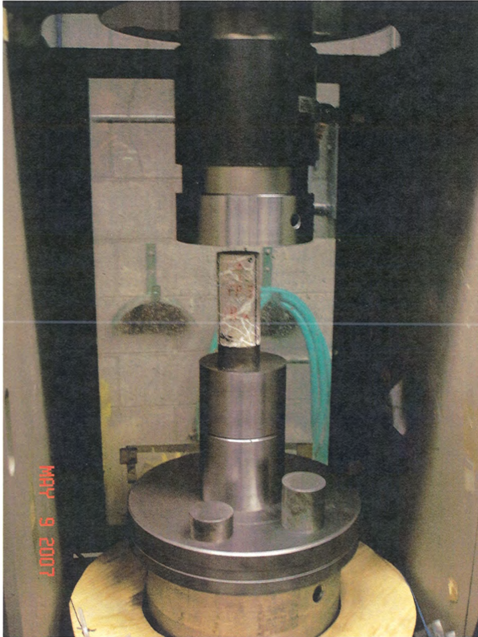
Unconfined Compression Strength testing of a rock core Rock Mechanics Laboratory – University of Nevada-Reno
