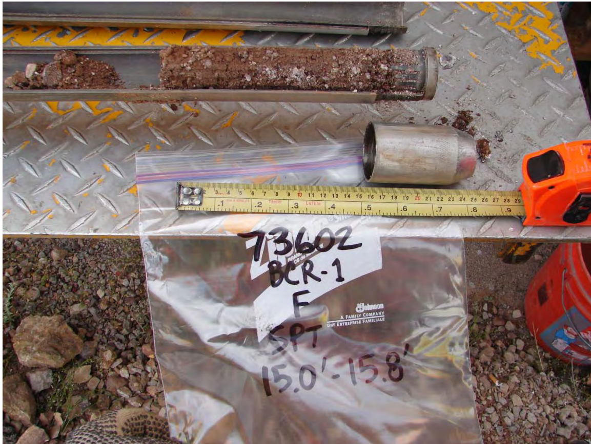
Photos 3 and 4. Drilling sample from Borehole BCR-1
