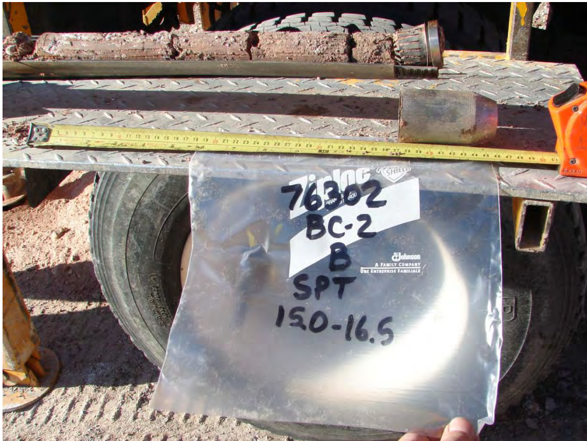
Photo 3. Drilling sample from Borehole BC-2
