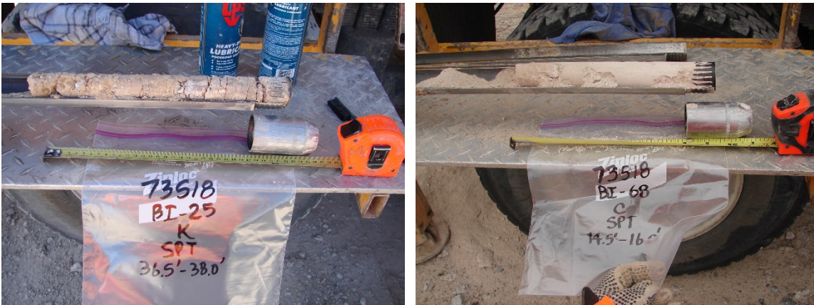
Photos 1 and 2. Soil Samples from Boreholes BI-25 (Clayey Sand with Gravel) and BI-68 (Sandy Lean Clay with Gravel)
