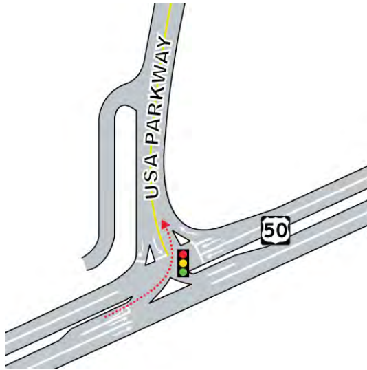
Figure 2-6. High-T Intersection Design
