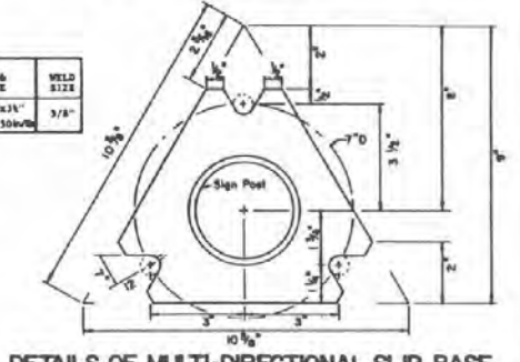
DETAILS OF MULTI-DIRECTIONAL SLIP BASE
