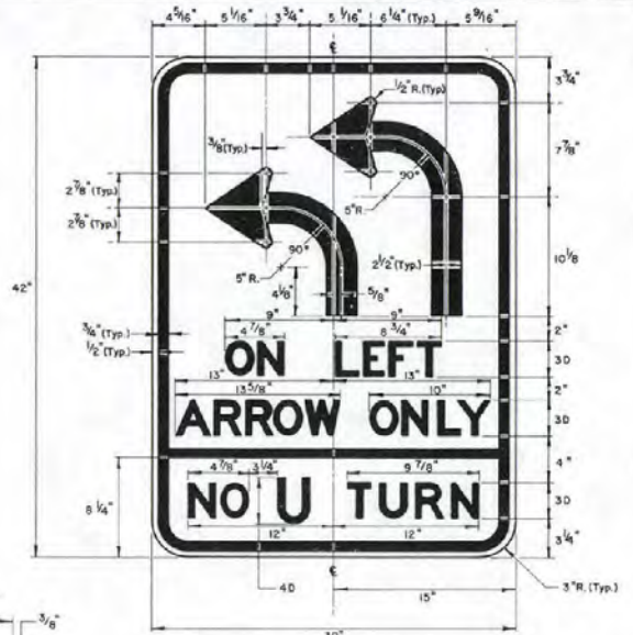
DETAIL "H" SIGN R3-8(S) BACKGROUND - WHITE (REFL.) LEGEND, BORDER - BLACK (NON-REFL.)
