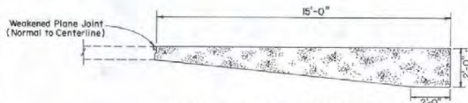
PAVEMENT END ANCHOR DETAIL
