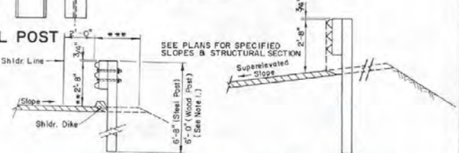
TYPICAL GUARDRAIL INSTALLATIONS
