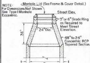
SECTION B-B TYPE I MANHOLE CONCENTRIC
