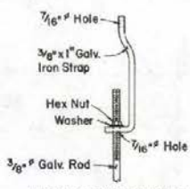
TRUSS TIGHTENER DETAIL B
