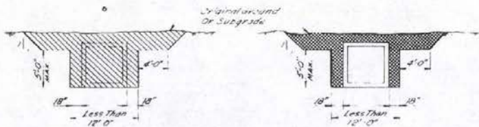
CULVERT IN EXCAVATION
