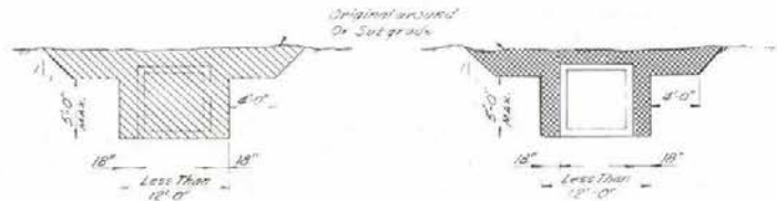
CULVERT IN EXCAVATION
