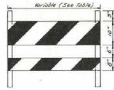
TYPE II BARRICADE (FRAMEWORK TO BE PAINTED WHITE)
