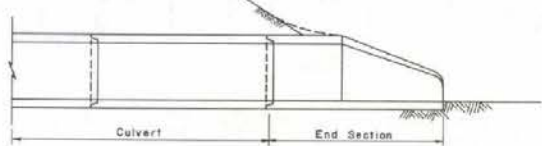
CROSS SECTION VIEW 18" RCP TO 54" RCP
