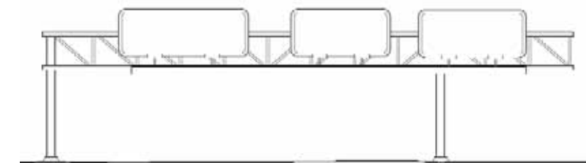
(5) Sign bridge with numerous trusses are visually cluttered.
