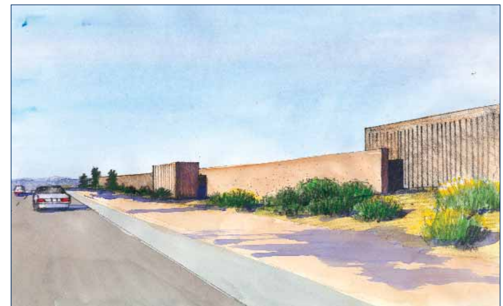
(3) This sequence of travel over approximately 1000 feet illustrates the sound wall design for the corridor. Characteristics include staggered wall planes, landscape planting in front of the wall face, and patterning on the wall face.
