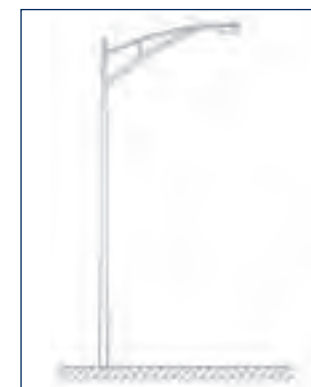
(4) Avoid this type of pole design in favor of more streamlined attachments.
