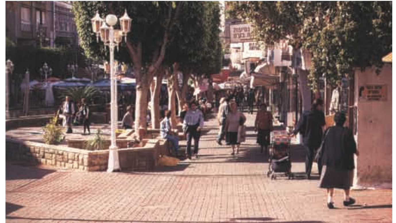
(8) Raised planters separate sidewalk areas from travel lanes and can provide seating opportunities.
