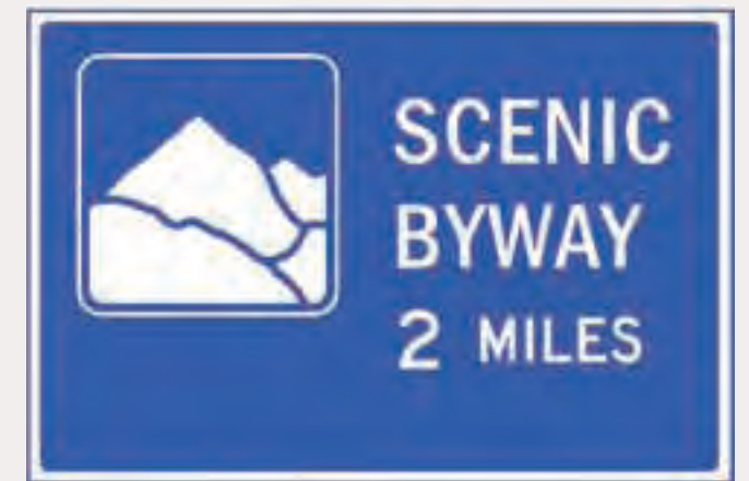
(1) Scenic byways should include a specific pictorial graphic that is related to the place, as part of the Statewide Place Name Sign Program.
