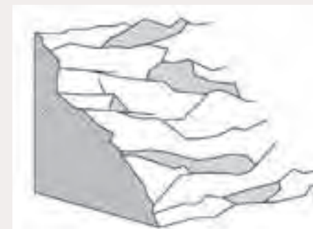
(4) Preferred custom benching, following the natural formation of the rock and accomplishing the same elevation change as shown in illustration 1.
