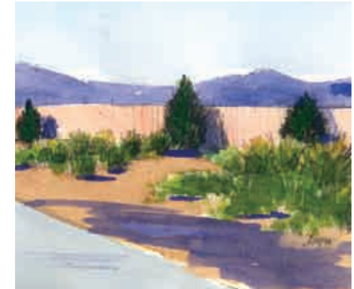
(2) Integrate noise walls into highway right-of-way with landscape planting between wall and roadway. The setback also allows earth contour grading to vary the wall heights and base grade.
