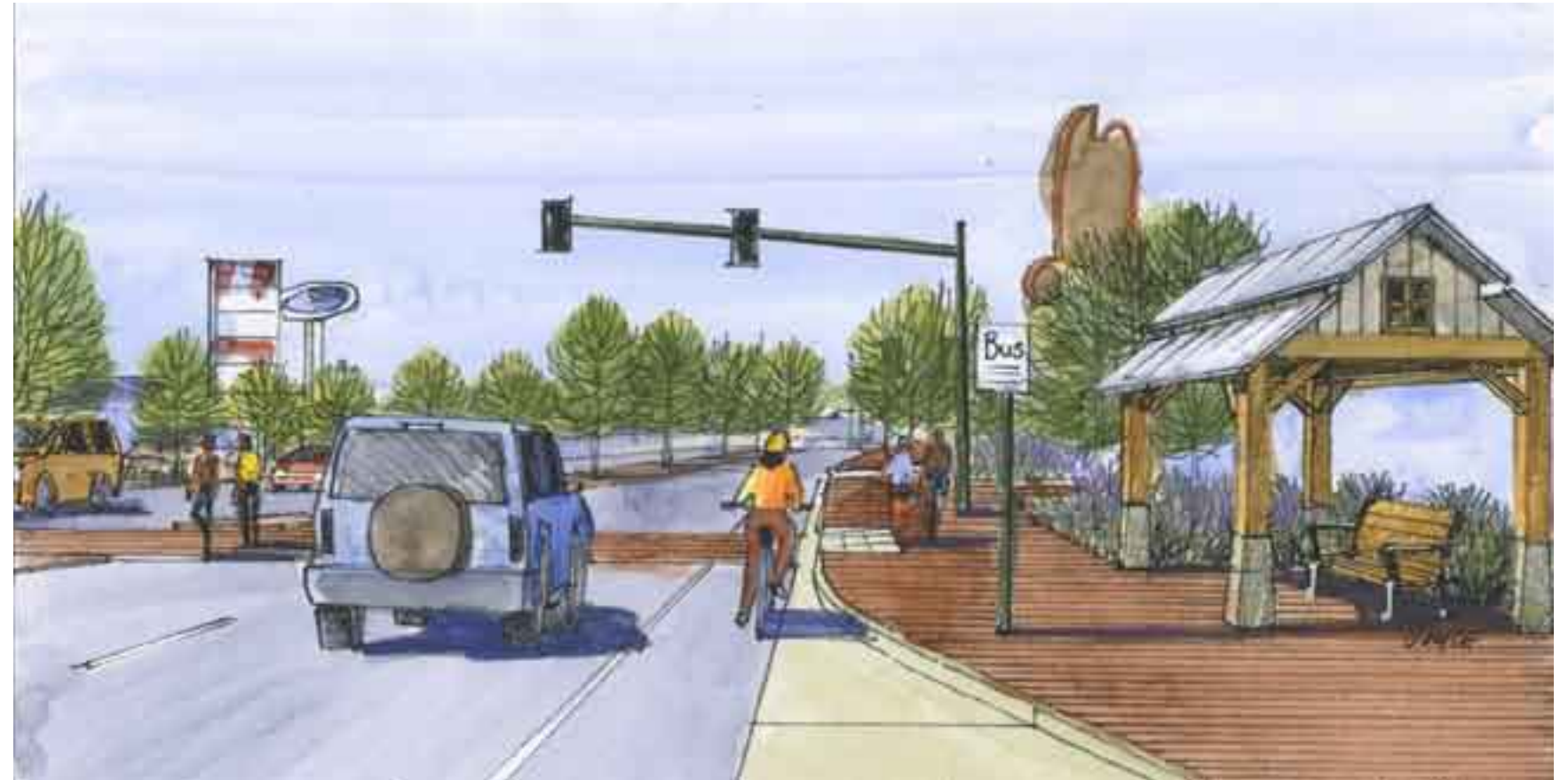
(2) Including transit stops and accentuated crossing points within transition zones increases pedestrian activity. The consolidation of curb cuts provides opportunities for a raised median to visually enhance wide rights-of-way.
