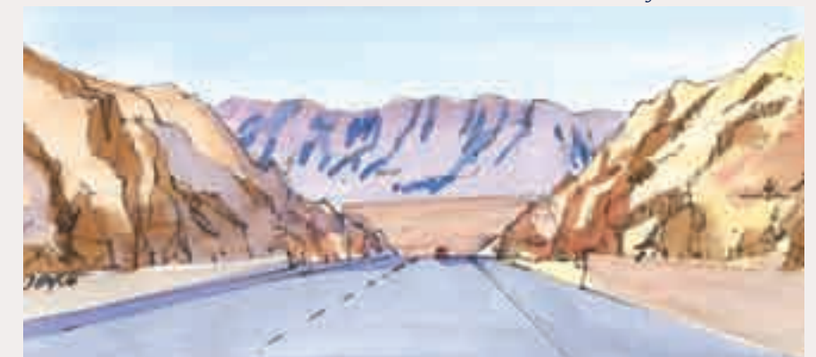
(5) Preferred re-sculpted rock cut changes artificial slope banks into naturally occurring landforms. Plan cuts that terrace, bench, and use bedding planes found in rock formations are the final design of any rock slope.
