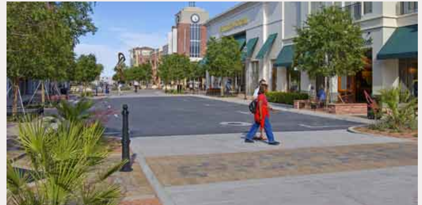
(3) Use of colored paving at pedestrian crossings elevates the importance of the pedestrian.
