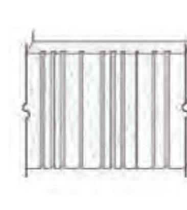
(3) Preferred prototypical surface pattern is rusticated variable vertical ribbing. Dimensions vary between 2"-8" apart.
