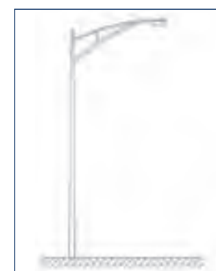
(4) Avoid this type of pole design in favor of more streamlined attachments.
