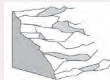
(4) Preferred custom benching follows the natural formation of the rock and accomplishes the same elevation change as shown in illustration 1.
