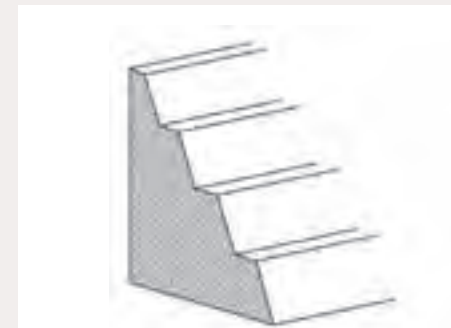
(1) Avoid straight cuts and benches with custom naturalized cuts.
