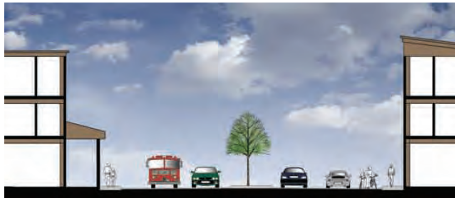
(2) An 80' right-of-way accommodates dual travel lanes and a planted median. A striped bike lane accommodates cyclists through the community center. Pedestrian amenities may be enhanced with widened sidewalks.
