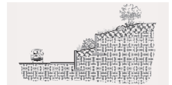
(3) Preferred designs incorporate a step or change of plane for a retaining wall greater than 14 vertical feet.
