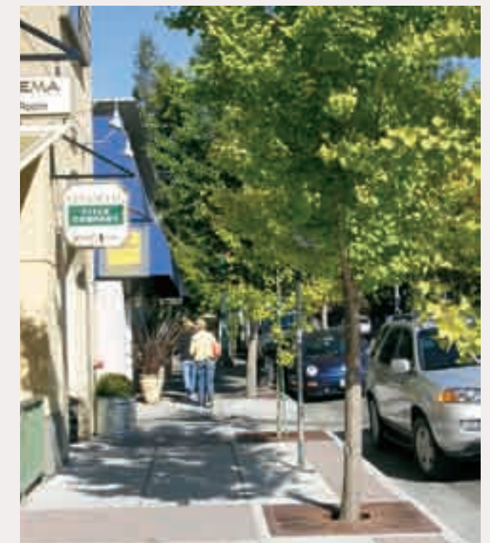
(3) The primary design objective for community interface zones is the highway's ability to accommodate a variety of town-center activities without reducing its function as a through street. On-street parking buffers pedestrians from travel lanes and helps slow traffic through town.
