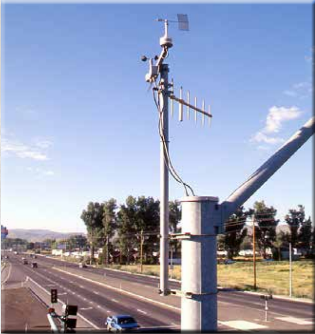
Road Weather Information Systems were placed on major highways and arterials in the 1980s. They transmitted weather and road conditions to better prepare NDOT crews for adverse conditions
