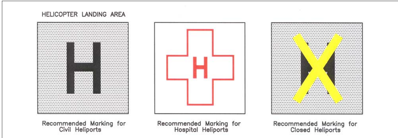
FIG 2-3-23 Helicopter Landing Areas
