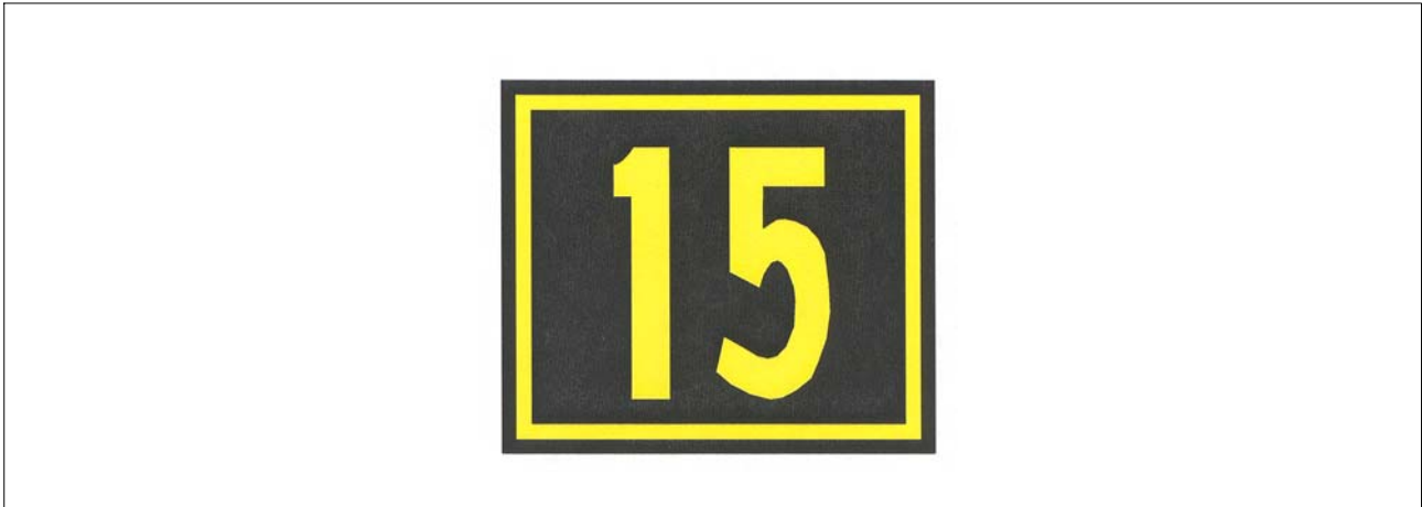
FIG 2-3-32 Runway Location Sign
