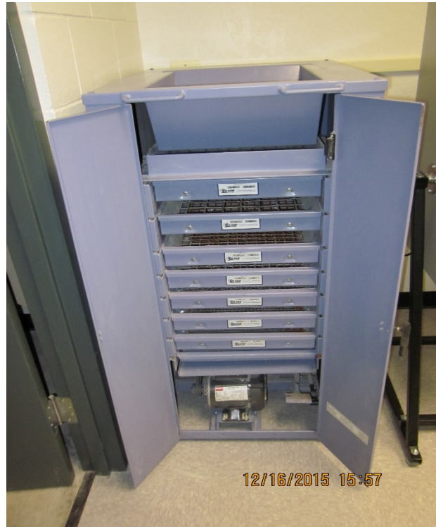
Figure 4 Large Test Master – Mechanical Shaker
