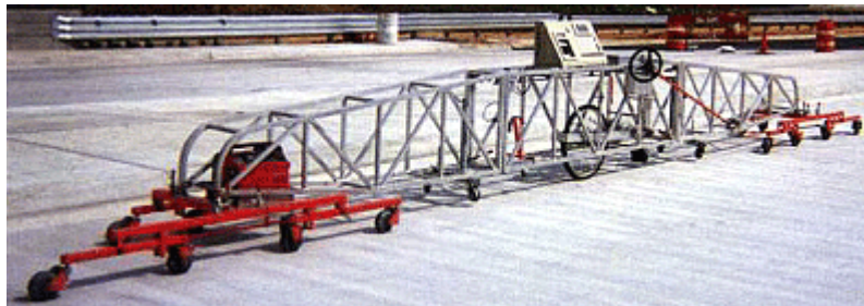
Figure 8: California type profilograph
