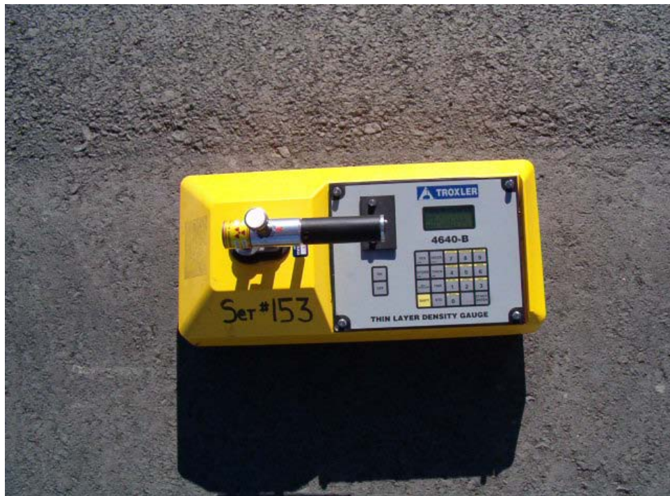
Thin layer density gauge positioning for one joint density test location.
