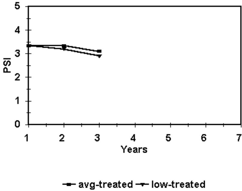
Figure 11. Average and low values of PSI for untreated and lime-treated mixtures on SR 663 in north-western Nevada.
