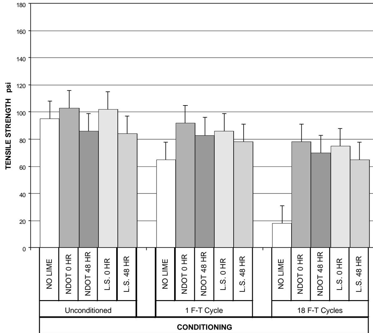
Figure 17. Average tensile strength property of the Lockwood PG 64-34 mixtures, vertical bars indicate the range of average value plus one least significant difference.
