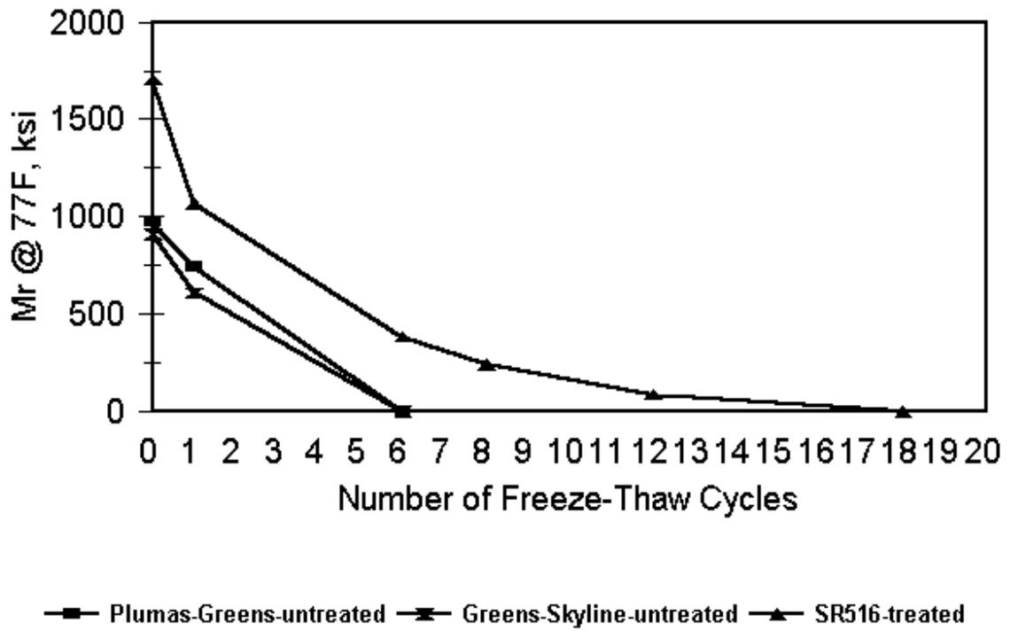
Figure 3. Mr property of field cores at various freeze-thaw cycles for the McCarran Boulevard and SR 516 projects.
