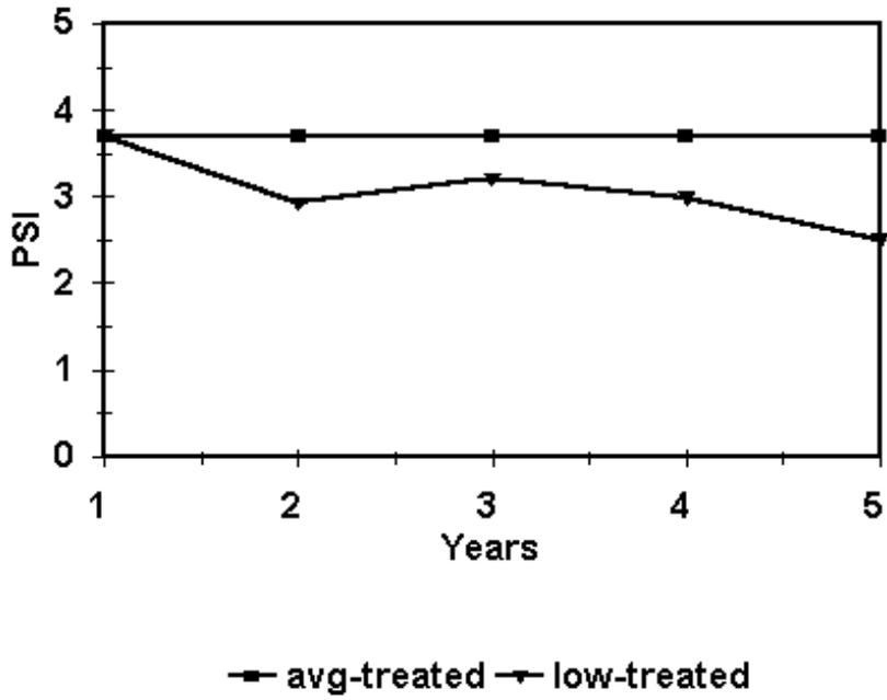
Figure 9. Average and low values of PSI for untreated and lime-treated mixtures on I-80 (2) in north-western Nevada.
