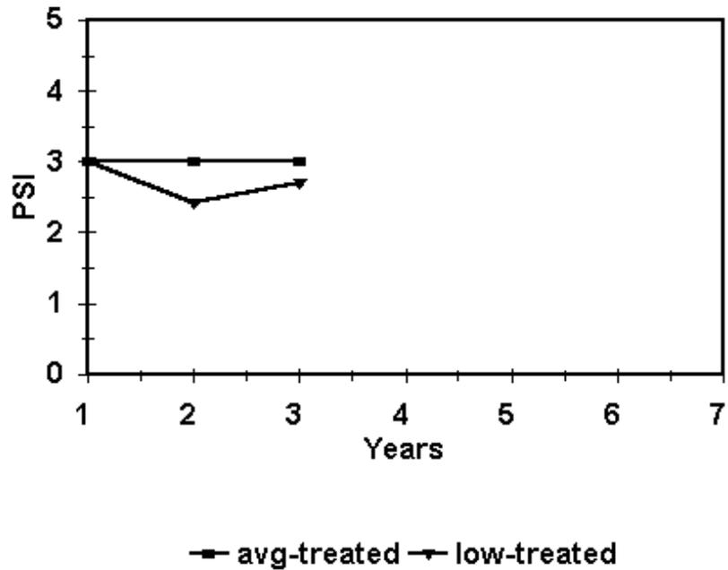
Figure 10. Average and low values of PSI for untreated and lime-treated mixtures on US 395 in north-western Nevada.
