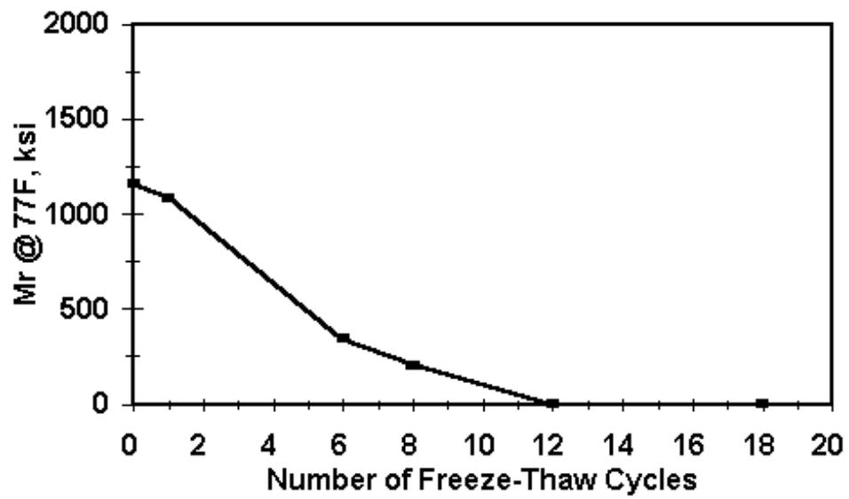
Figure 4. Mr property of field cores at various freeze-thaw cycles for the Sahara Avenue project.
