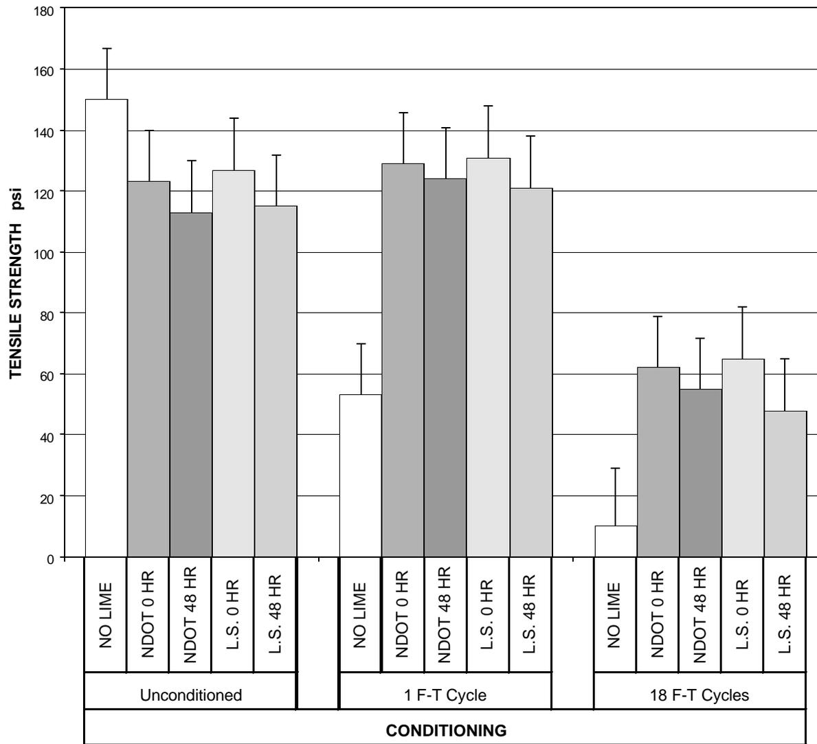
Figure 21. Average tensile strength property of the Lone Mountain AC-30 mixtures, vertical bars indicate the range of average value plus one least significant difference.
