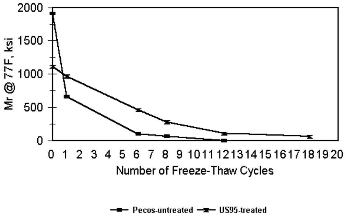
Figure 1. Mr property of field cores at various freeze-thaw cycles for the Pecos road and US 95 projects.
