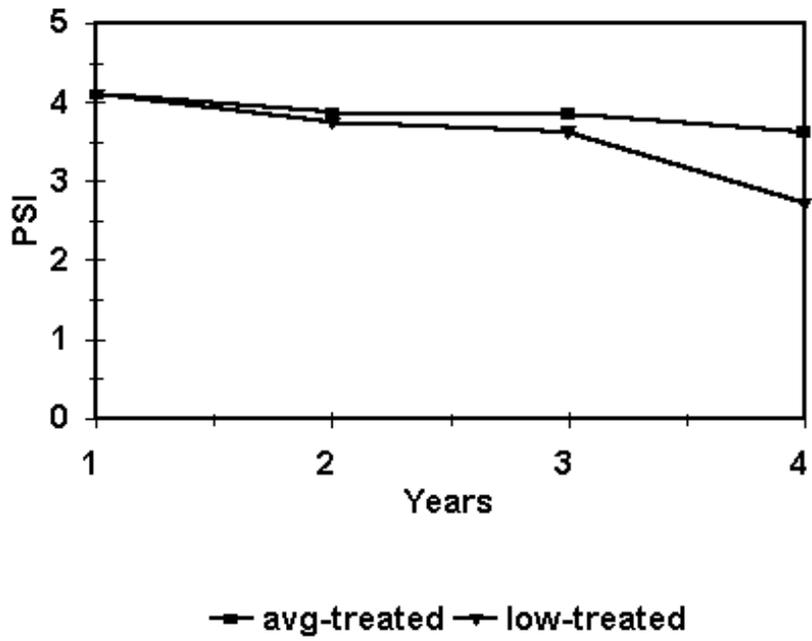
Figure 7. Average and low values of PSI for untreated and lime-treated mixtures on US 95 in southern Nevada.
