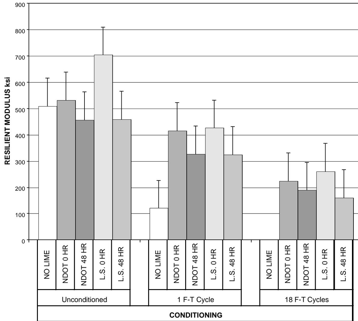
Figure 23. Average resilient modulus property of the Lone Mountain AC-30 mixtures, vertical bars indicate the range of average value plus one least significant difference.
