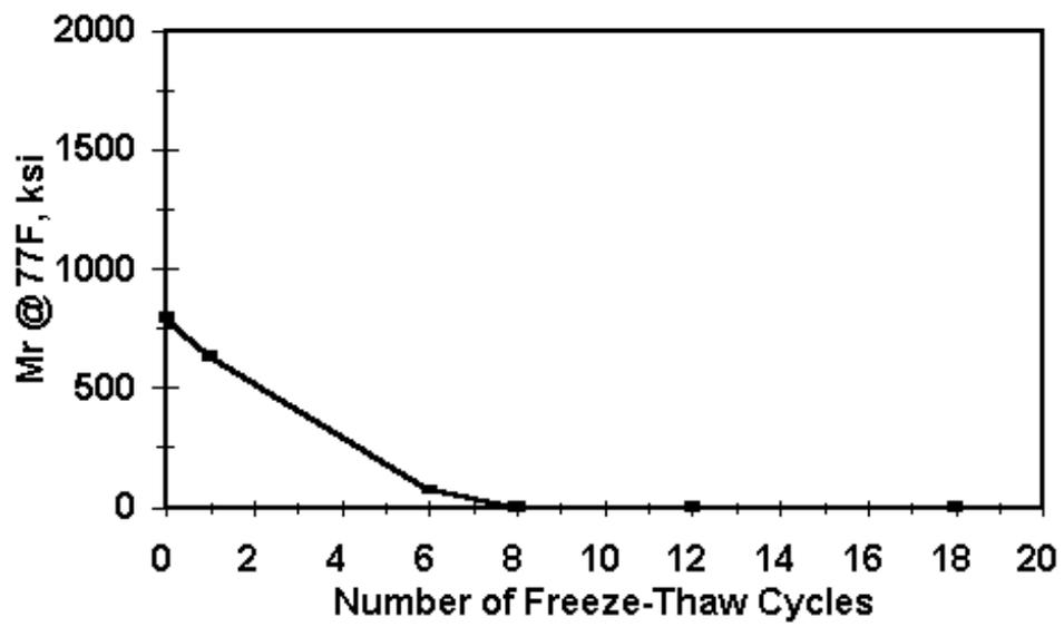
Figure 5. Mr property of field cores at various freeze-thaw cycles for the Lakeside Drive project.
