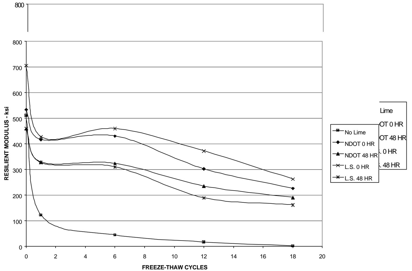
Figure 26. Resilient modulus property of the Lockwood PG 64-34 mixtures at various freeze-thaw cycles.
