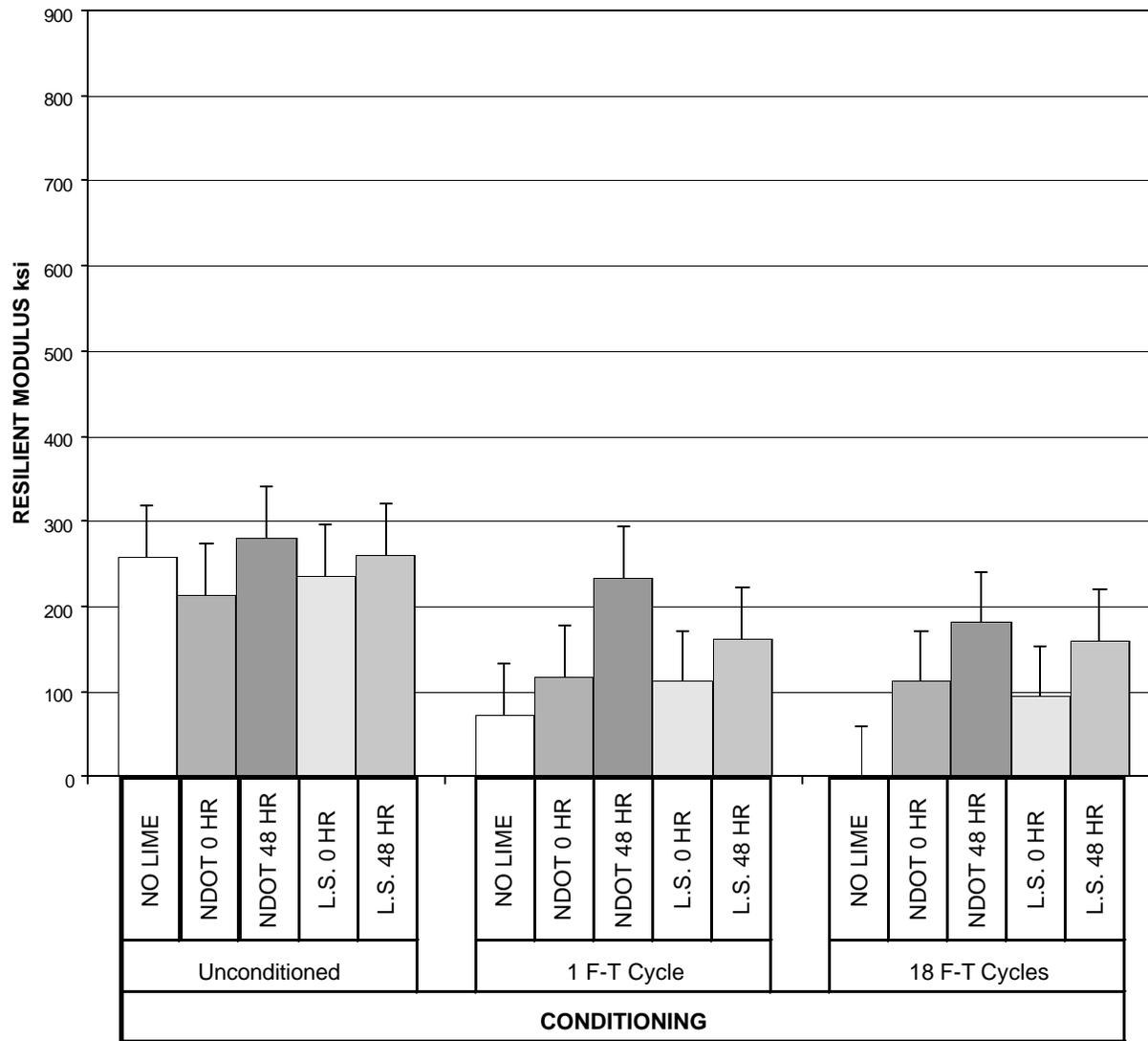
Figure 15. Average resilient modulus property of the Lockwood AC-20P mixtures, vertical bars indicate the range of average value plus one least significant difference.
