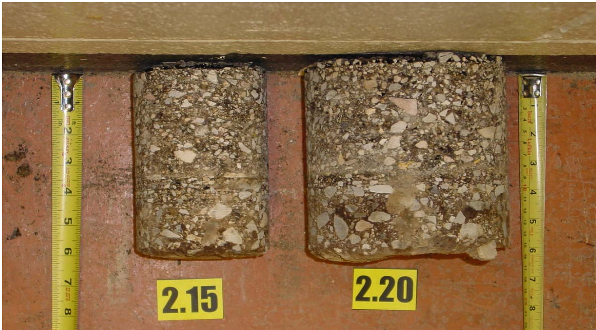
2 Months after Construction: Cores in Good Condition Pavement Condition: Good Condition
