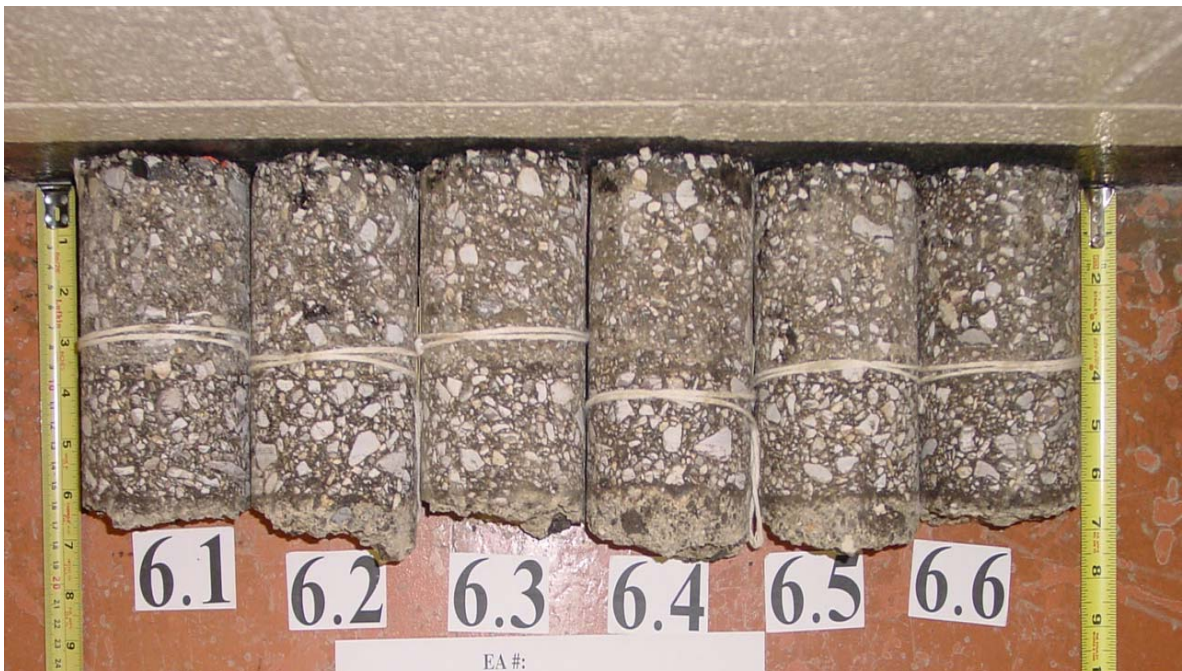
(b) 2 Years after Construction: Cores in Good Condition Pavement Condition: Good Condition
