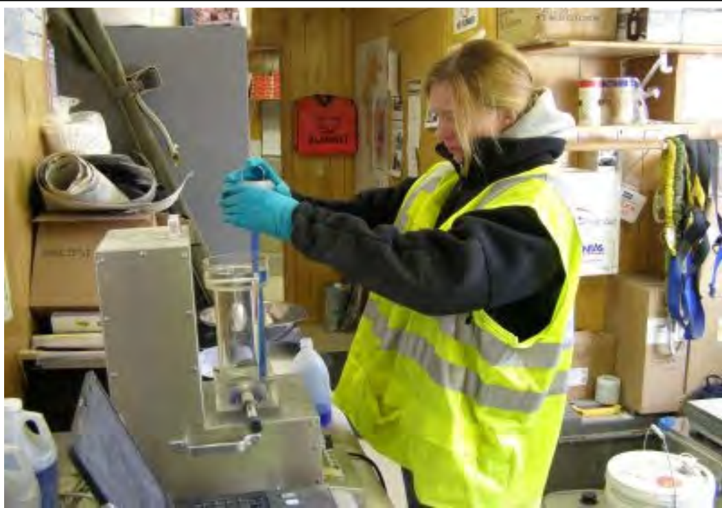
Figure 6.12: Air void analysis test set up
