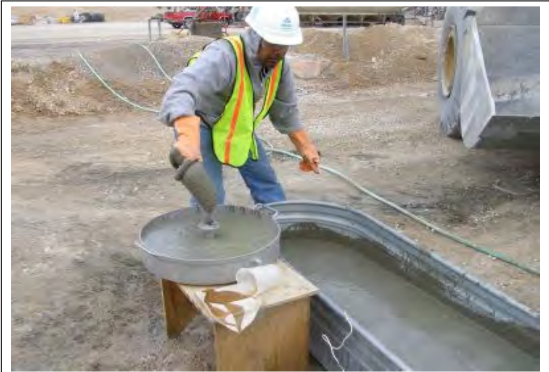
Figure 6.22: Rheology test sampling for pumped SCC
