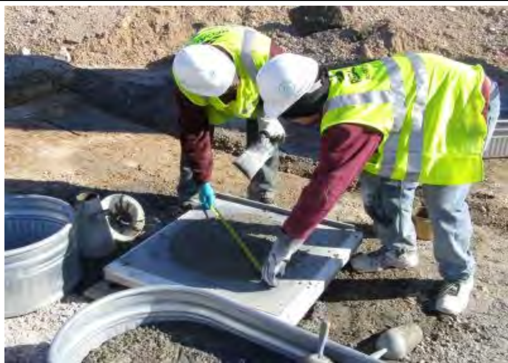
Figure 6.8c: Slump flow test (continued)
