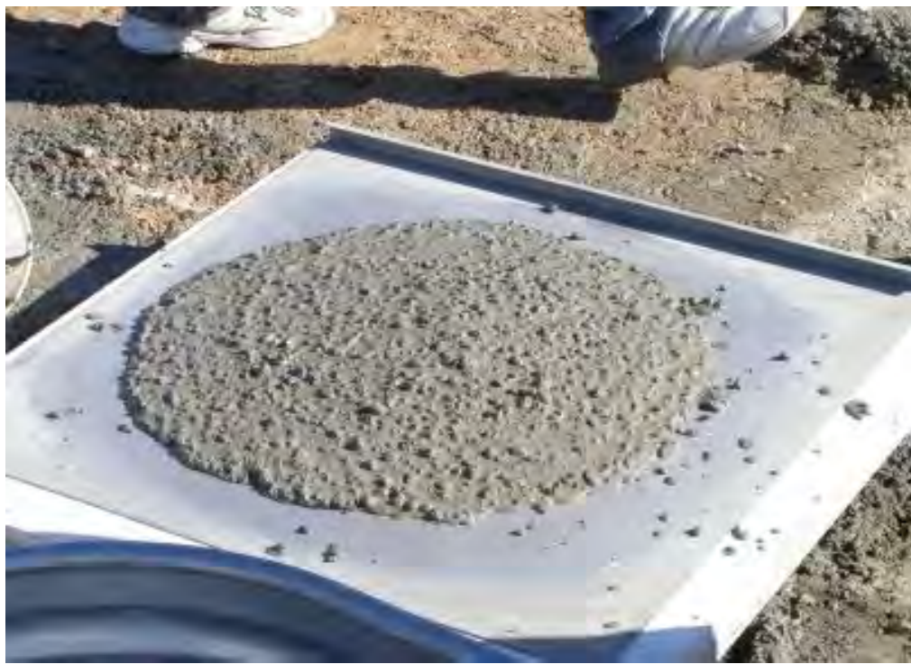
Figure 6.8b: Slump flow test (continued)
