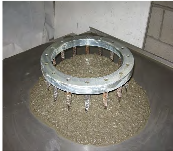
a) Slump flow (unconfined workability) and Visual stability index (VSI, dynamic segregation resistance), and b) J-ring (passing ability) tests
