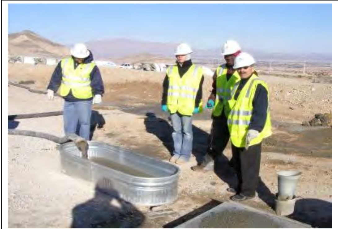
Figure 6.17: Pumping test - post-pumping SCC sample collection
