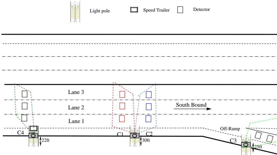
**Figure 5.9 Automatic Work Zone Information System and the Setting for Evaluation**
