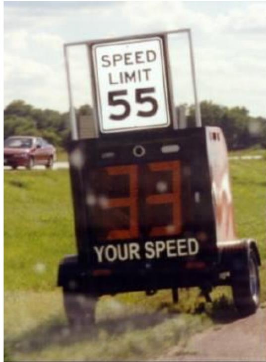
**Figure 1.1 An Example of a Speed Monitoring Display**
