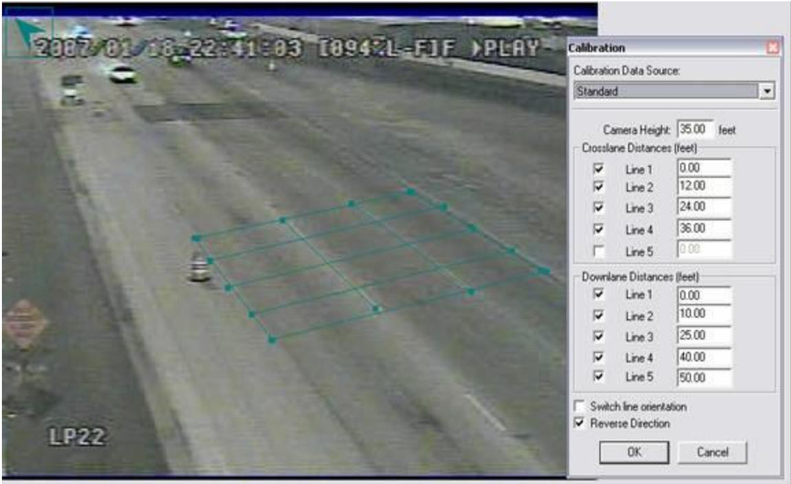
Figure 4.3 Calibration of Autoscope
