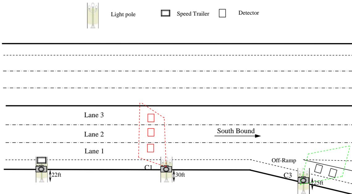
**Figure 5.8 Simplified Automatic Work Zone Information System for Testing on I-515**
