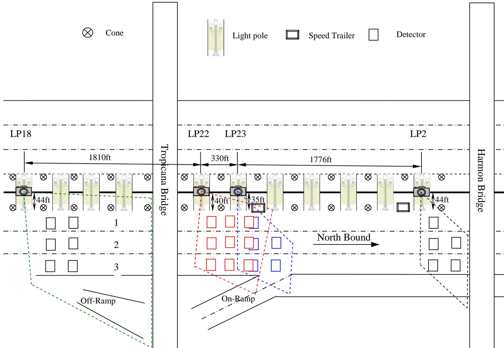
**Figure 4.1 Camera Layout on the Test Site**
