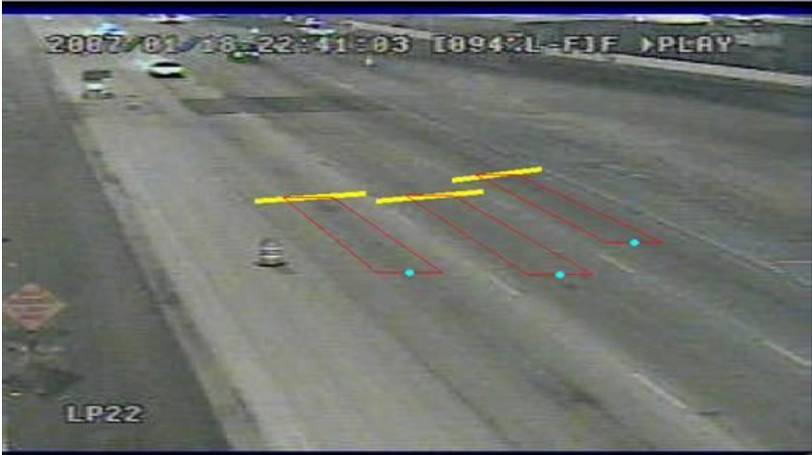
Figure 4.5 Speed Detector
