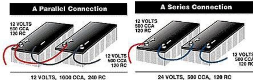
**Figure B3 Two 12V Deep-Cycle Batteries Connected in Parallel or in Series to Provide Sufficient Operation Voltage and Current**
