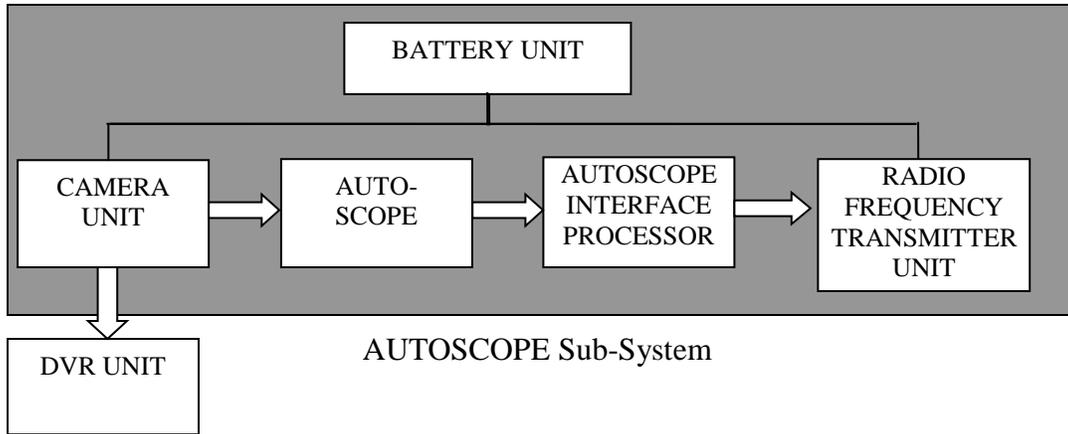
**Figure B7 Autoscope Sub-System Block Diagram**
