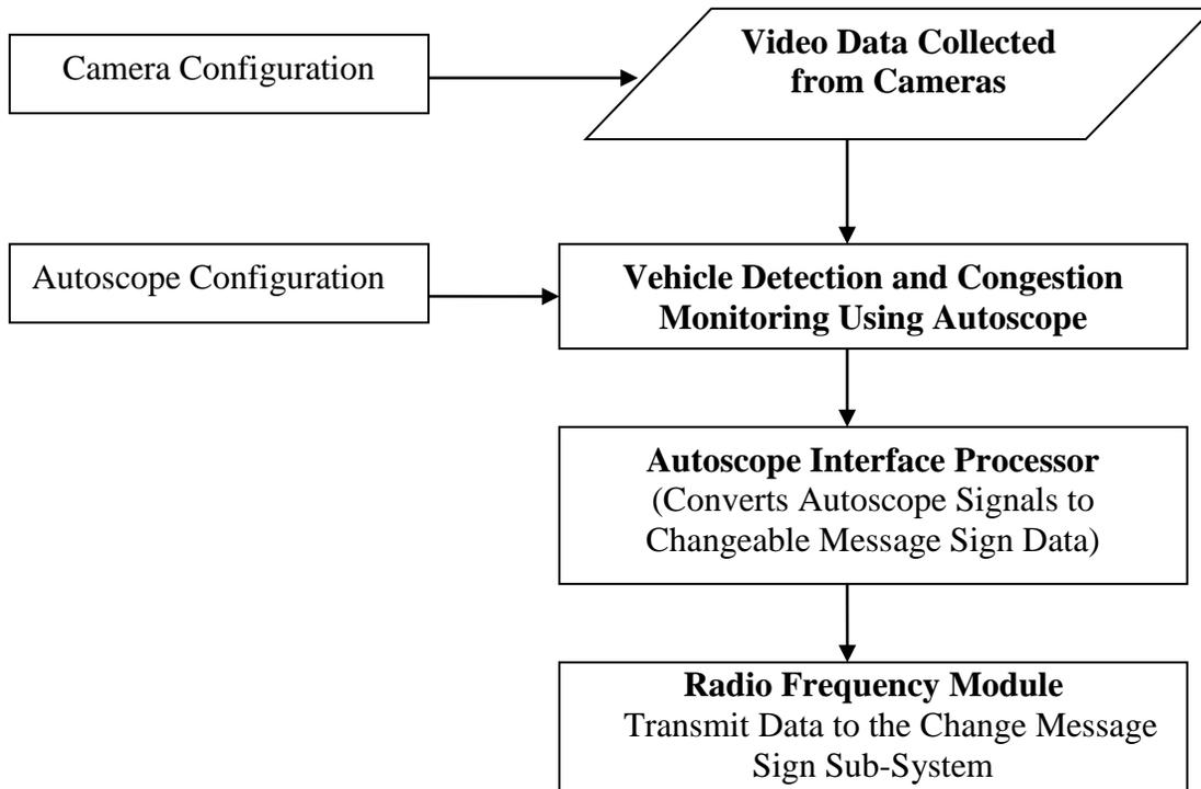
**Figure B8 Autoscope Sub-System Operation Flow**
