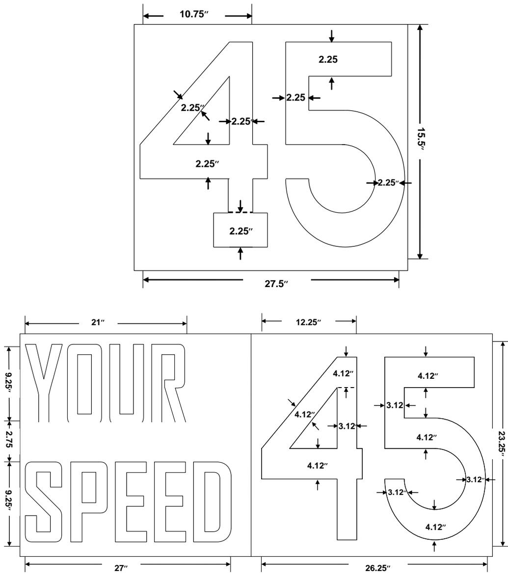
**Figure 3.4 Size Measurements for the Small Sign (above) and Big Signs (below)**
