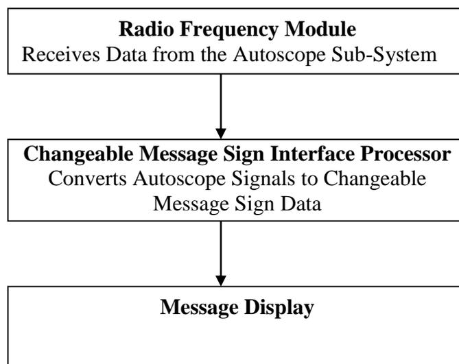
**Figure B10 Changeable Message Sign Sub-System Operation Flow**
