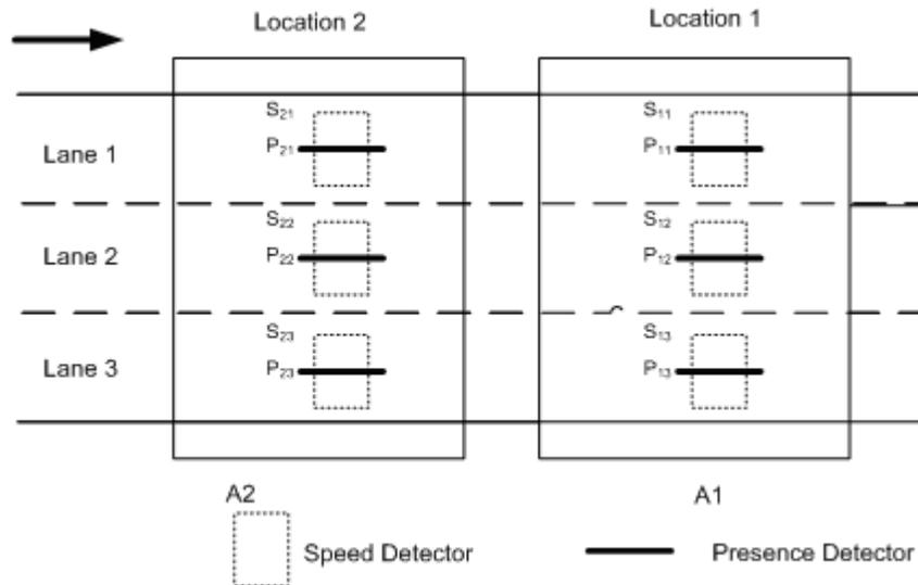
**Figure B11 Presence and Speed Detectors within the Coverage of the Autoscope, a Vision Detection Product**
