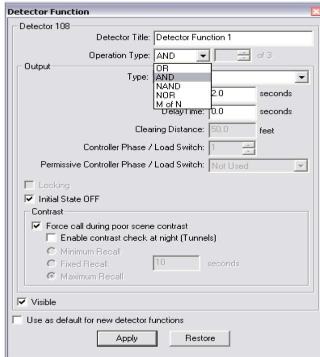
**Figure A4 Boolean Detector Function Configuration**
