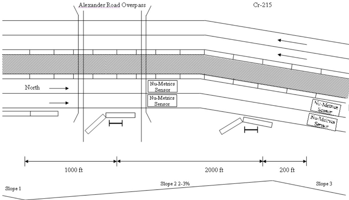
**Figure 3.6 Layout of Speed Trailer and Detectors on the Test Site on Cr-215**
