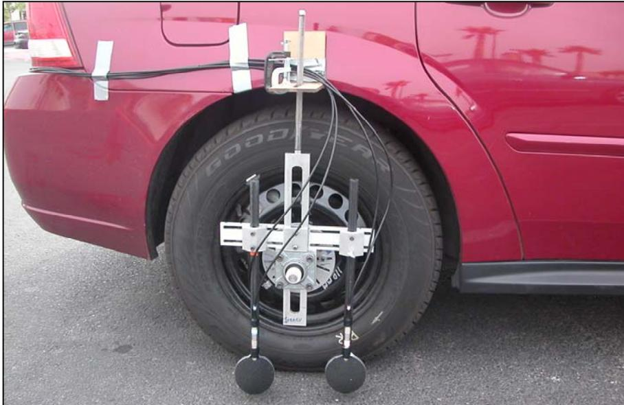
**Figure 1: OBSI Equipment Installed on the Malibu Test Vehicle**
