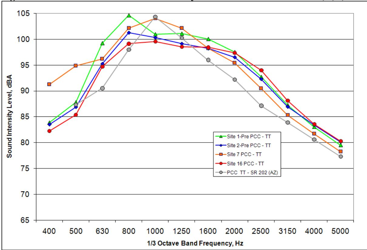
**Figure 13: 1/3 Octave band levels for Randomly Transverse Tined PCC Sites 8 and 17b**
