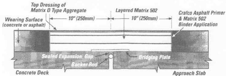
Figure 1. Typical Matrix 502 Asphaltic Plug Bridge Joint System
