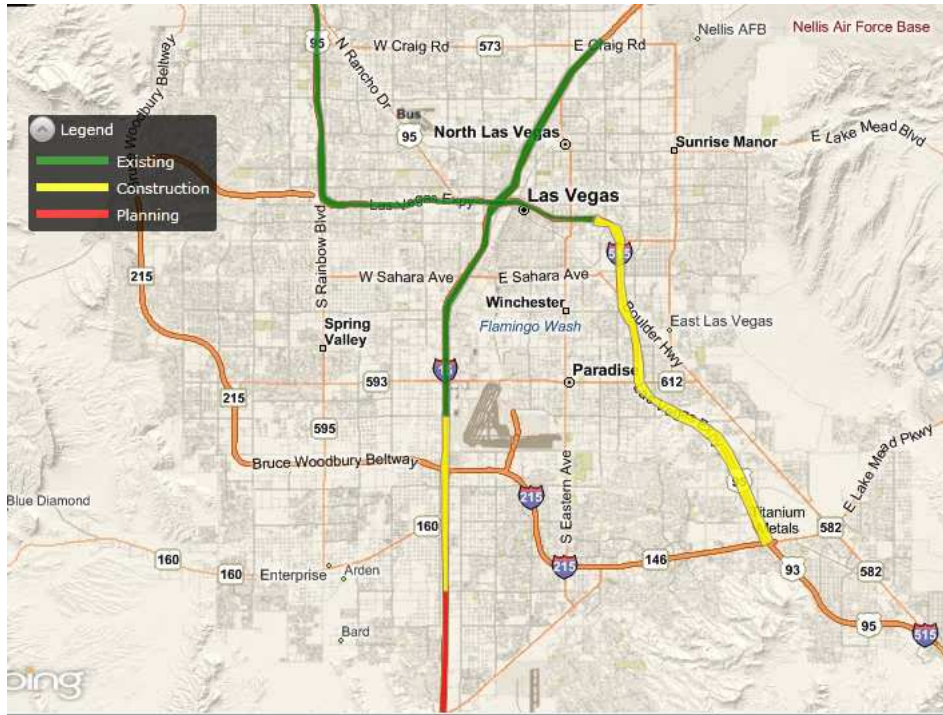
Figure 4.1: FAST Intelligent Transportation System (ITS) Coverage. Green= Existing ITS, Yellow= under construction ITS, and Red= under planning ITS.
