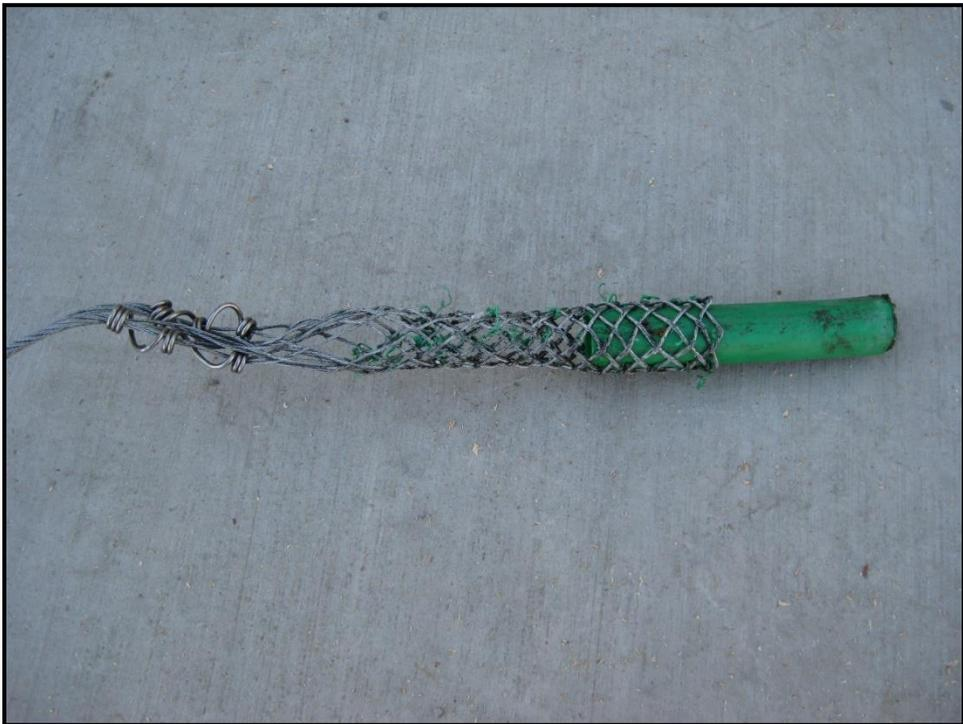
**Figure 2-16: Cable Gripper**
