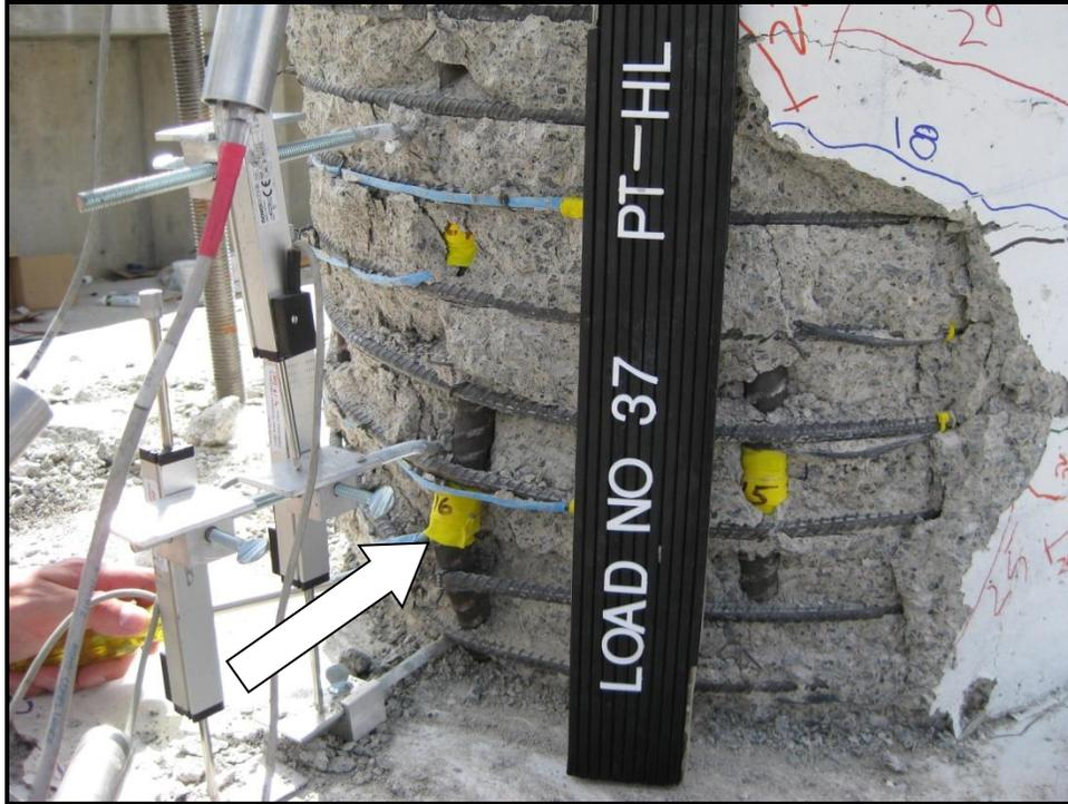
**Figure 4-41: PT-HL, First Transverse Reinforcing Bar Fracture**
