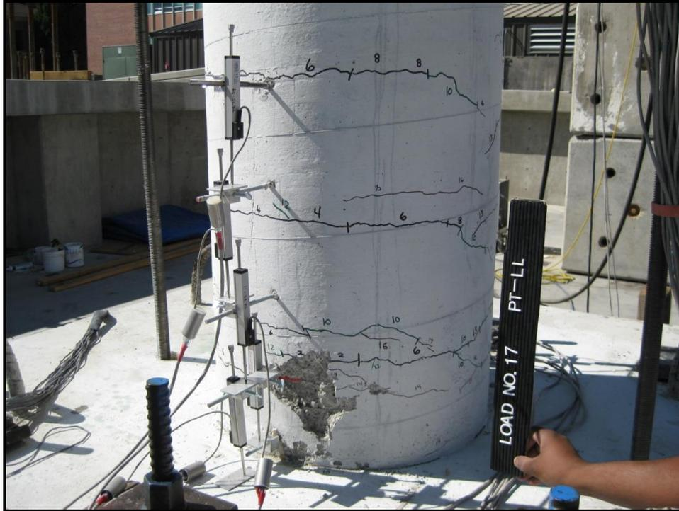
**Figure 4-3: PT-LL Initial Spalling on East, Visible Spiral**
