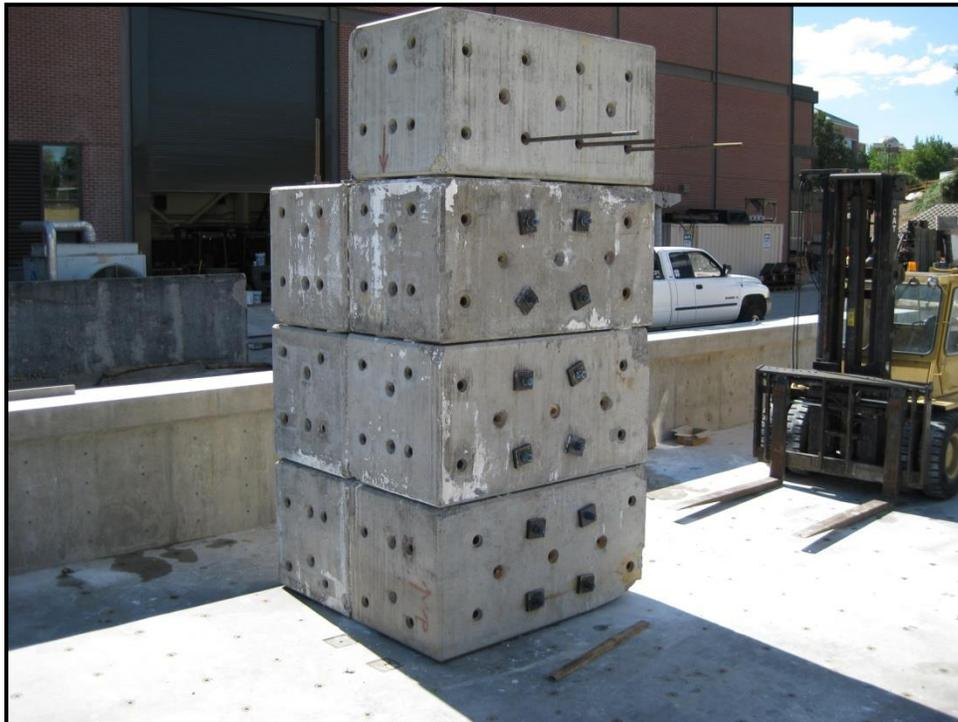
**Figure 3-7: Reaction Wall**
