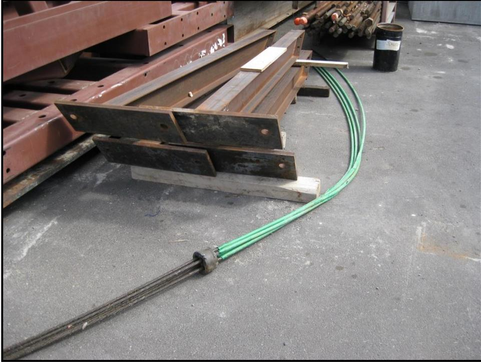
**Figure 4-73: Removed Tendon**
