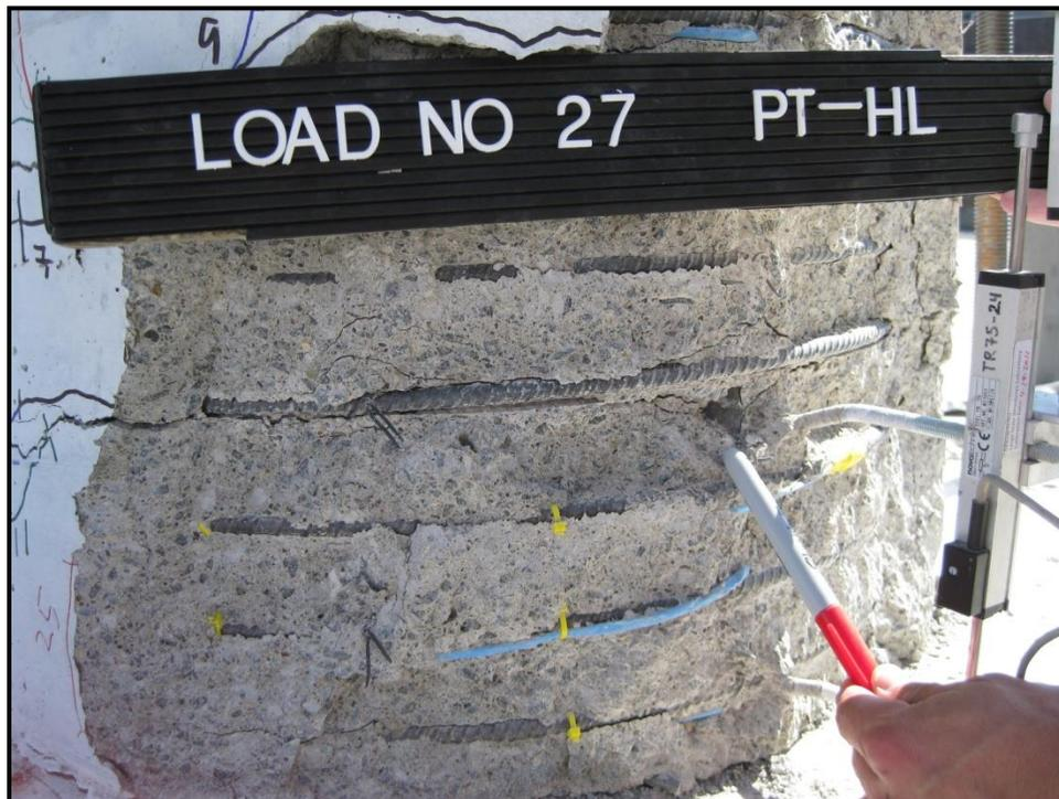
**Figure 4-38: PT-HL, Visible Longitudinal Reinforcement, West Side**
