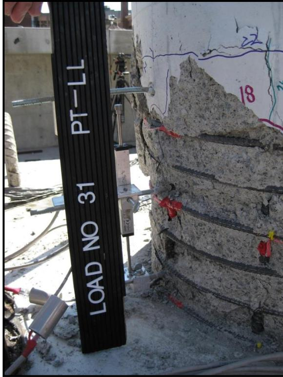
**Figure 4-5: PT-LL Buckling Longitudinal Reinforcing Bar, East**
