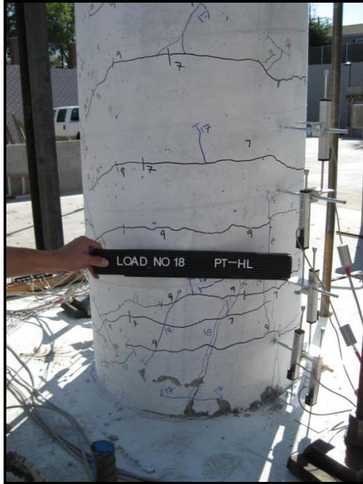
**Figure 4-35: PT-HL, First Spalling, West Side**
