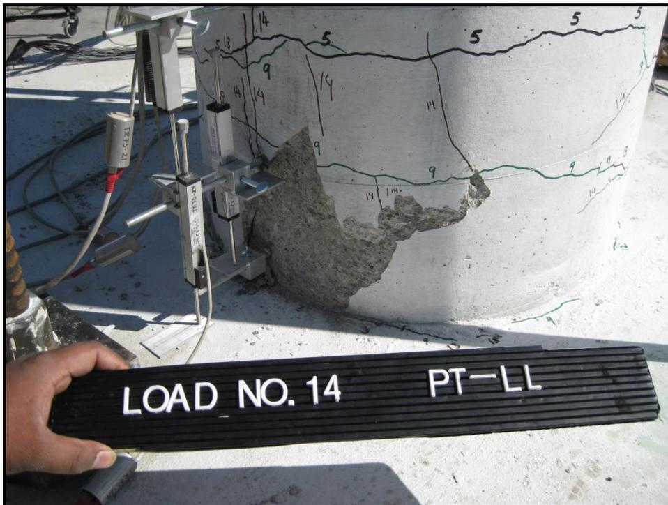
**Figure 4-2: PT-LL Initial Spalling on West**
