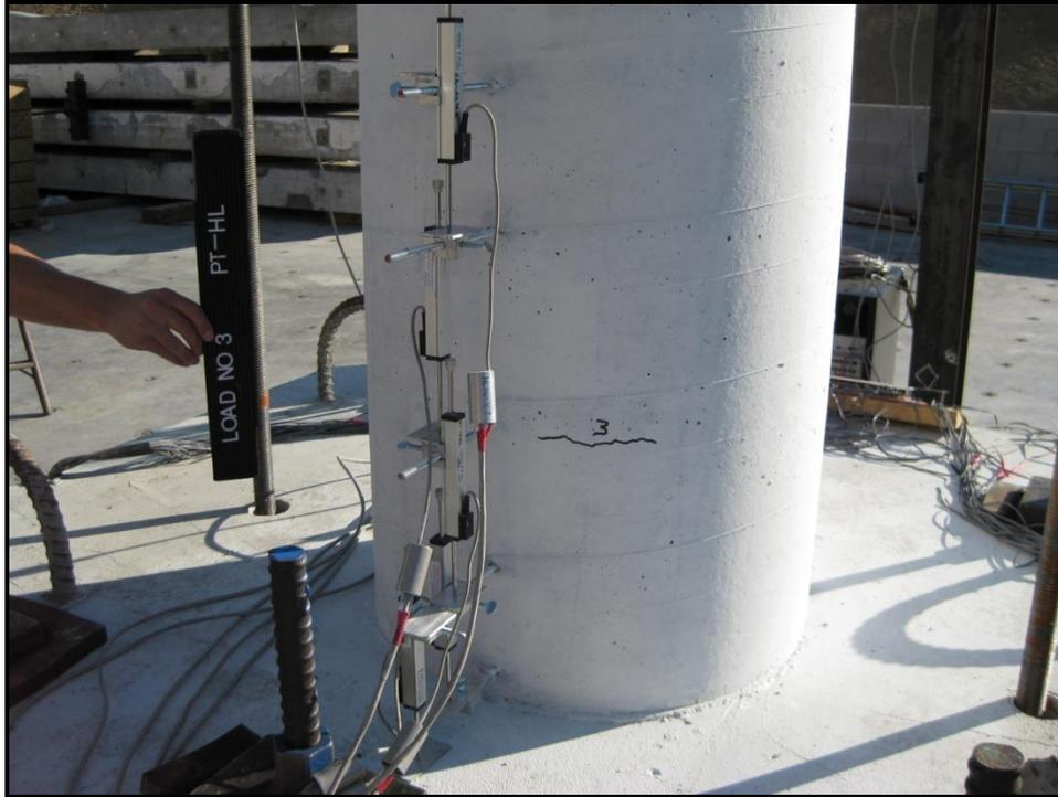
**Figure 4-33: PT-HL, First Crack**
