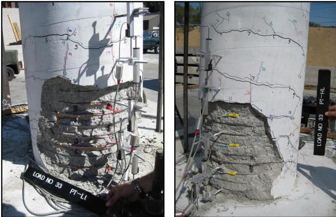
**Figure 4-72: 7% Drift Damage Comparison**
