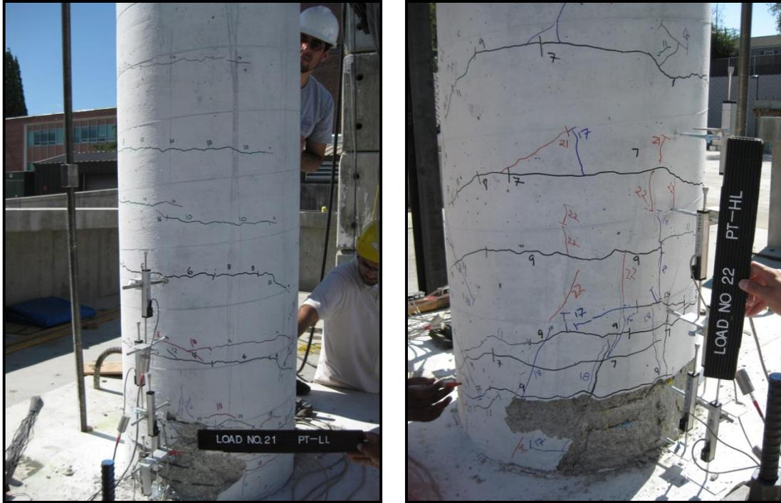
**Figure 4-69: 4% Drift Damage Comparison**
