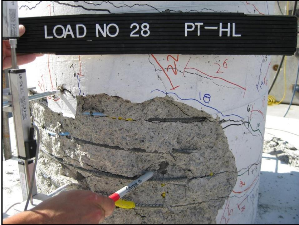
**Figure 4-39: PT-HL, Visible Longitudinal Reinforcement, East Side**
