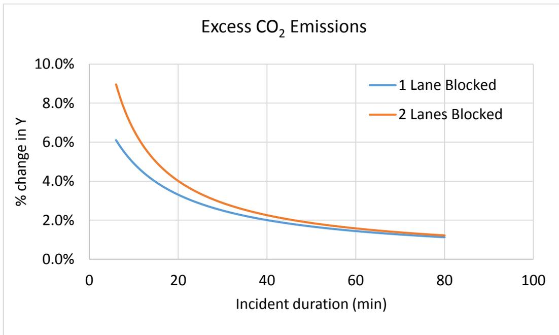
Figure 7-6. Percent Change in Excess CO<sub>2</sub> Emissions for unit change in Lane-Minutes of Blockage
