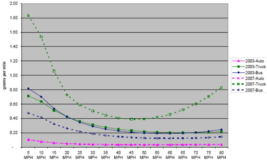
Figure 3-4. PM<sub>10</sub> Emissions versus Speed
