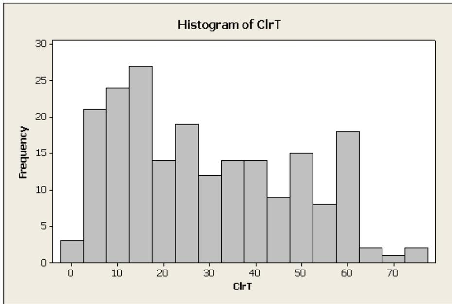
Figure 5-1. Histogram of Incident Clearance Durations (minutes)
