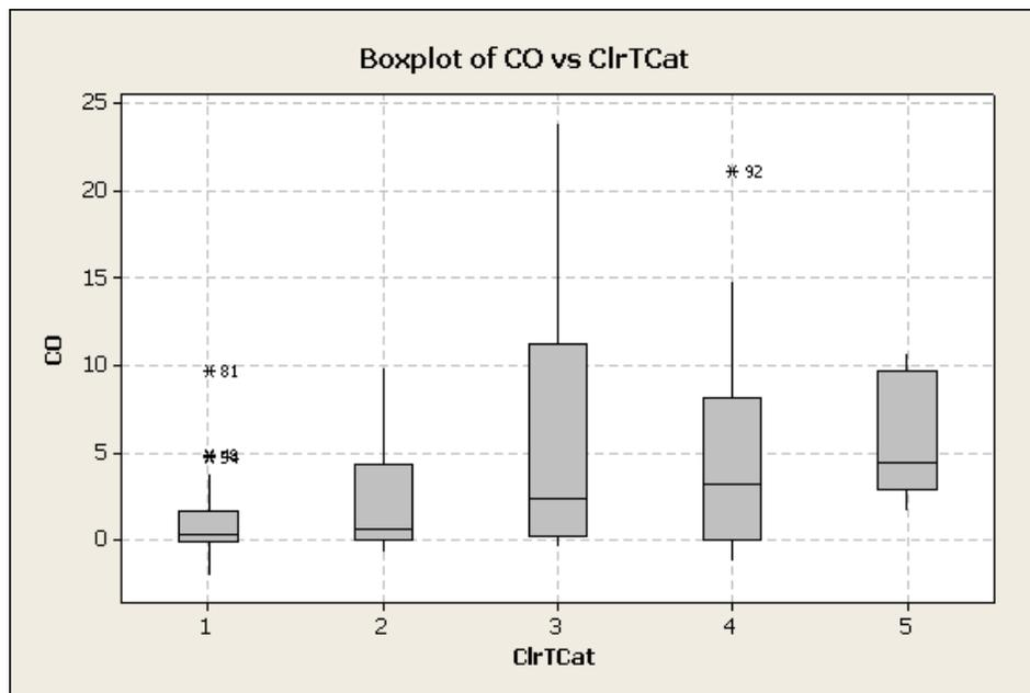
Figure 5-21. Box-plot: Excess CO emissions (in Kgs) vs. Incident Duration
