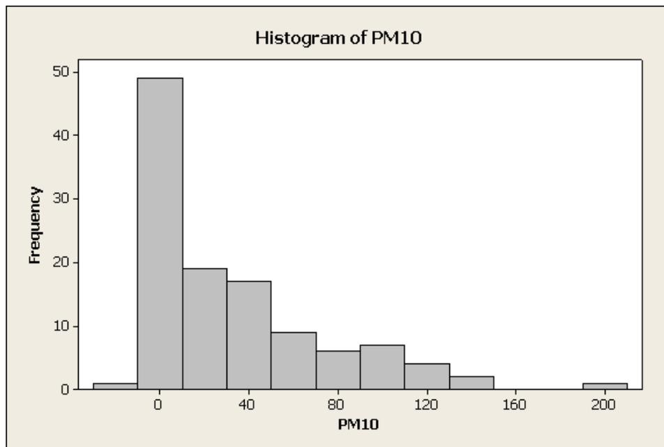
Figure 5-25. Histogram: Excess PM<sub>10</sub> Emissions in grams
