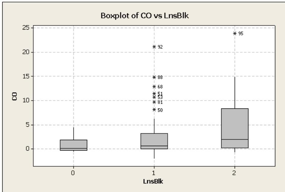
Figure 5-20. Box-plot: Excess CO emissions (in Kgs) vs. Number of Blocked lanes
