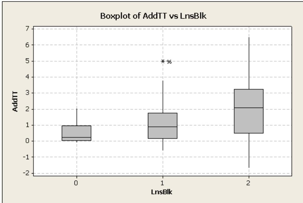
Figure 5-4. Box-plot: Primary Additional Travel Time (in minutes) Vs. Number of Blocked Lanes
