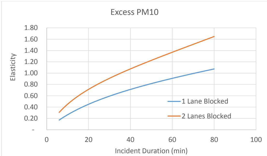
Figure 7-11. Elasticity for Excess PM10 emissions with respect to Incident Duration
