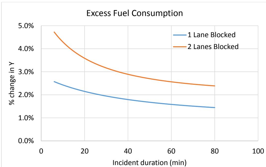
Figure 7-4. Percent Change in Excess Fuel Consumption for unit change in Lane-Minutes of Blockage
