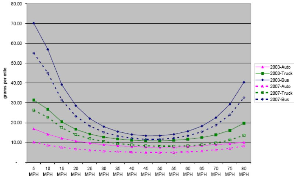
Figure 3-2. CO Emissions versus Speed
