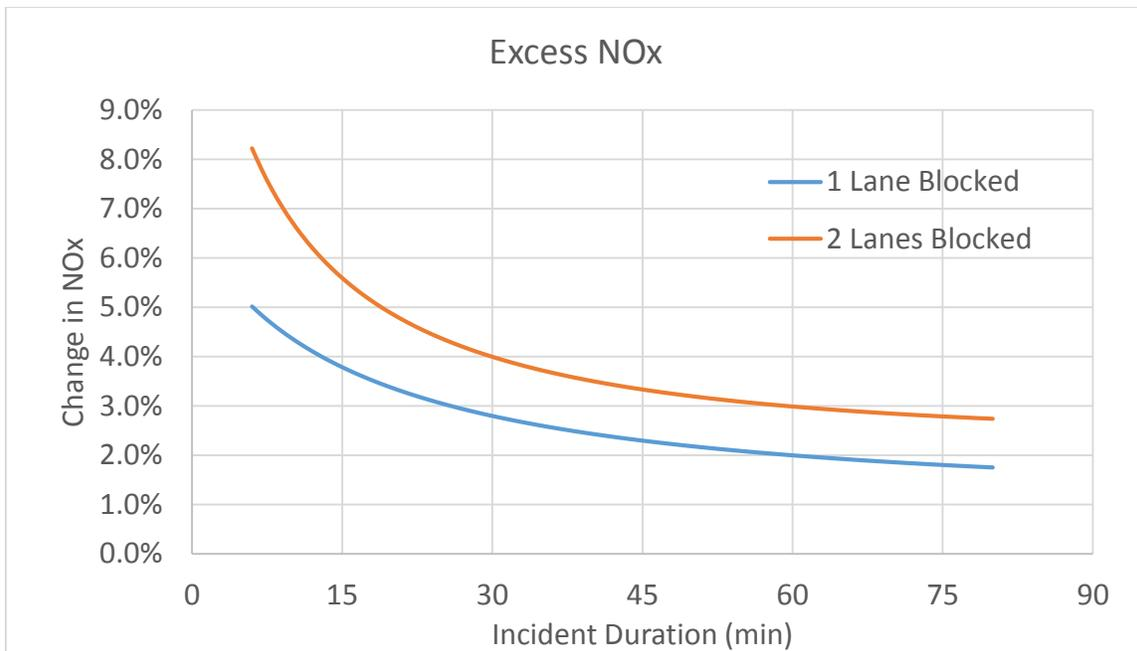
Figure 7-10. Percent Change in Excess NO<sub>x</sub> Emissions for 1 minute change in incident duration
