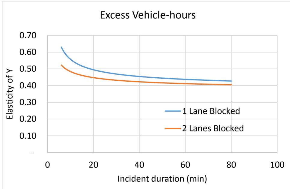
Figure 7-1. Elasticity of Excess VHT as a function of Incident Duration
