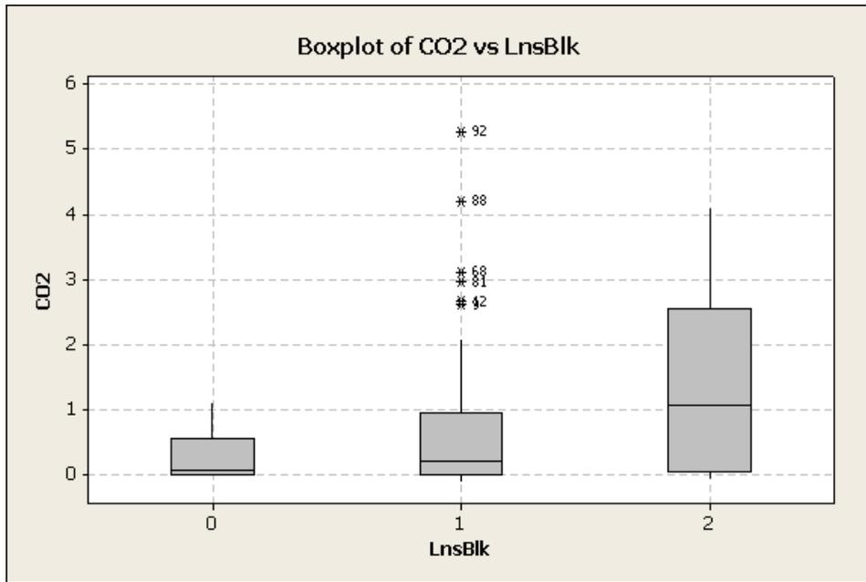
Figure 5-17. Box-plot: Excess CO<sub>2</sub> emissions (in Tons) vs. Number of Blocked lanes
