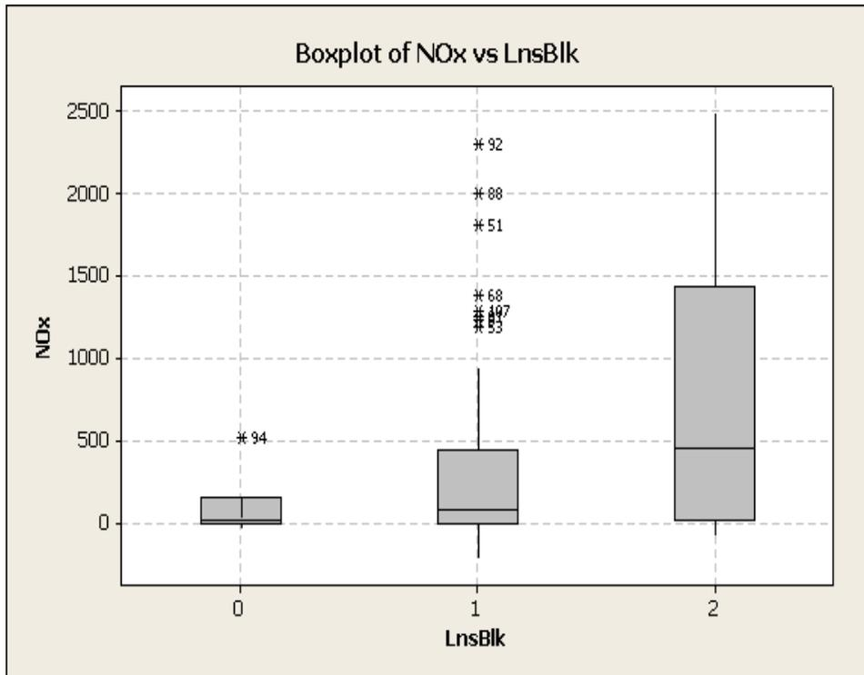
Figure 5-23. Box-plot: Excess NO<sub>x</sub> emissions (in Grams) vs. Number of Blocked lanes
