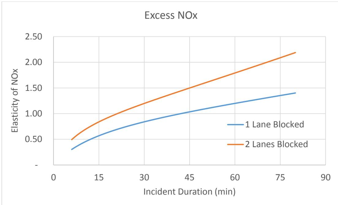
Figure 7-9. Elasticity of Excess NO<sub>x</sub> Emissions with respect to incident duration
