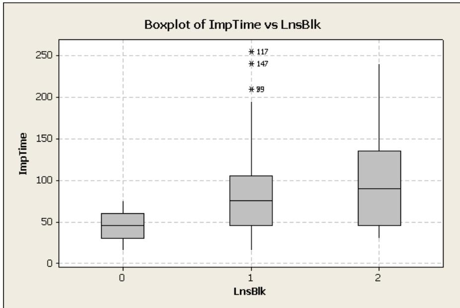
Figure 5-9. Box-plot: Temporal Impact (in minutes) Vs. Number of Blocked Lanes
