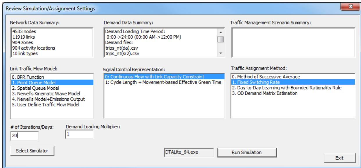
Figure 15. Model Selection for Running Traffic Assignment
