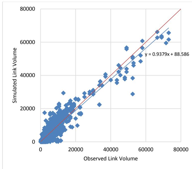
Figure 23. Plot of Simulated and Observed Link Volume (Prior to ODME)
