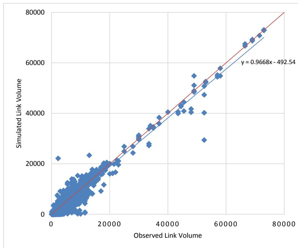
Figure 24. Plot of Simulated and Observed Link Volume (after ODME)
