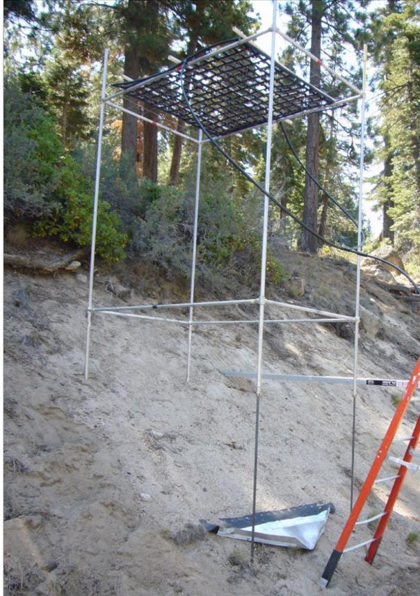
Figure 3.2. Typical rainfall simulator setup
