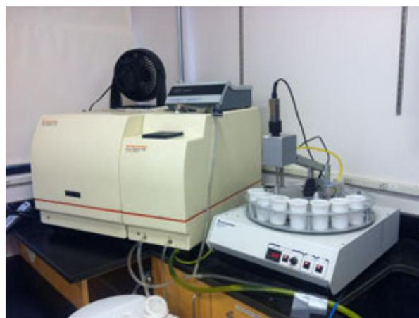
Figure 3.8. Laser particle size analyzer (DRI)
