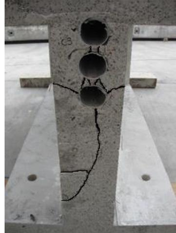
b) Cross section with cracks drawn.
