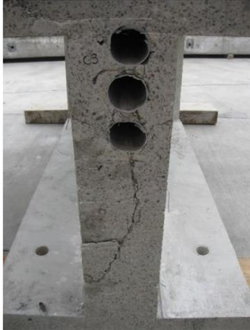
a) Cross section with cracks.
