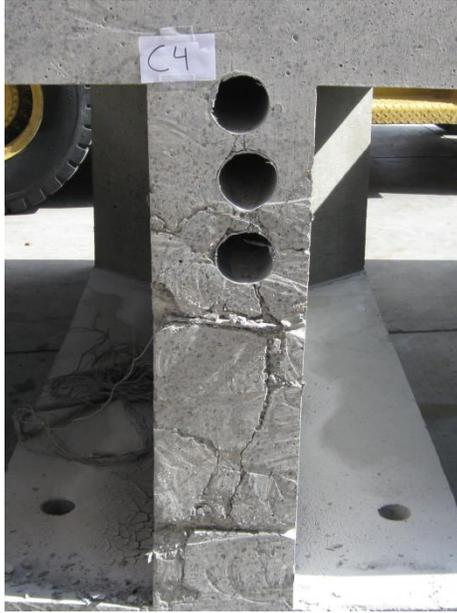
a) Cross section with cracks.
