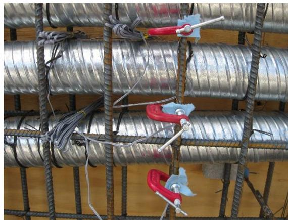
**Figure 2-25: Shear reinforcement strain gauges installed on beam.**
