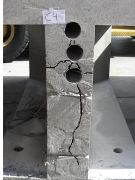
b) Cross section with cracks drawn.
