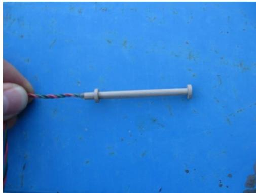
**Figure 2-27: Embedded concrete strain gauge.**
