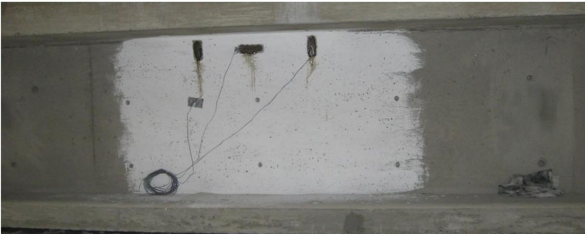
**Figure 3-5: C1 web face after completion of all loading with no cracks.**
