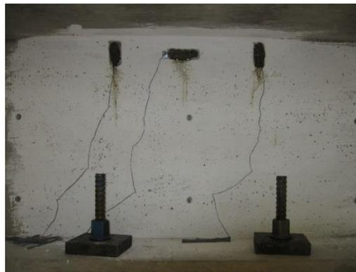
**Figure 2-33: Concrete surface strain gauges installed on web face.**
