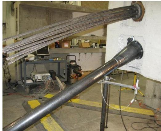
**a) Air pressure/grout caps. b) Steel trumpet used for air pressure testing.**
