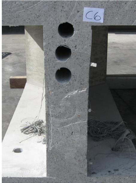
**Figure 3-69: C6 cut beam cross section with no cracks.**
