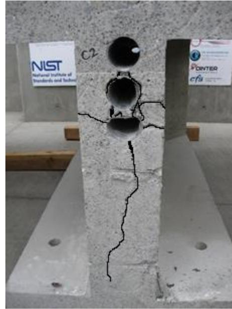
b) Cross section with cracks drawn.
