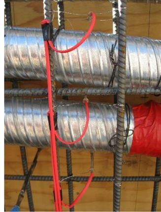
a) Strain gauges tied to shear reinforcement.      b) Strain gauges around ducts.
