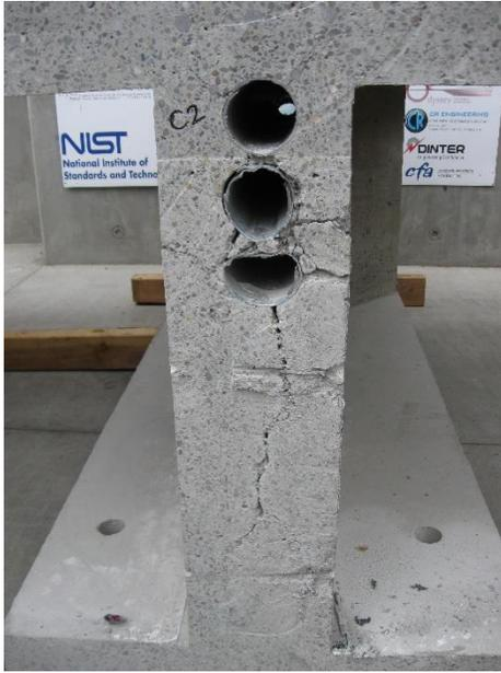
a) Cross section with cracks.
