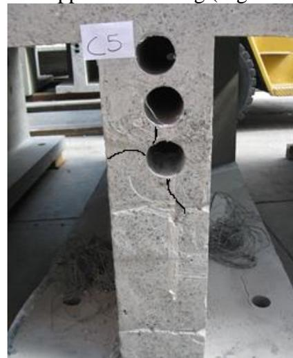
**b) Cross section with cracks drawn.**
