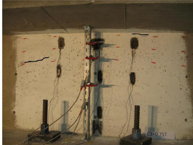
**Figure 3-25: C3 crack appearance at 0.75fpuB.**
