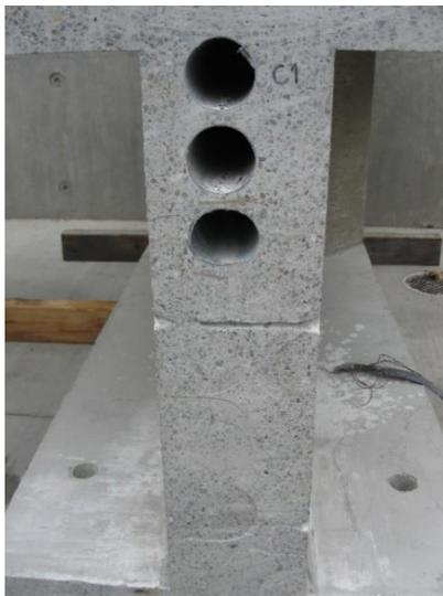
a) Cross section with minimal cracks.
