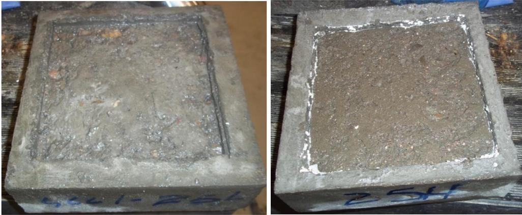
**Figure 6.9 (Left) 0.75-25-L and (right) 0.75-25-H specimens after 15 freezing and thawing cycles.**
