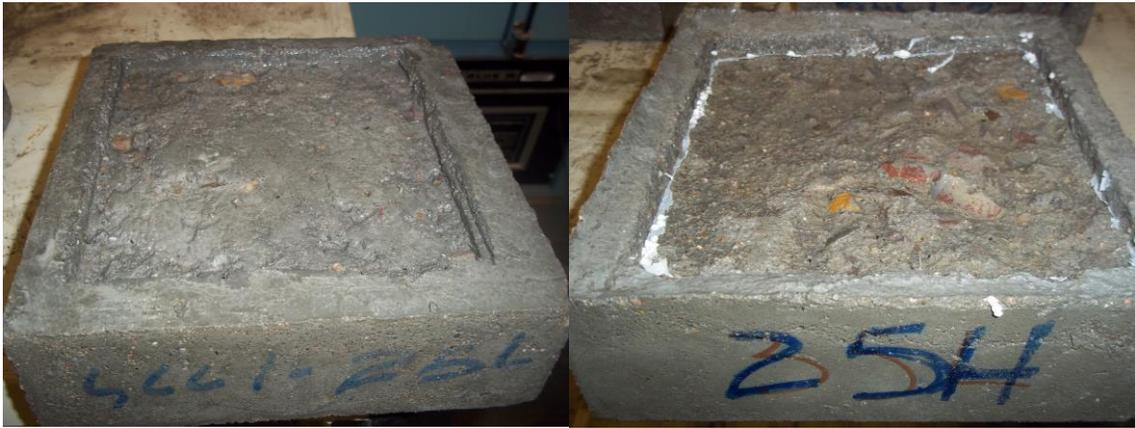
**Figure 6.13 (Left) 0.75-25-L and (right) 0.75-25-H after 30 freezing and thawing cycles.**
