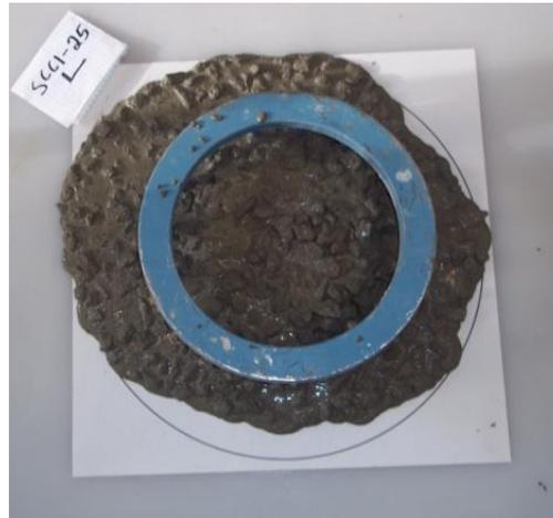
**Figure 4.2 J-ring flow diameter for low-slump SCC with 25% fly-ash replacement (0.75-25-L).**
