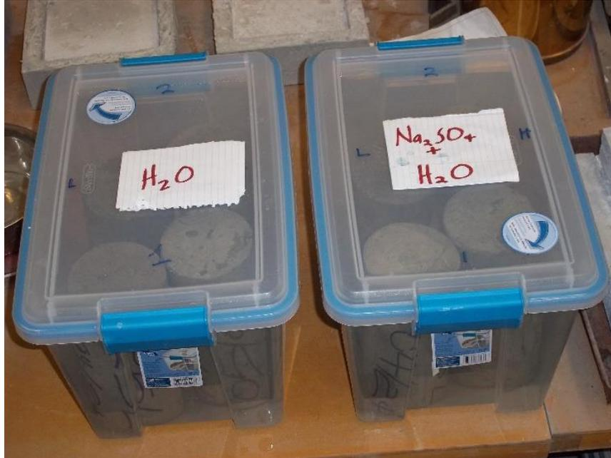
**Figure 4.13** Experimental setup for the sulfate attack test.
