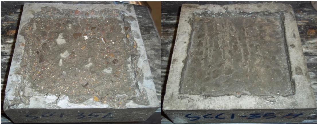
**Figure 6.10 (Left) 0.75-35-L and (right) 0.75-35-H after 15 freezing and thawing cycles.**
