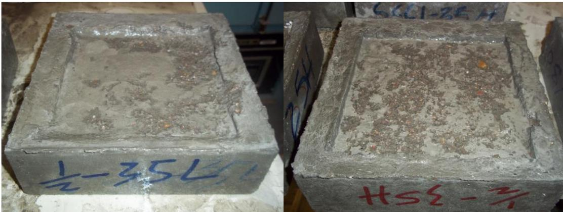
**Figure 6.18 0.5-35-L (Left) and 0.5-35-H (right) after 10 freezing and thawing cycles.**
