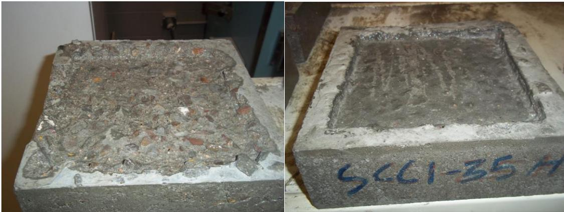
**Figure 6.14 (Left) 0.75-35-L and (right) 0.75-35-H after 30 freezing and thawing cycles.**
