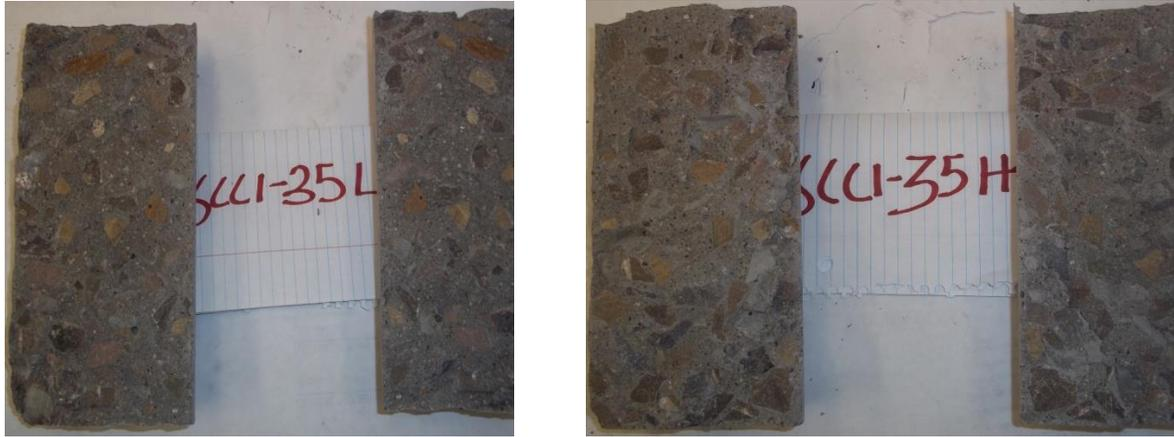
**Figure 4.8 Coarse aggregate distribution for hardened 0.75-35.**
