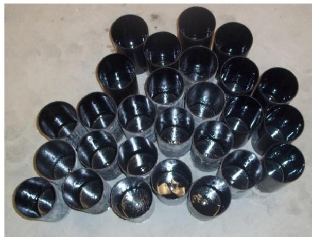
**Figure 4.4** Lubricated cylindrical molds for specimen fabrication.
