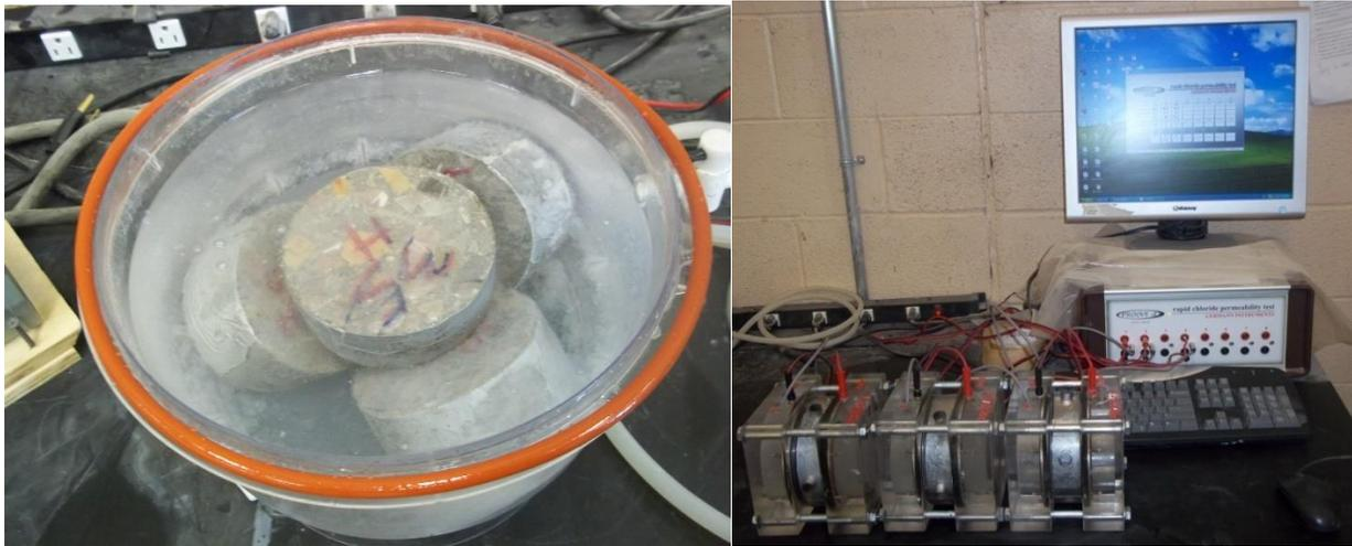
**Figure 4.12** Experimental setup for the rapid chloride penetration test (RCPT).
