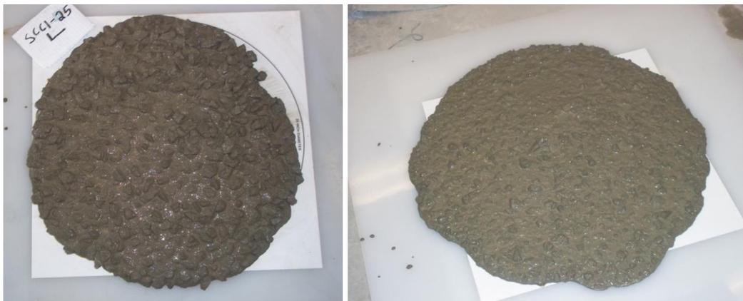
**Figure 4.1** Low and high diameters of slump flow for 0.75% coarse aggregate and 25% fly ash.
