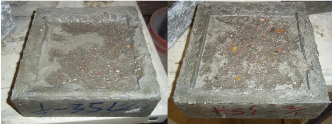
**Figure 6.20 (Left) 0.5-35-L and (right) 0.5-35-H after 20 freezing and thawing cycles.**
