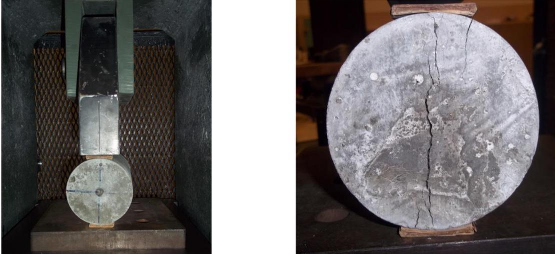
**Figure 4.6 Experimental setup for the Splitting Tensile Strength test.**
