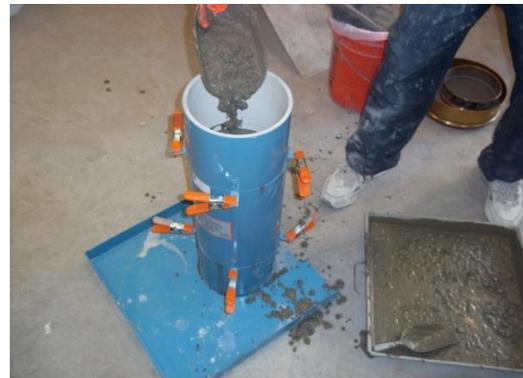
**Figure 4.3 Test setup for Static Column Segregation for 0.75-25-L.**
