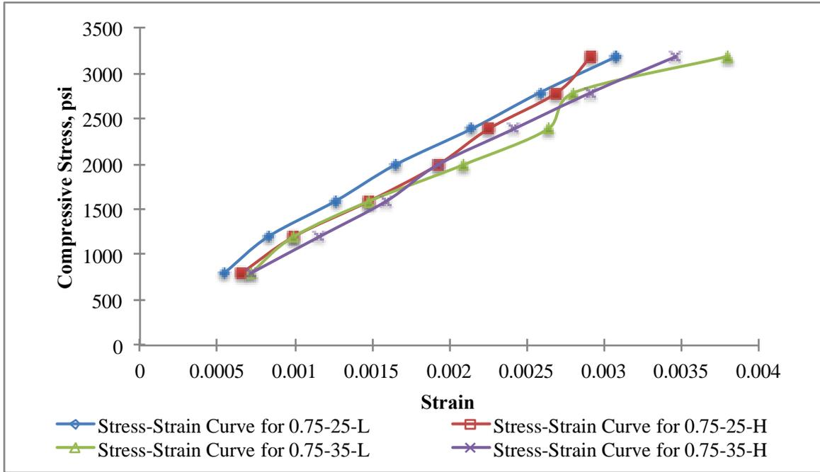
**Figure 6.4 Stress-strain curves for 0.5-in self-consolidating concrete mixture designs.**
