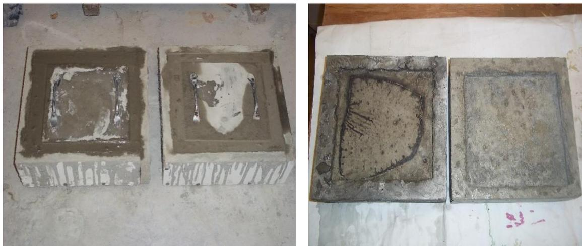
**Figure 4.14** Fabrication of specimens for the surface scaling test.
