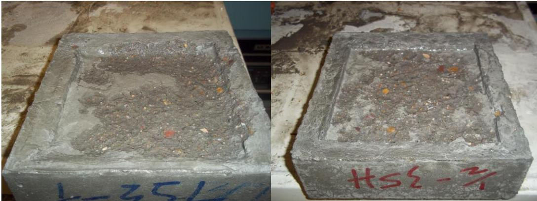
**Figure 6.22 (Left) 0.5-35-L and (right) 0.5-35-H after 30 freezing and thawing cycles.**
