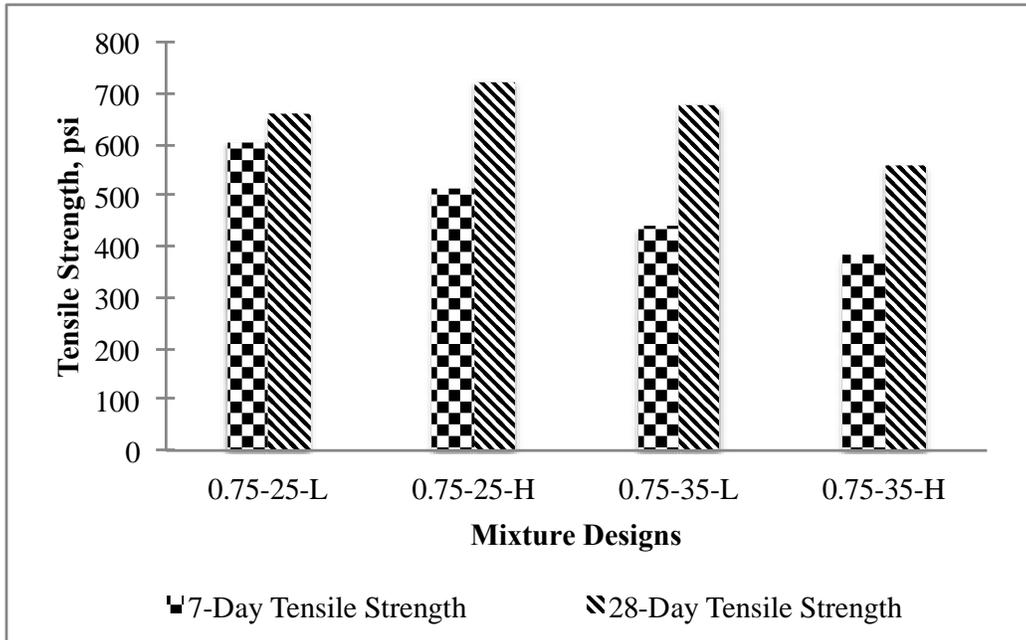
**Figure 6.2 Tensile strength for 0.5-in coarse aggregate SCC mixtures.**
