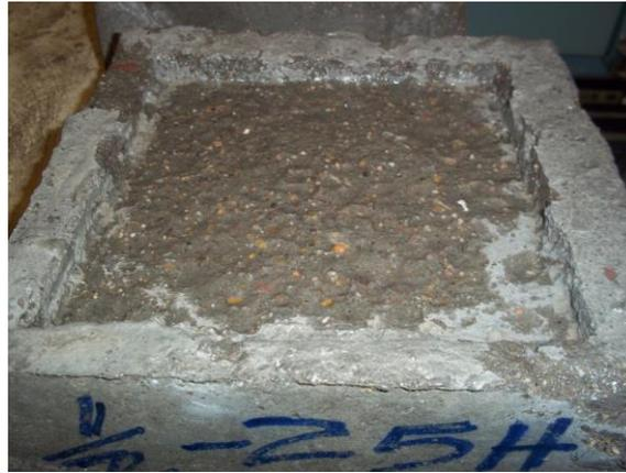
**Figure 6.19 0.5-25-H after 20 freezing and thawing cycles.**
