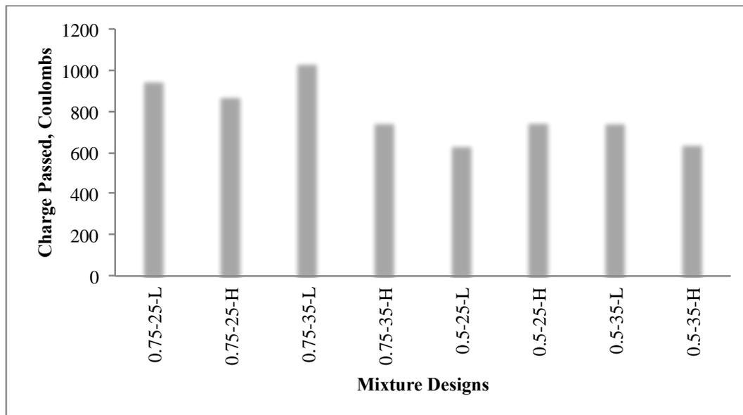
**Figure 6.5 Charge passed for self-consolidating concrete mixtures.**
