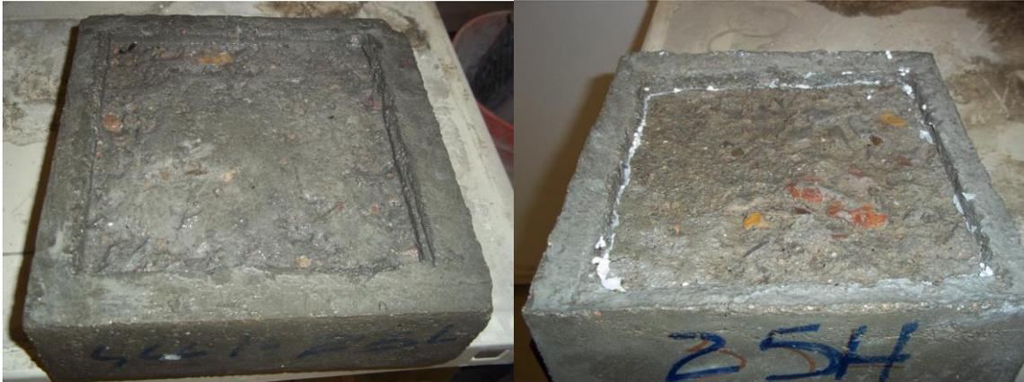
**Figure 6.11 (Left) 0.75-25-L and (right) 0.75-25-H after 20 freezing and thawing cycles.**
