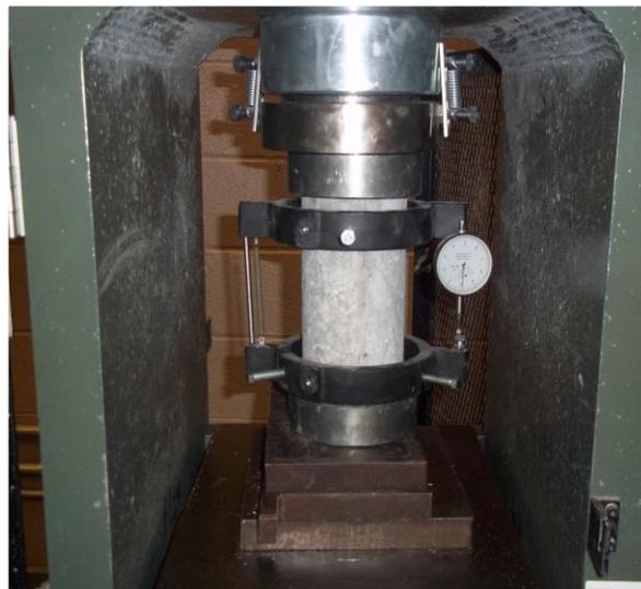
**Figure 4.11 Experimental setup for the Static Modulus of Elasticity test.**
