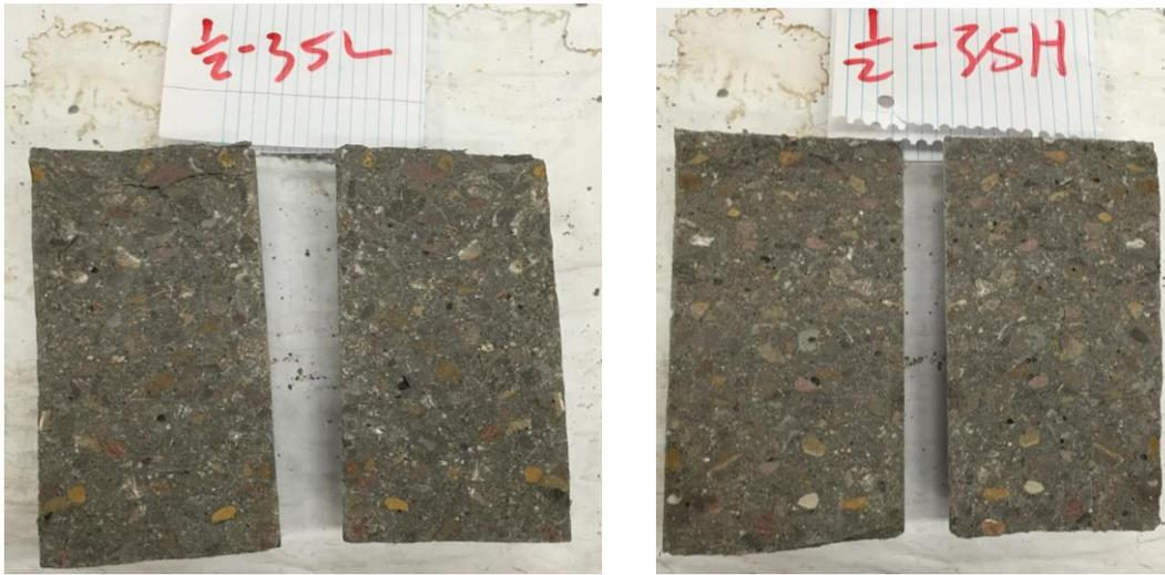
**Figure 4.10 Coarse aggregate distribution for hardened 05-35.**
