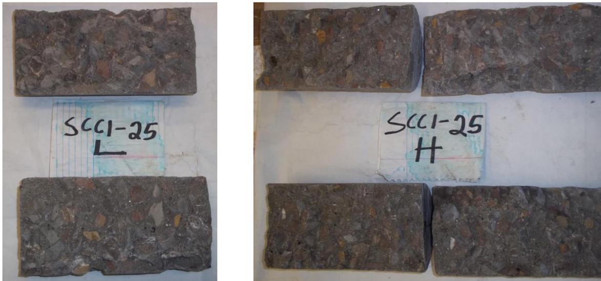
**Figure 4.7 Coarse aggregate distribution for hardened 0.75-25**
