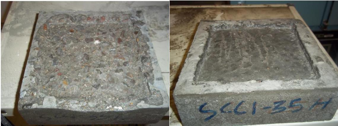
**Figure 6.12 (Left) 0.75-35-L and (right) 0.75-35-H after 20 freezing and thawing cycles.**
