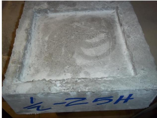
**Figure 6.15 Specimen 0.5-25-H prior to commencement of freezing and thawing cycles**
