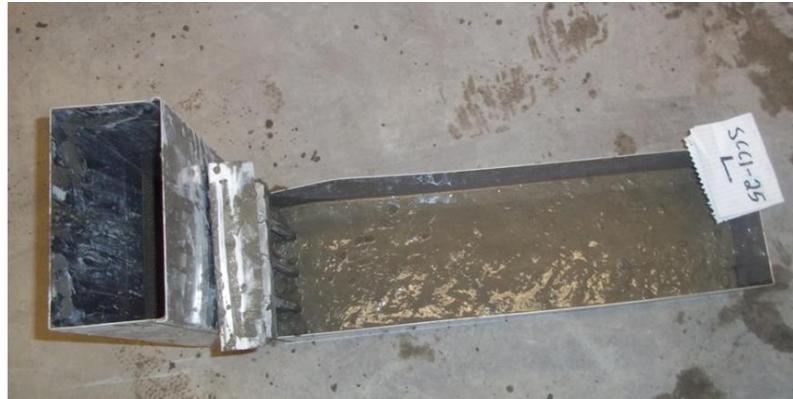
**Figure 4.3** Experimental setup for the L-Box test (0.75-25-L).
