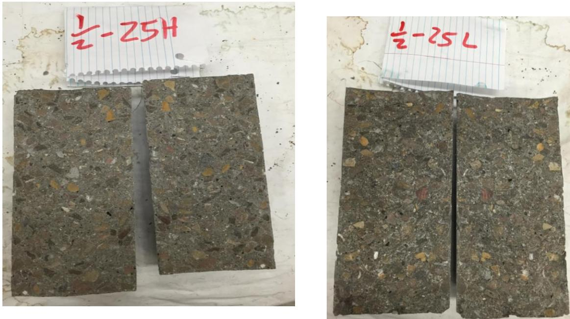
**Figure 4.9 Coarse aggregate distribution for hardened 05-25.**
