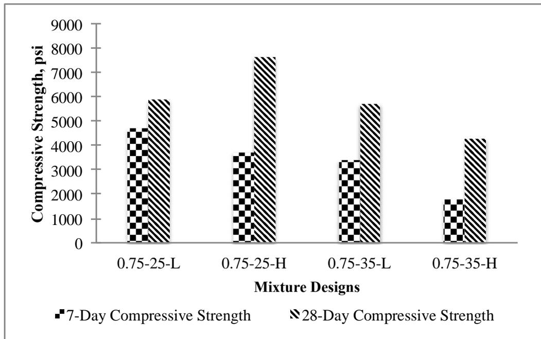
**Figure 6.1 Compressive strength for 0.75-in coarse aggregate SCC mixtures.**
