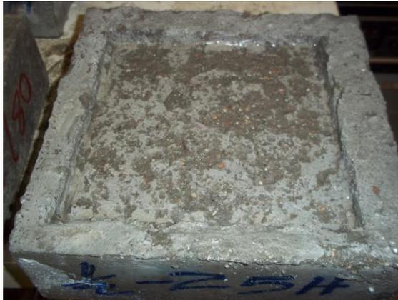
**Figure 6.17 0.5-25-H after 10 freezing and thawing cycles.**
