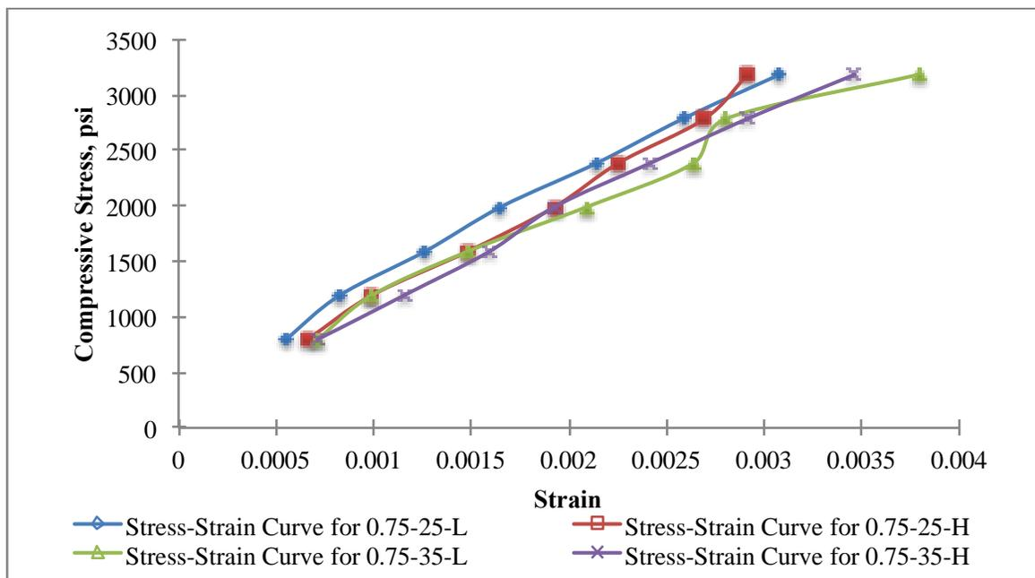
**Figure 6.3 Stress-strain curves for 0.75-in self-consolidating concrete mixture designs.**
