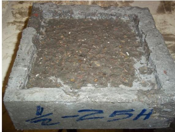
**Figure 6.21 0.5-25-H after 30 freezing and thawing cycles.**
