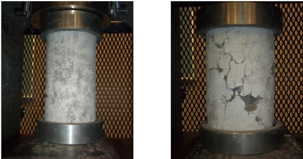
**Figure 4.5 Experimental setup for Compressive Strength testing.**
