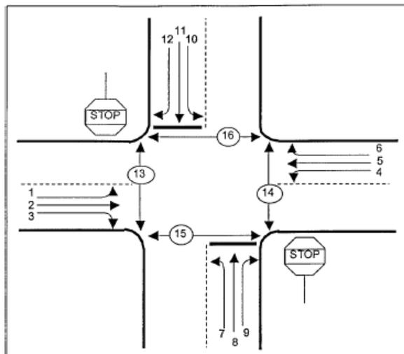
**Figure 2 Movement Numbers for Right-turn Volume Adjustment**
