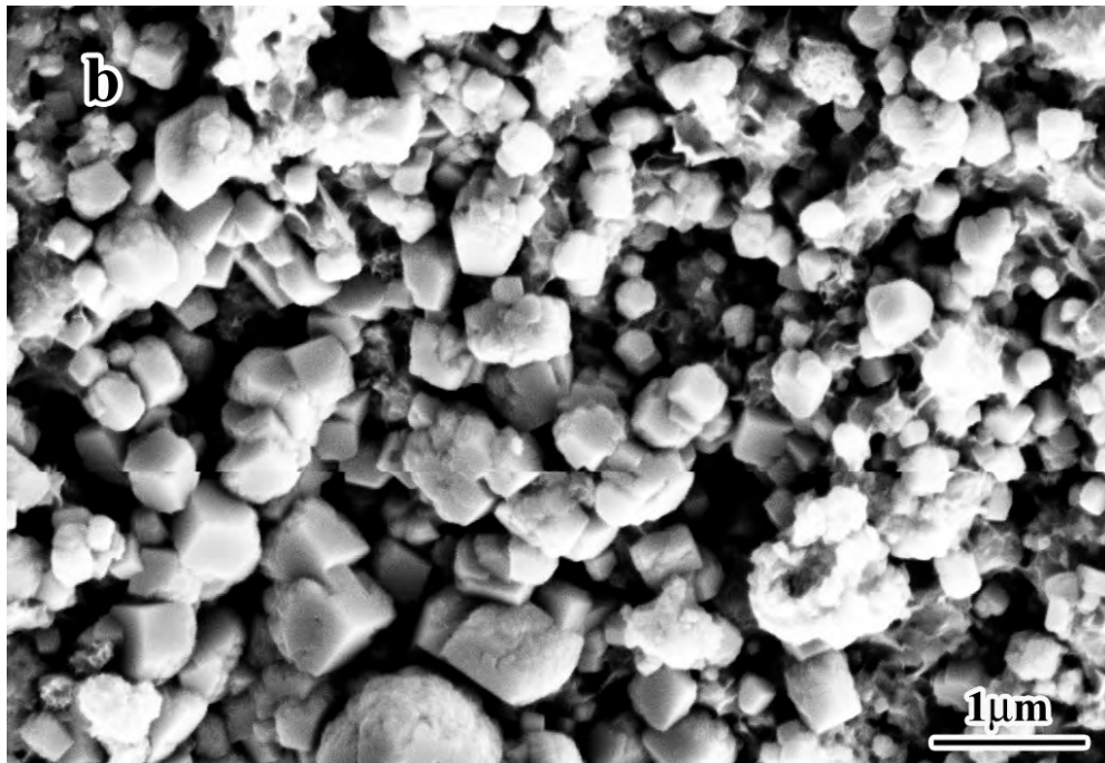
Figure 6- 18 SEM microstructure images of the HMWM coatings after 15 F/T cycles with exposure to NaCl solution a) low magnification, b) high magnification.
