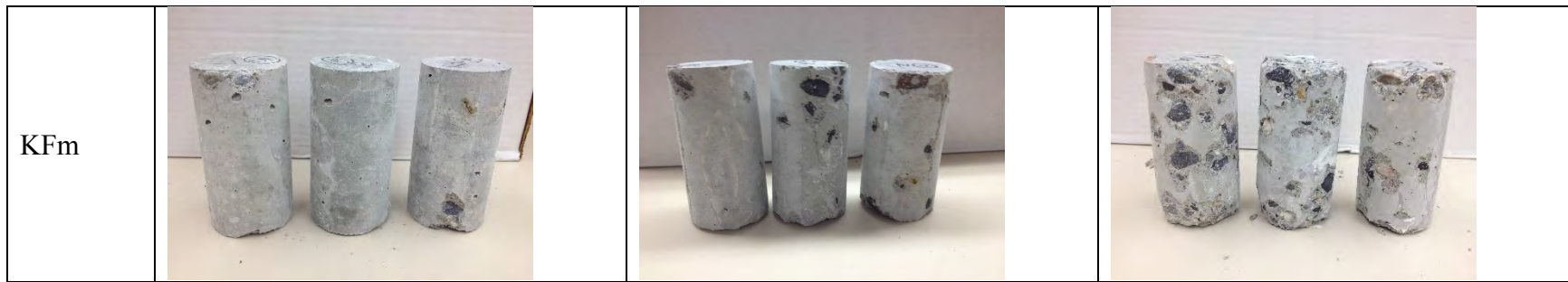
Figure 5- 4 The external morphologies of laboratory-fabricated concrete cylinders exposed to various deicer solutions after 3, 7, and 15 F/T and W/D cycles.
