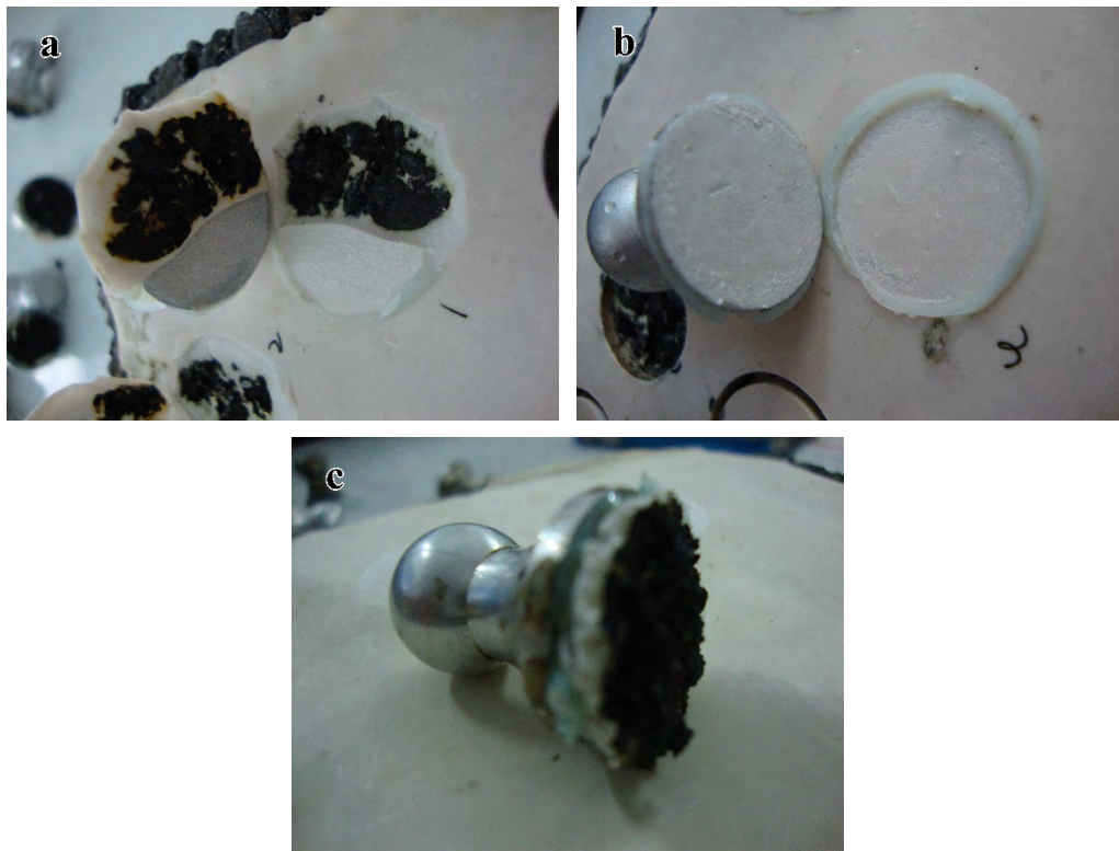
Figure 6- 10 External failure images of the acrylic polymer coating on asphalt concrete, a) failure of both polymer and asphalt, b) failure of polymer, and c) failure of asphalt.
