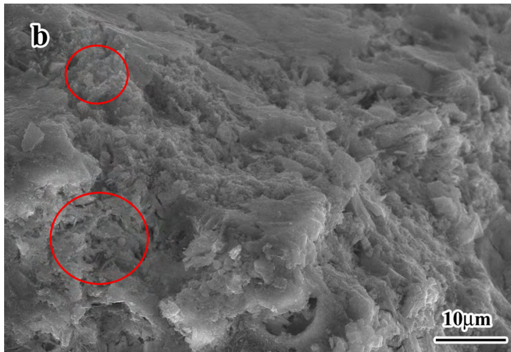
Figure 4- 4 SEM fracture surface morphologies of the samples cored from the Creek site with a) low and b) high magnification.
