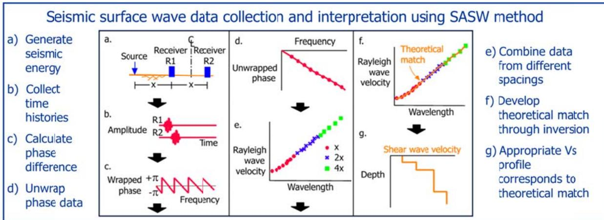
Figure 1. Diagrammatic explanation of the SASW method which is one of several used to generate detailed VS profiles nonintrusively by capitalizing on the dispersive characteristic of Rayleigh-type surface waves when moving through layered media.
