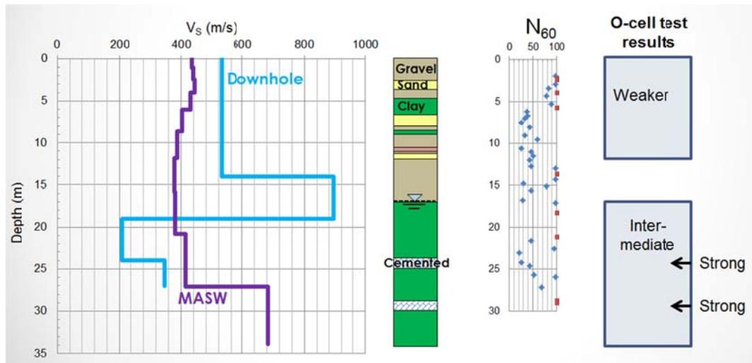
Figure 5. Hole 2: Measured VS, sediment lithology,  $N_{60}$  and general observations from Osterberg cell (O-cell) test.
