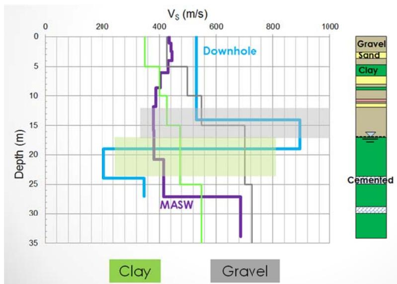
Figure 4. Hole 2: Measured VS compared against local representative profiles (green for clay, gray for gravel), and sediment lithology. Color-coded rectangles reflect variability of data from which representative profiles were created, at depths of interest for this site (gravel layer at ~12-17 m and clay layer at ~17-24 m).
