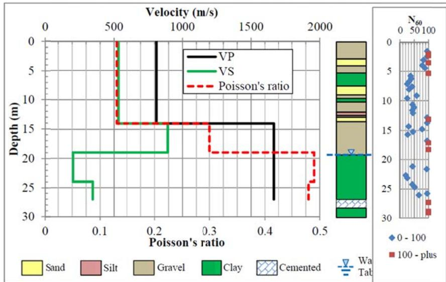
Figure 2. VP, VS, Poisson's ratio, sediment log and  $N_{60}$  for Hole 2 at CC215/US95 site. (Figure 3.13 from Samuel 2015.)
