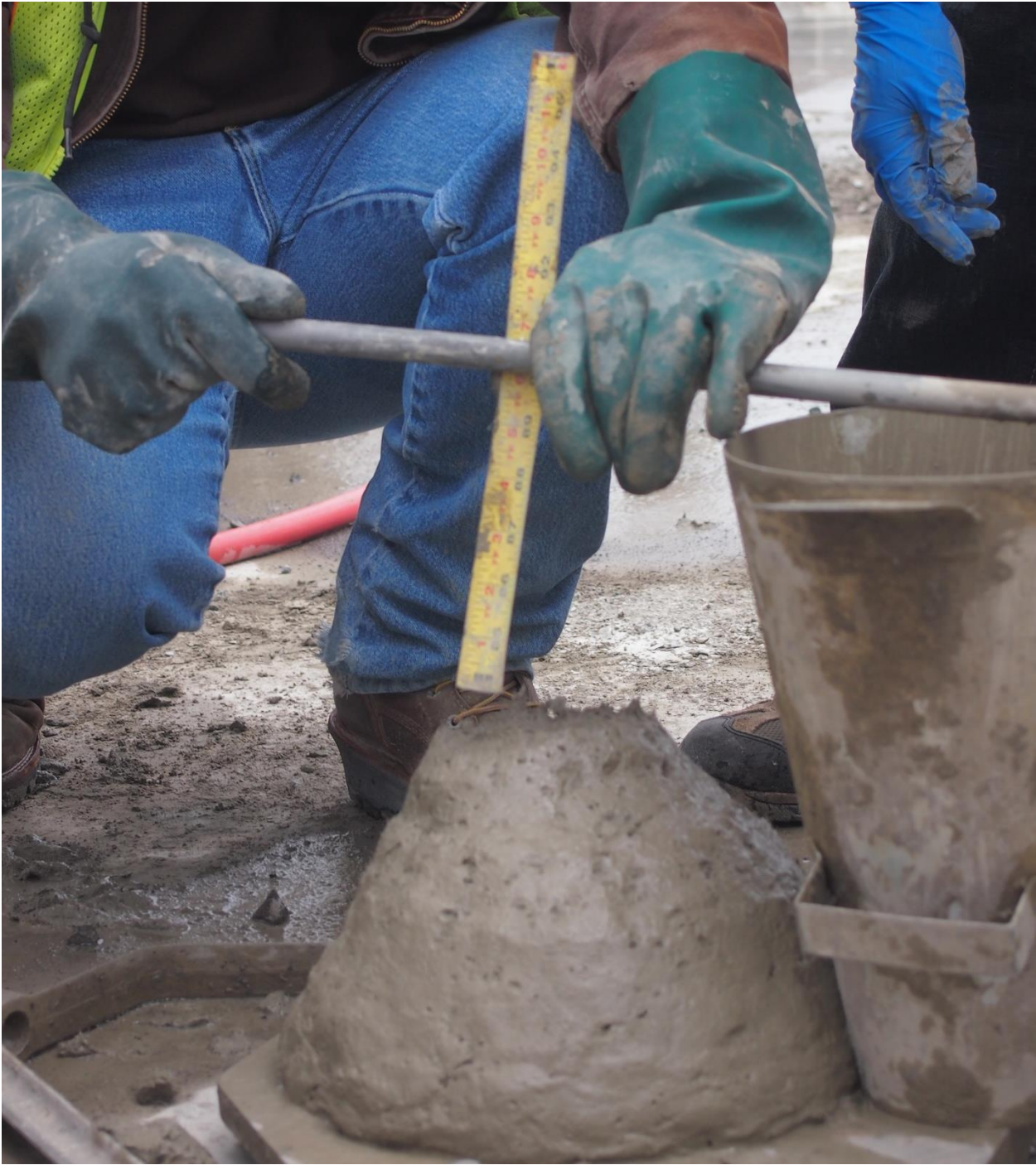
Figure 69 Slump of Fresh MECC Material from Trial Batch A.
