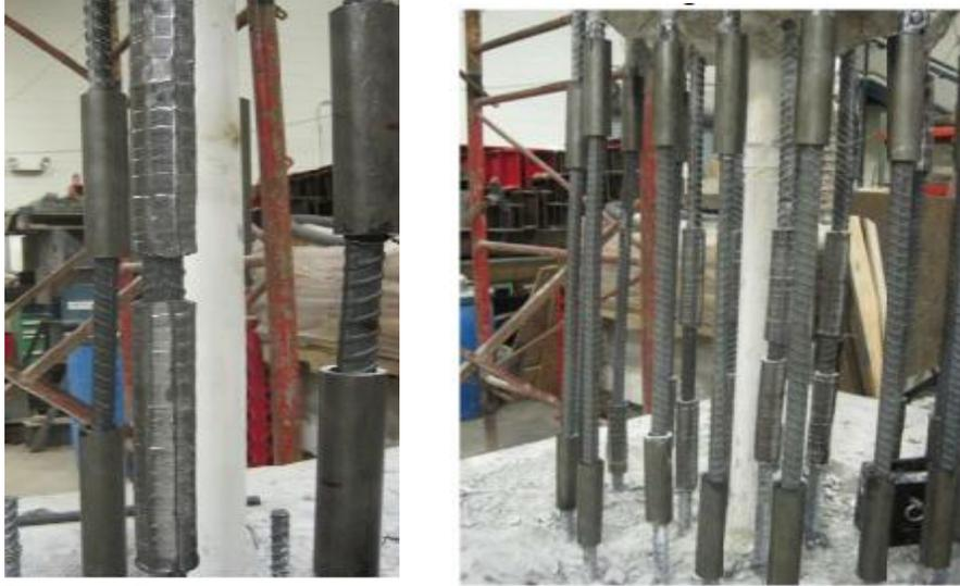
**Figure D.22** Damaged bars and coupler repair (Saini et al, 2013)
