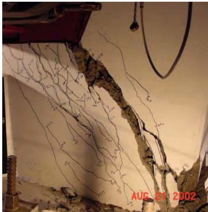
**Figure D.8** Angled stem wall failure of specimen (Bozorgzadeh et. al. 2004)
