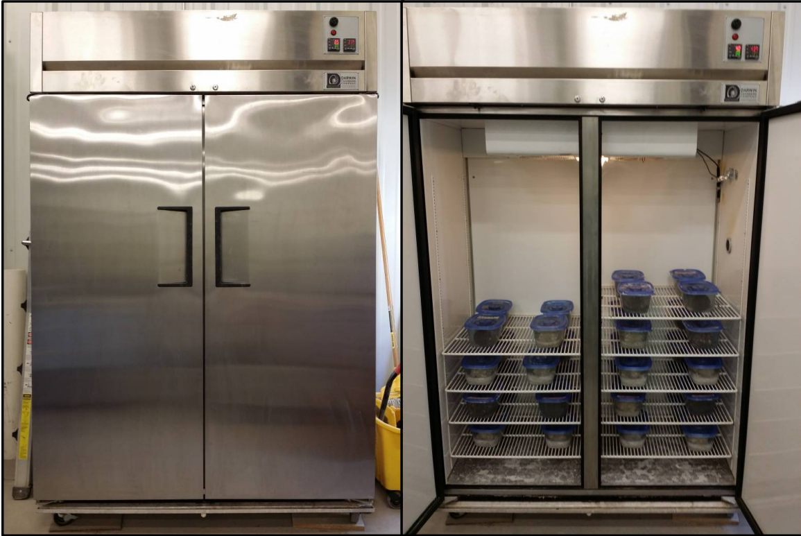
Figure 2-17: Cooler Used for Pre-Cooling of Freeze/Thaw Samples
