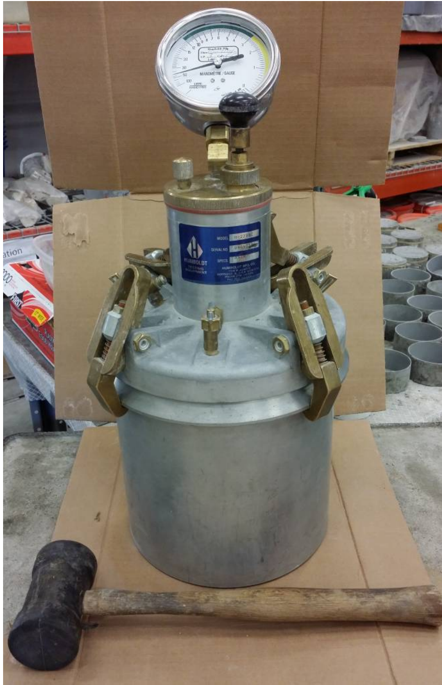
Figure 2-5: Air Content Meter - Pressure Type
