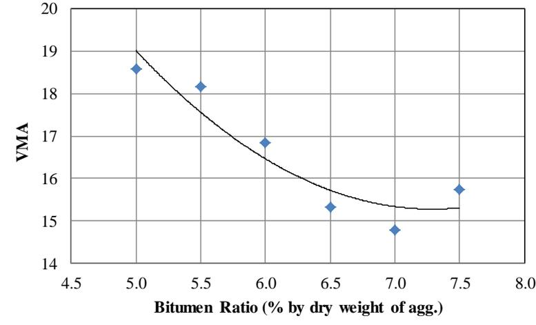
**Figure B-6 Variation of mix design properties with binder content for AC20 + 15%Am#40**
