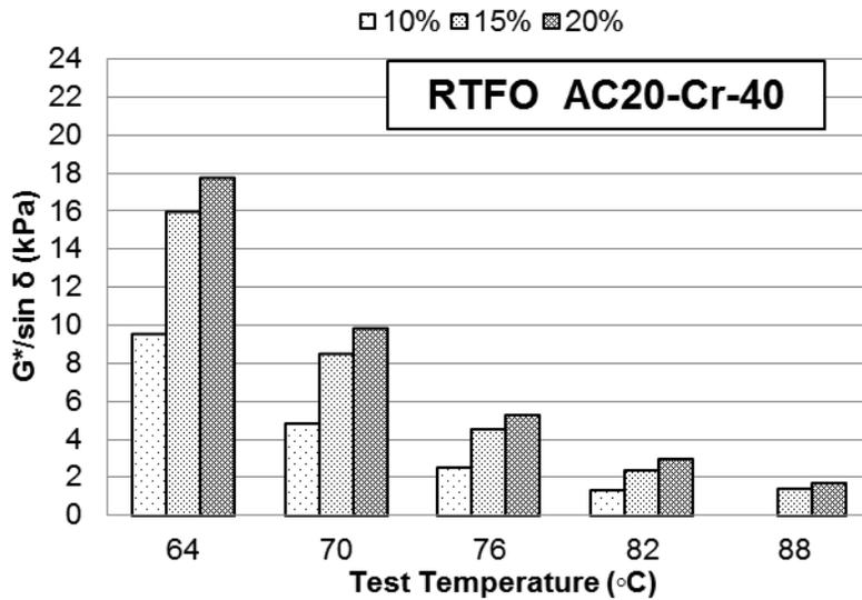
Figure A-87  $G^*/\sin(\delta)$  at different temperatures for RTFO B6416 mixed with CRM Cryogenic #40
