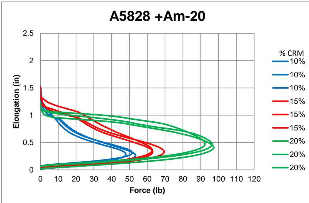
**Figure A-42 Force vs Elongation for A5828 mixed with Ambient #20**
