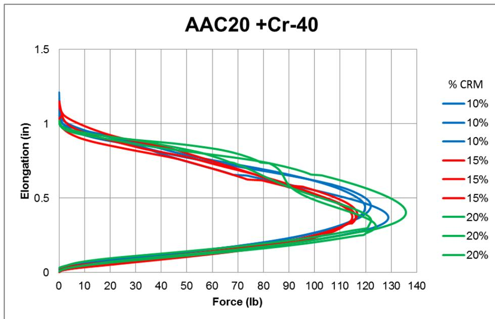
**Figure A-54 Force vs Elongation for AAC20 mixed with Cryogenic #40**
