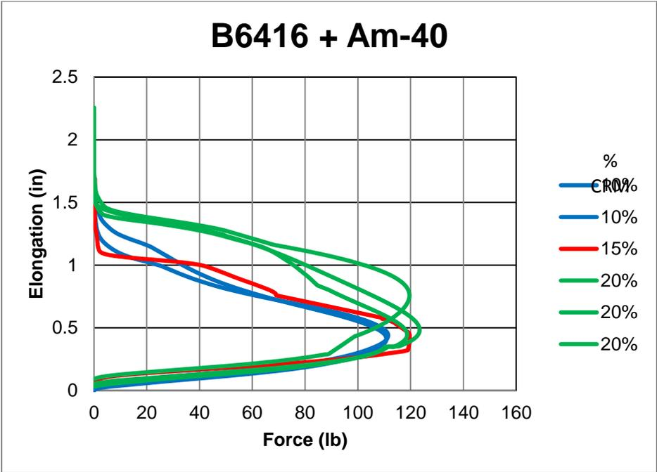
Figure A-47 Force vs Elongation for B6416 mixed with Ambient #40
