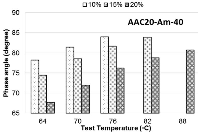
**Figure A-24 Phase angle at different temperatures for AAC20 mixed with CRM Ambient #40**
