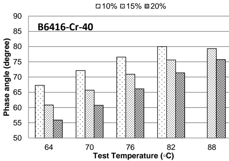
**Figure A-94 Phase angle at different temperatures for RTFO B6416 mixed with CRM Cryogenic #40**
