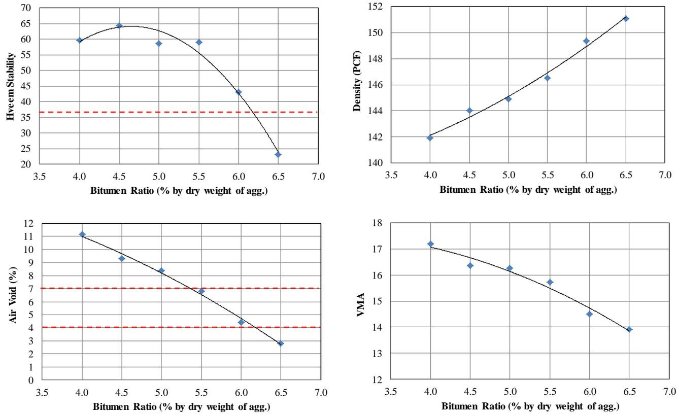
**Figure B-1 Variation of mix design properties with binder content for B76-22NV**
