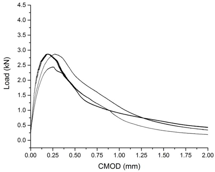
**Figure B-28 The load curves of A7622VTR mixtures under DCT test**
