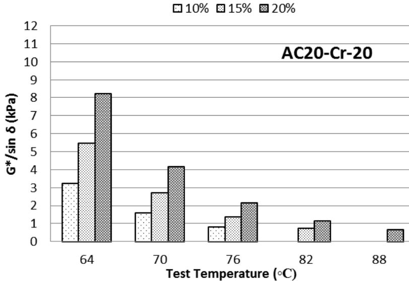
Figure A-12  $G^*/\sin(\delta)$  at different temperatures for AAC20 mixed with CRM Cryogenic #20
