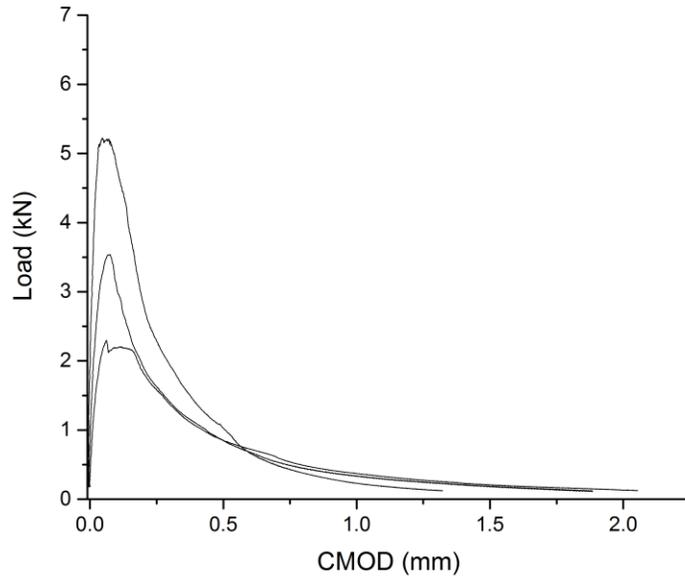
**Figure B-8 The load curves of A6428NV mixtures under SCB test**
