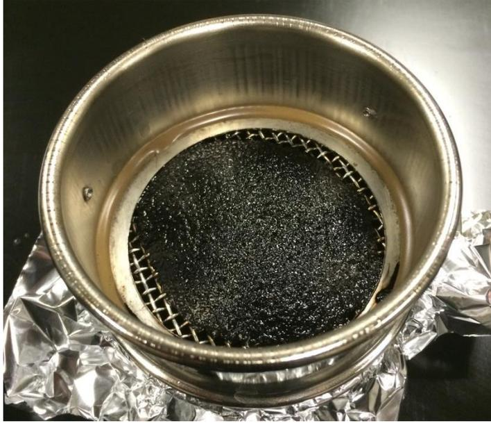
**Figure A-68 particles retained on sieve for A5828-Cr-40-20**
