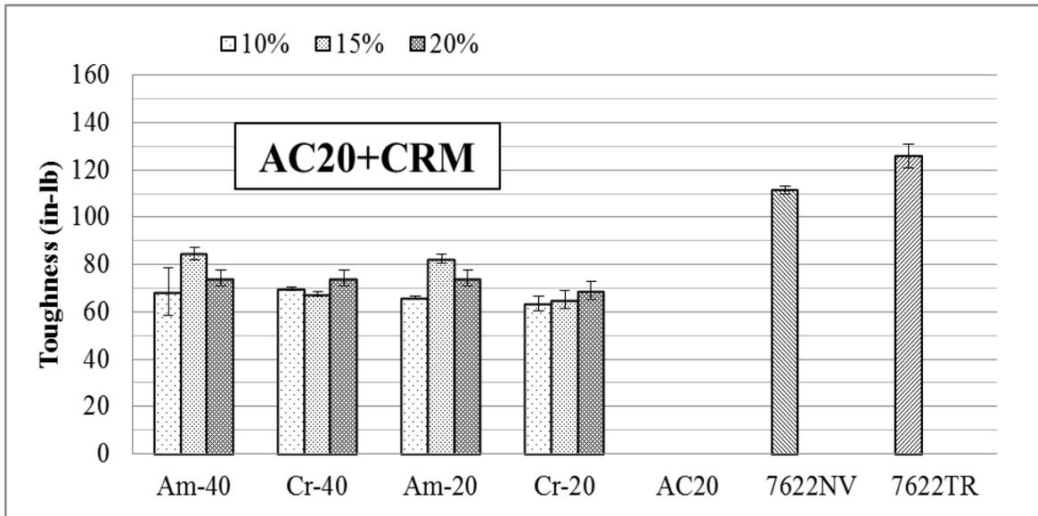
**Figure A-59 Toughness of AAC20 samples mixed with CRM, polymer modified and terminal blend**
