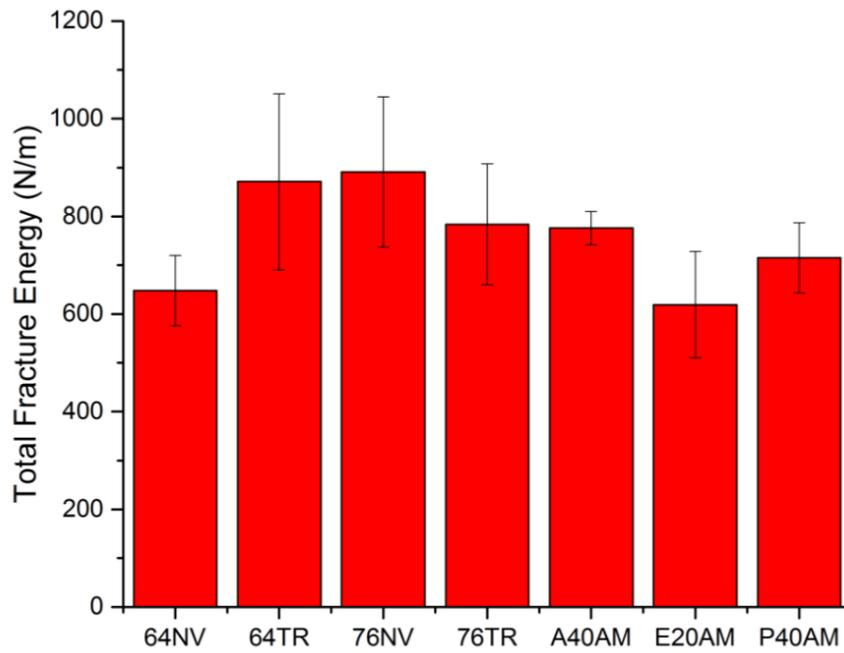
Figure B-17 The average total fracture energy values of various mixtures under SCB test
