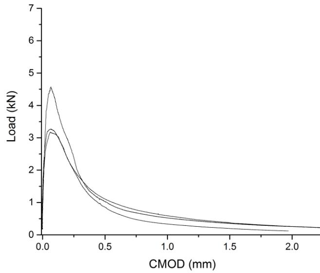
**Figure B-14** The load curves of A5828-AM-40-15 mixtures under SCB test
