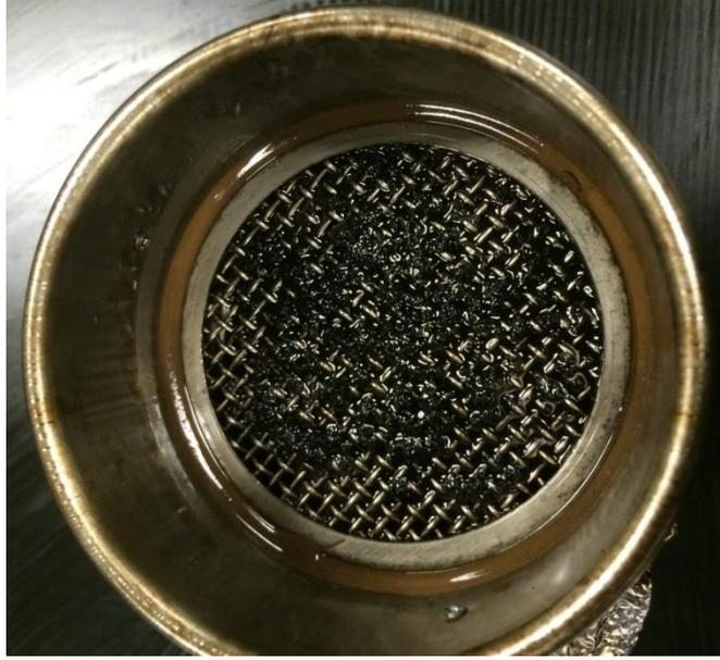
**Figure A-74 particles retained on sieve for AAC20-Cr-20-10**
