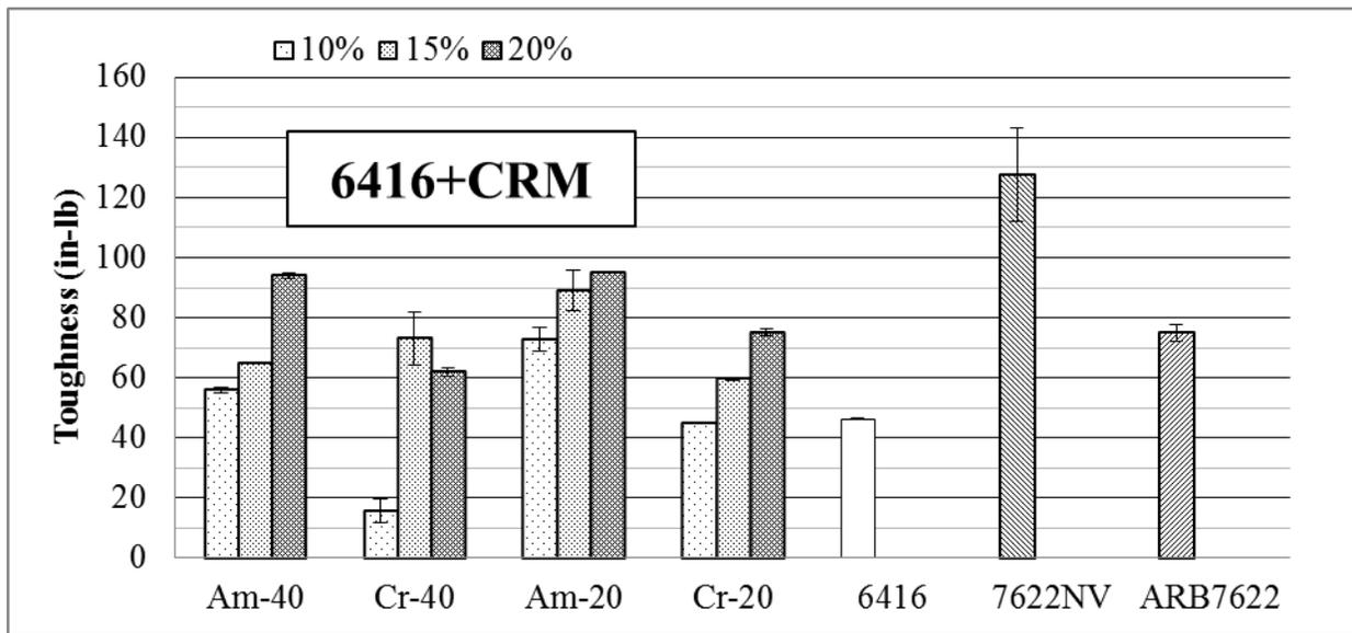
Figure A-58 Toughness of B6416 samples mixed with CRM, polymer modified and asphalt rubber binder
