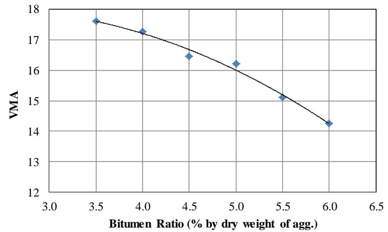
Figure B-2 Variation of mix design properties with binder content for B76-22NVTR
