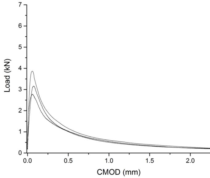
**Figure B-12 The load curves of AAC20-AM-40-15 mixtures under SCB test**
