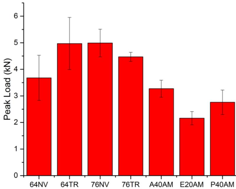
Figure B-16 The average peak load values of various mixtures under SCB test
