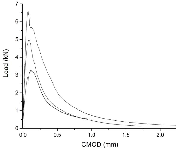
**Figure B-9 The load curves of A6428NVTR mixtures under SCB test**
