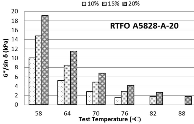
Figure A-80  $G^*/\sin(\delta)$  at different temperatures for RTFO B6416 mixed with CRM Ambient #20
