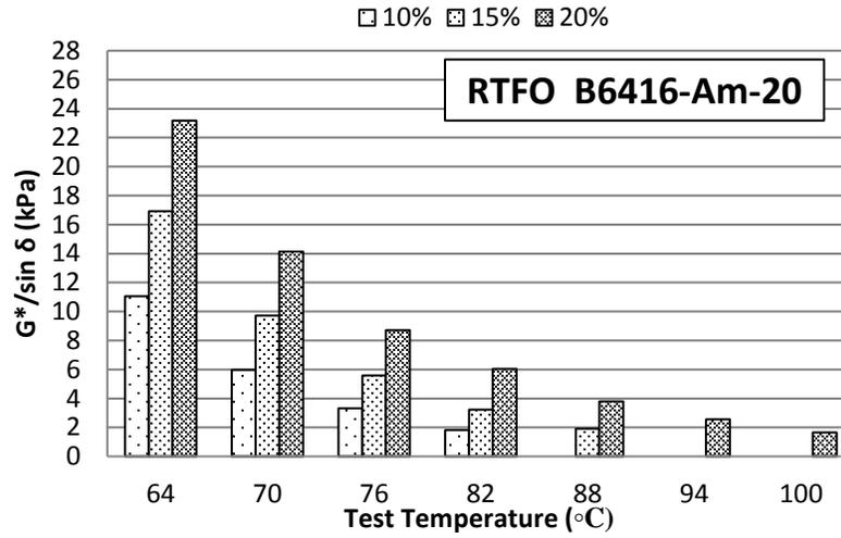
**Figure A-84  $G^*/\sin(\delta)$  at different temperatures for RTFO B6416 mixed with CRM Ambient #20**
