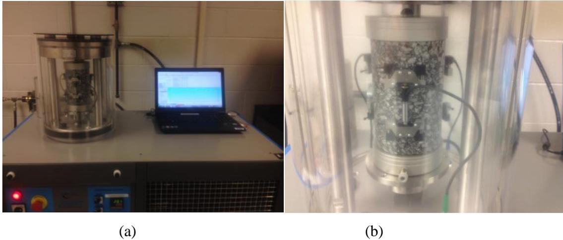
**Figure 5.4. Dynamic modulus tests of various alternative polymerized mixtures**
