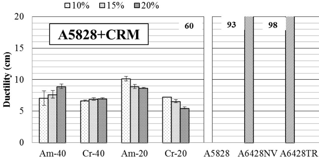
Figure A-31 Ductility of A5828 mixed with CRM, polymer modified and terminal blend
