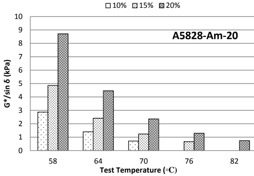
**Figure A-3  $G^*/\sin(\delta)$  at different temperatures for A5828 mixed with CRM Ambient #20**
