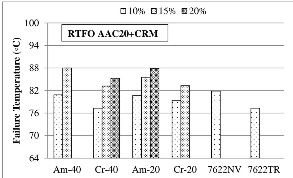
**Figure A-92 Failure temperature for RTFO AAC20 and mixed with CRM, and polymer modified 7622 and terminal blend tire rubber**
