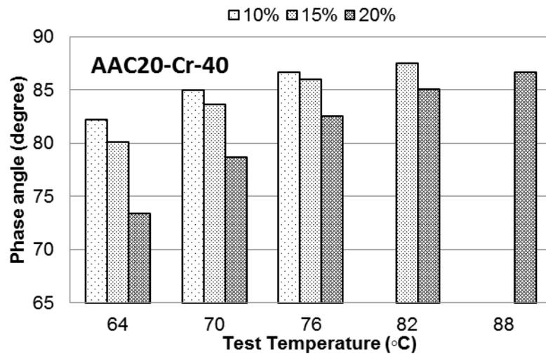
**Figure A-25 Phase angle at different temperatures for B6416 mixed with CRM Cryogenic #40**
