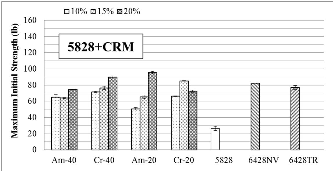
Figure A-63 Maximum Initial Strength of A5828 samples mixed with CRM, polymer modified and terminal blend
