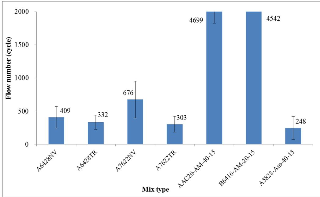
**Figure B-24 Flow number values of various mixtures at 59° C**
