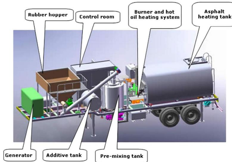
**Figure 2.9. A Typical On-Site Blending System for Rubberized Binder (28)**
