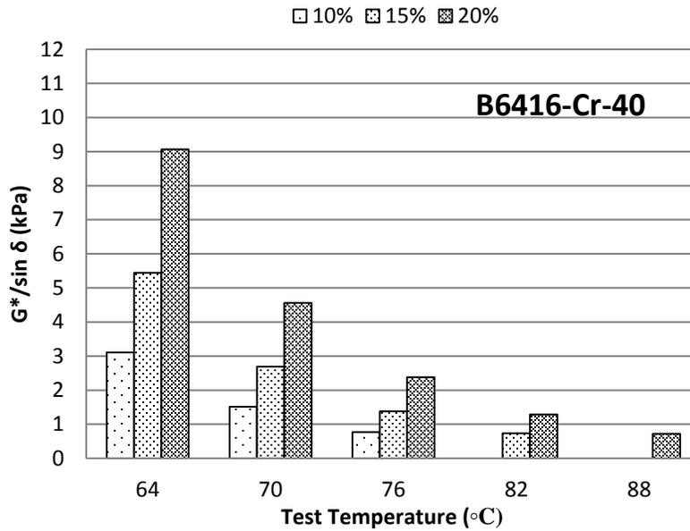
**Figure A-6  $G^*/\sin(\delta)$  at different temperatures for B6416 mixed with CRM Cryogenic #40**
