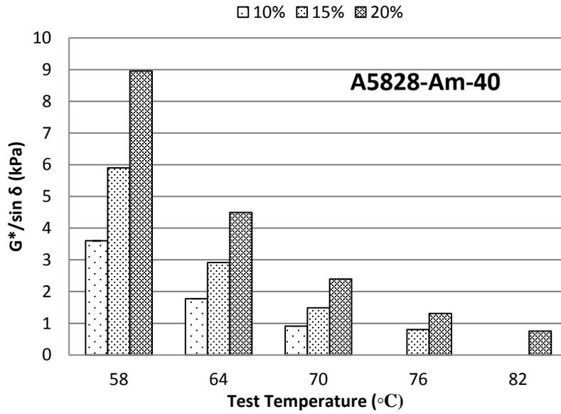
Figure A-1  $G^*/\sin(\delta)$  at different temperatures for A5828 mixed with CRM Ambient #40
