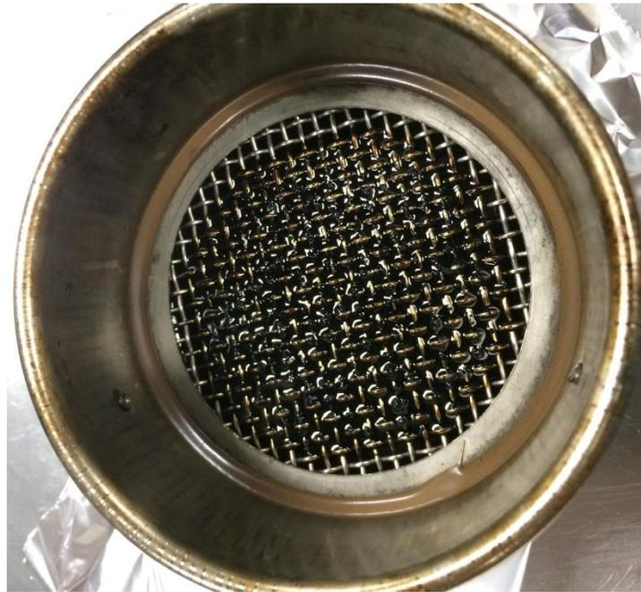
**Figure A-75 particles retained on sieve for AAC20-Cr-40-10**
