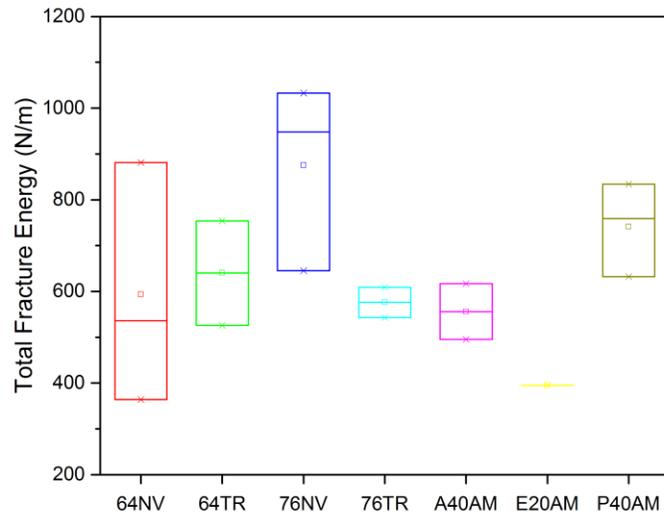
**Figure B-32 The fracture energy of various mixtures under DCT test**
