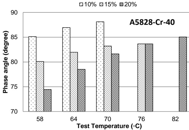
Figure A-17 Phase angle at different temperatures for A5828 mixed with CRM Cryogenic
