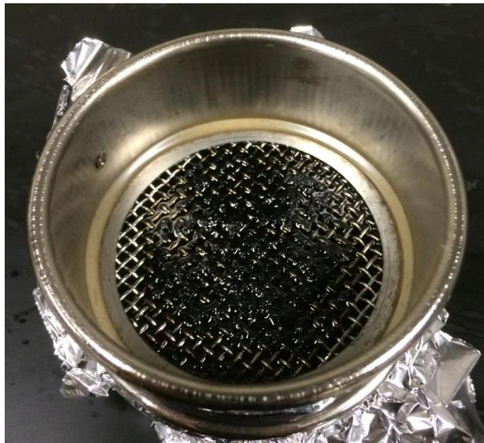
**Figure A-67** particles retained on sieve for A5828-Cr-40-15
