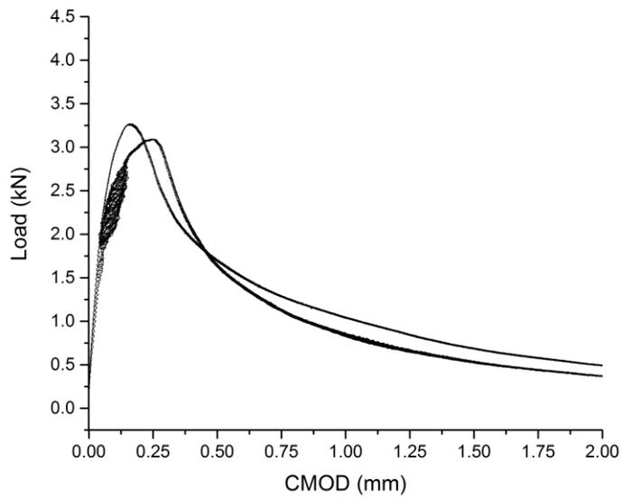
**Figure B-29 The load curves of AAC20-AM-40-15 mixtures under DCT test**
