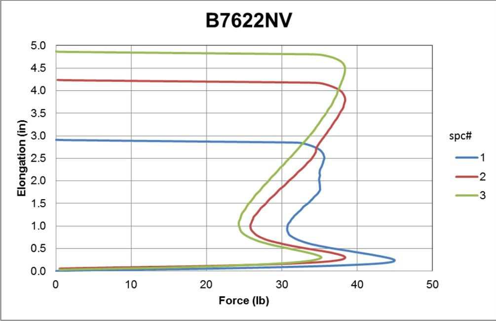
**Figure A-45 Force vs Elongation for B7622NV from source B**
