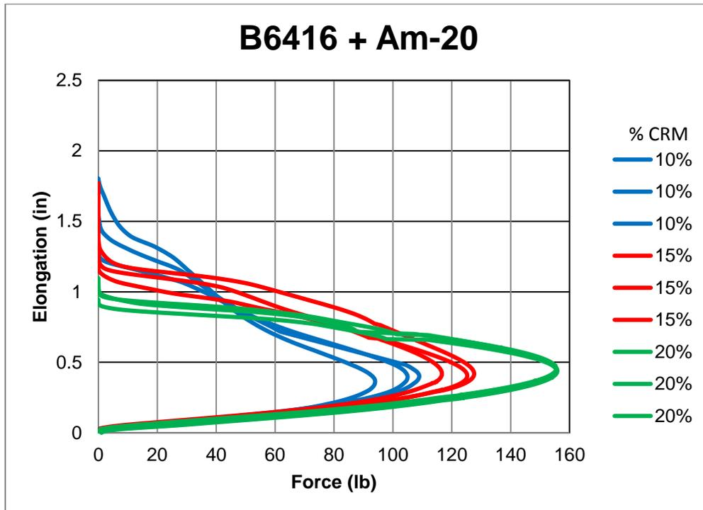
**Figure A-49 Force vs Elongation for B6416 mixed with Ambient #20**
