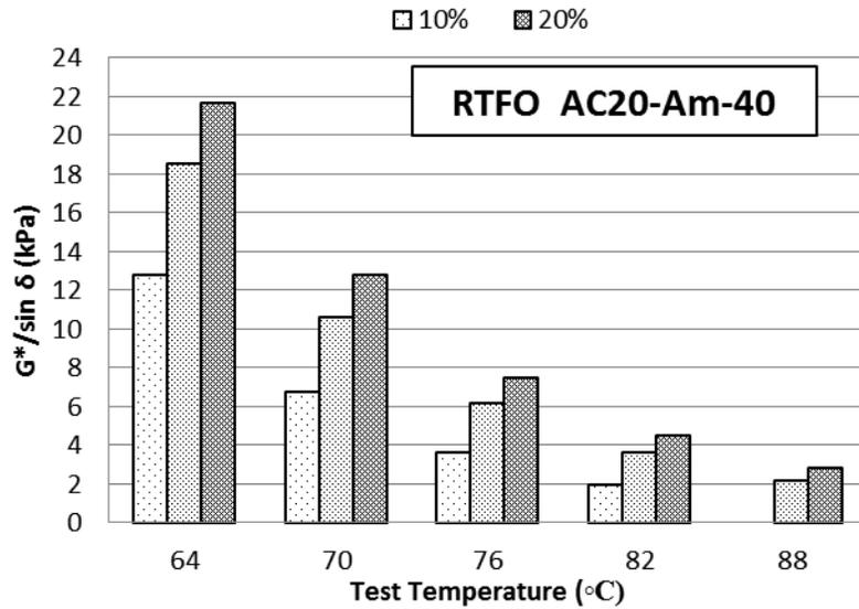
Figure A-86  $G^*/\sin(\delta)$  at different temperatures for RTFO B6416 mixed with CRM Ambient #40
