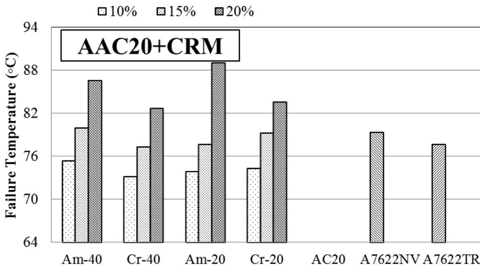
**Figure A-15 Failure temperature for AAC20 and mixed with CRM polymer, and terminal blend tire rubber**
