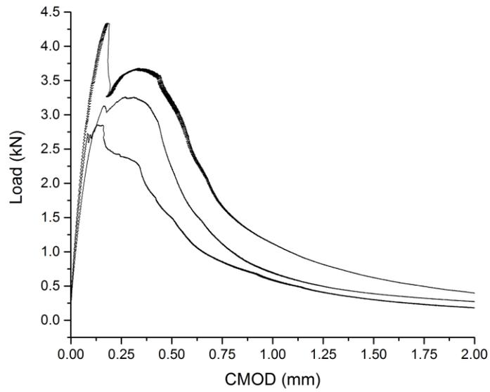
**Figure B-25 The load curves of A6428NV mixtures under DCT test**
