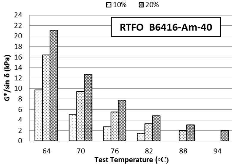
**Figure A-82  $G^*/\sin(\delta)$  at different temperatures for RTFO B6416 mixed with CRM Ambient #40**
