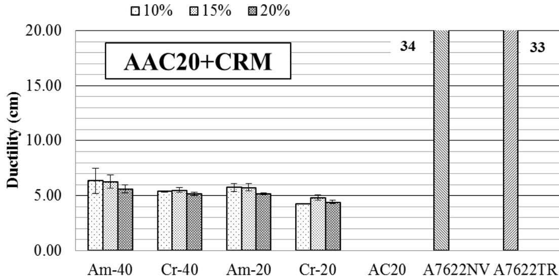
**Figure A-33 Ductility of AAC20 mixed with CRM, polymer modified and terminal blend**
