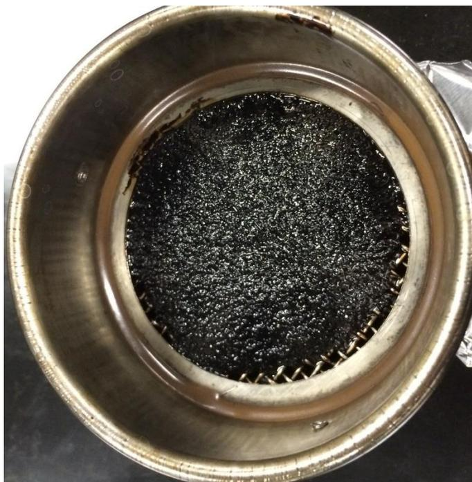
**Figure A-77 particles retained on sieve for AAC20-Cr-40-20**
