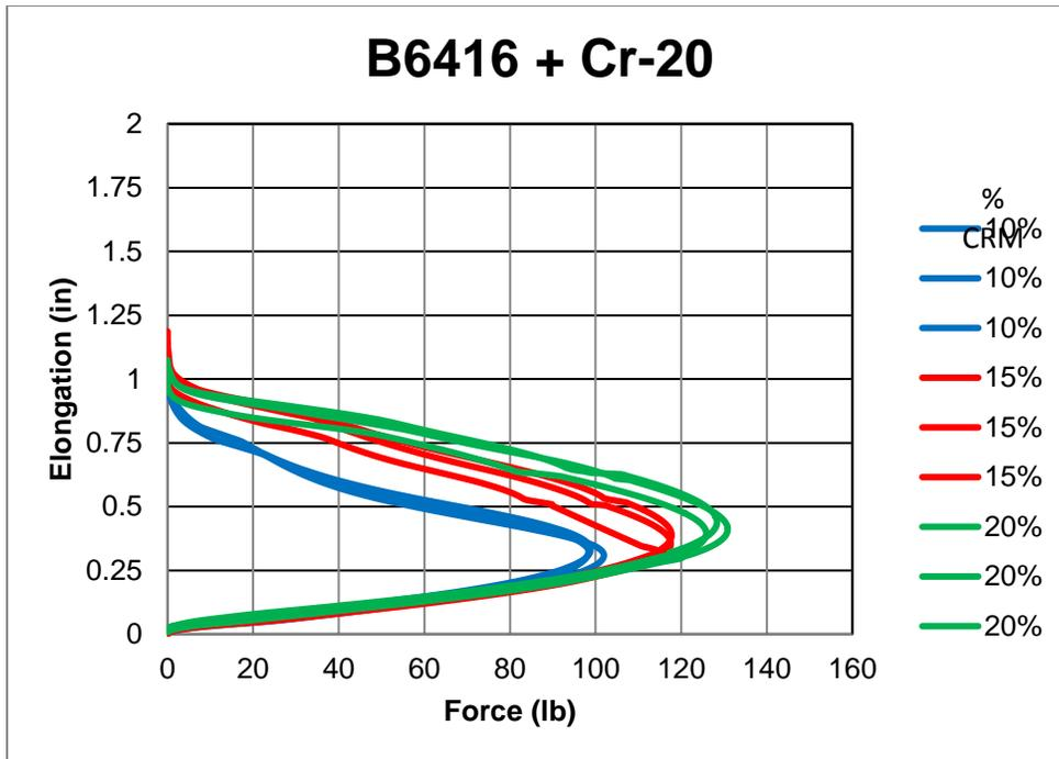
**Figure A-50 Force vs Elongation for B6416 mixed with Cryogenic #40**
