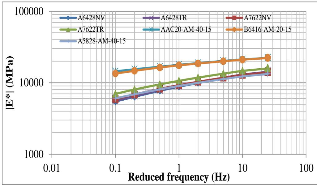
Figure B-18 Dynamic modulus values of various mixtures at 4° C
