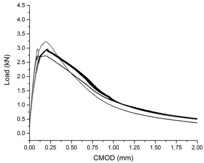
**Figure B-31 The load curves of A5828-AM-40-15 mixtures under DCT test**
