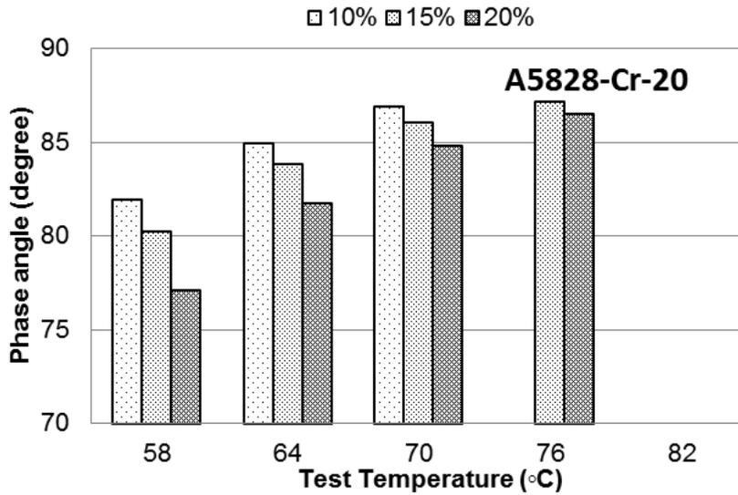
**Figure A-19 Phase angle at different temperatures for A5828 mixed with CRM Cryogenic #20**
