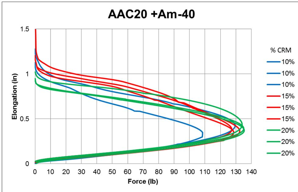
**Figure A-53 Force vs Elongation for AAC20 mixed with Ambient #40**
