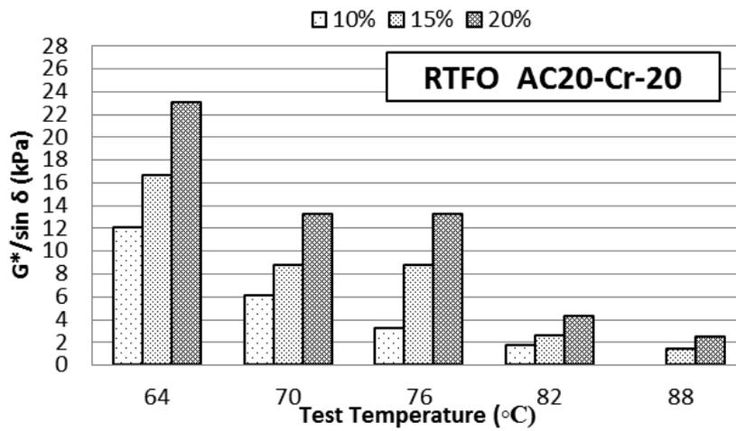
Figure A-89  $G^*/\sin(\delta)$  at different temperatures for RTFO B6416 mixed with CRM Cryogenic #20
