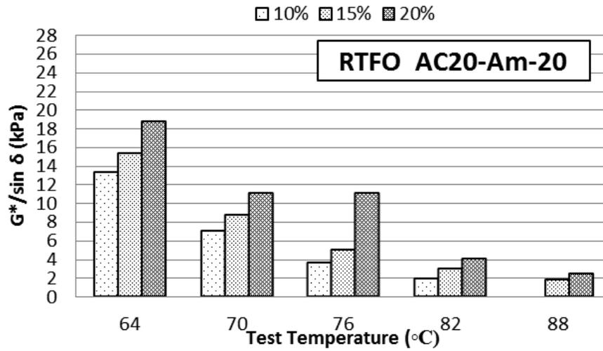
Figure A-88  $G^*/\sin(\delta)$  at different temperatures for RTFO B6416 mixed with CRM Ambient #20
