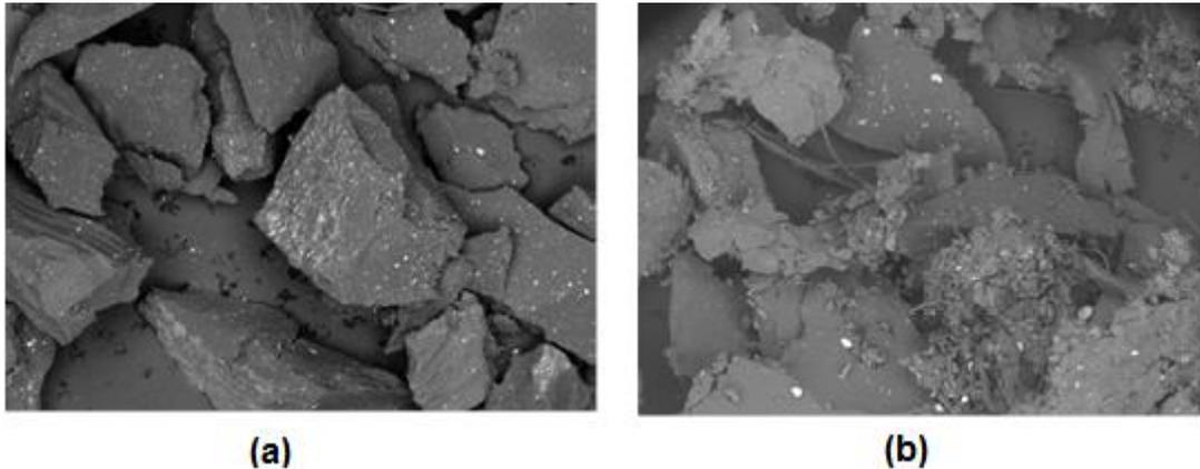
**Figure 2.8. SEM micrographs of a) Cryogenically and b) Ambient Ground CRM (at 30x magnification)**
