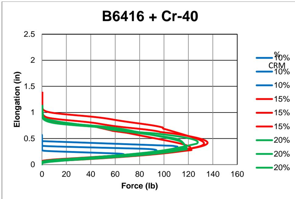
**Figure A-48 Force vs Elongation for B6416 mixed with Cryogenic #40**
