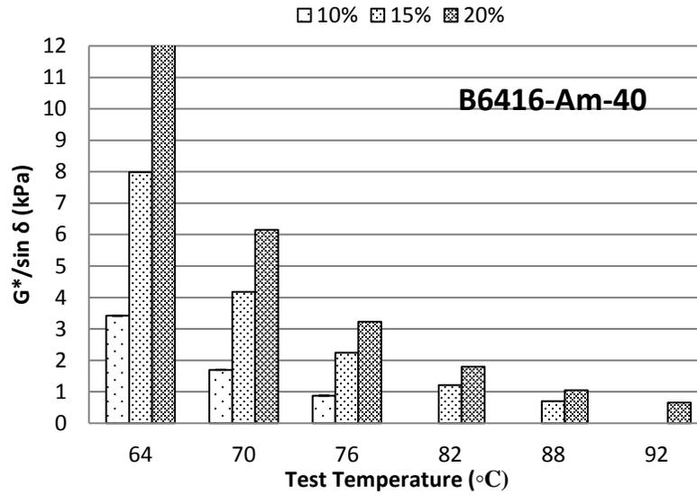
**Figure A-5  $G^*/\sin(\delta)$  at different temperatures for B6416 mixed with CRM Ambient #40**
