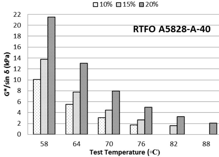
**Figure A-78  $G^*/\sin(\delta)$  at different temperatures for RTFO A5828 mixed with CRM Ambient #40**
