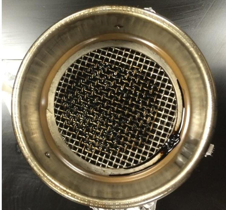
**Figure A-70 few particles retained on sieve for B6416-Cr-40-10**
