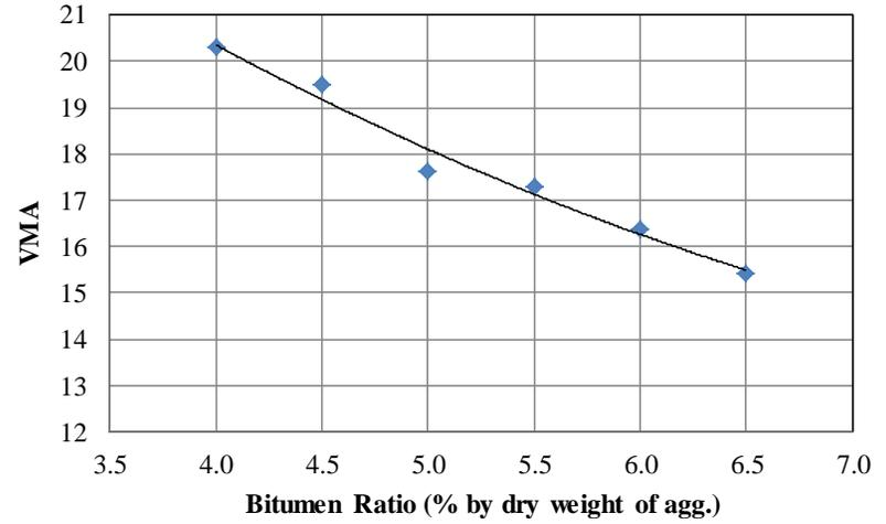
**Figure B-7 Variation of mix design properties with binder content for B58-28 + 15%Am#40**
