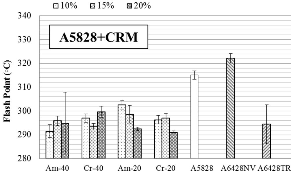
Figure A-34 Flash Point of A5828 samples mixed with CRM, polymer modified and terminal blend
