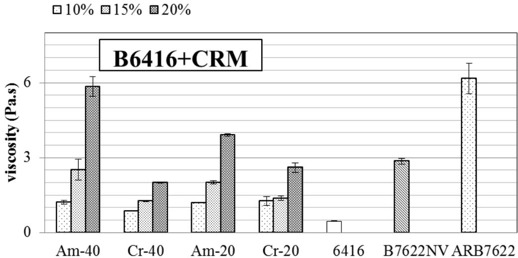
**Figure A-29 Viscosity of B6416 mixed with CRM, polymer and terminally blend tire rubber**
