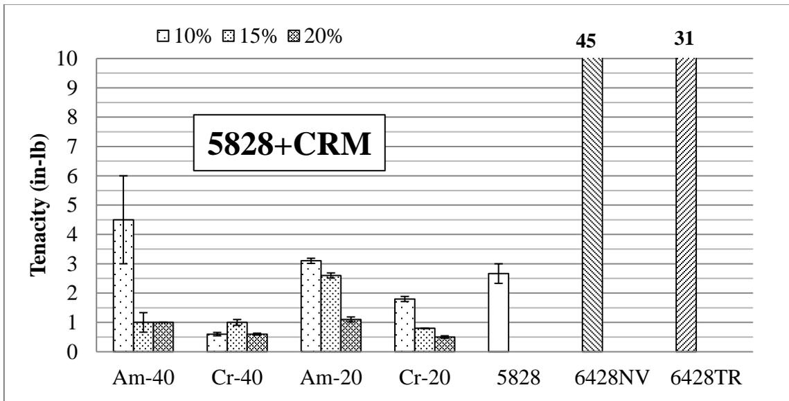
**Figure A-60 Tenacity of A5828 samples mixed with CRM, polymer modified and terminal blend**
