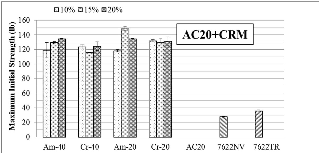
**Figure A-65 Maximum Initial Strength of AAC20 samples mixed with CRM, polymer modified and terminal blend**
