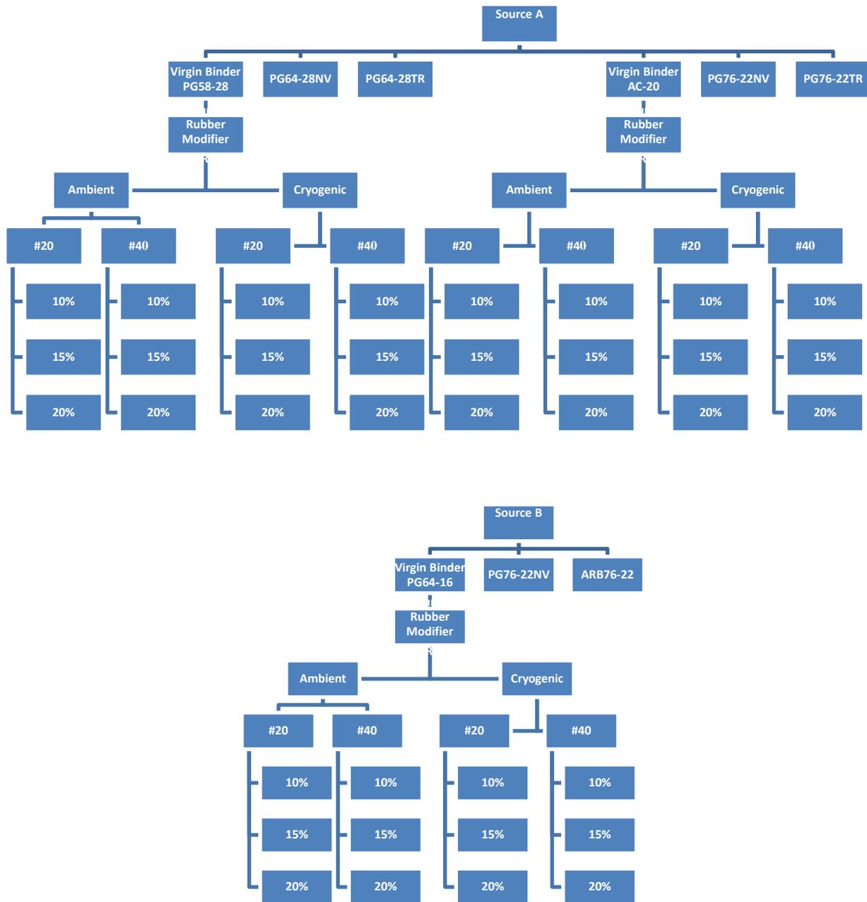
**Figure 3.2. Asphalt binder samples obtained from sources A and B and made in the lab**
