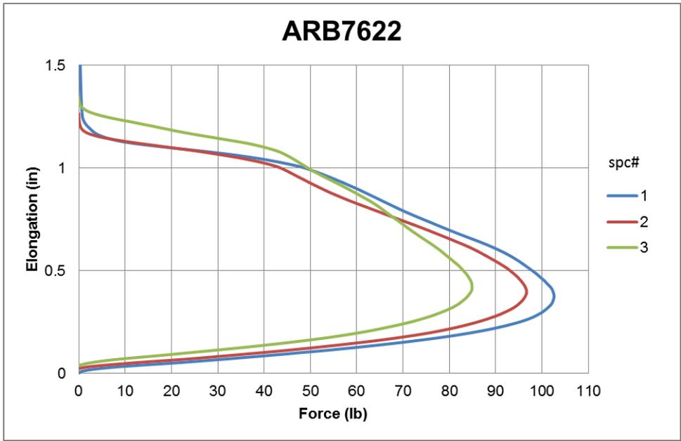
Figure A-46 Force vs Elongation for ARB7622 (asphalt rubber binder)
