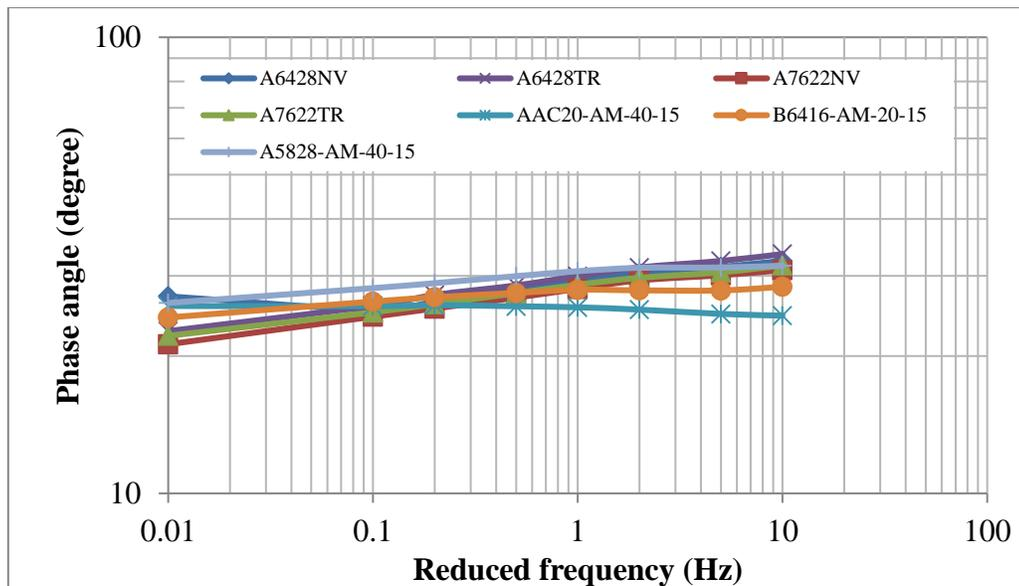
Figure B-23 Phase angle values of various mixtures at 40° C
