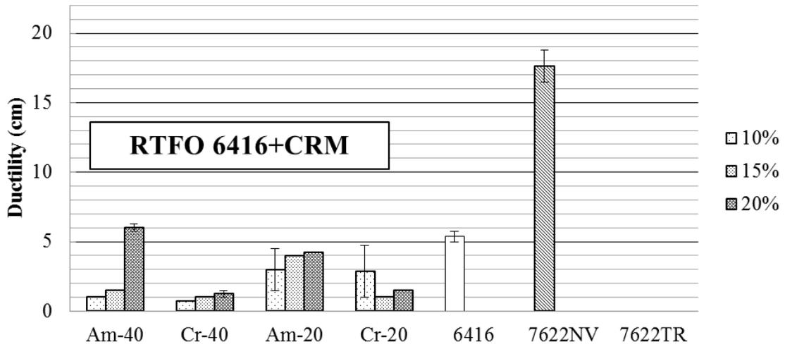
**Figure A-98 Ductility of RTFO B6416 mixed with CRM, polymer modified and asphalt rubber binder PG76-22**
