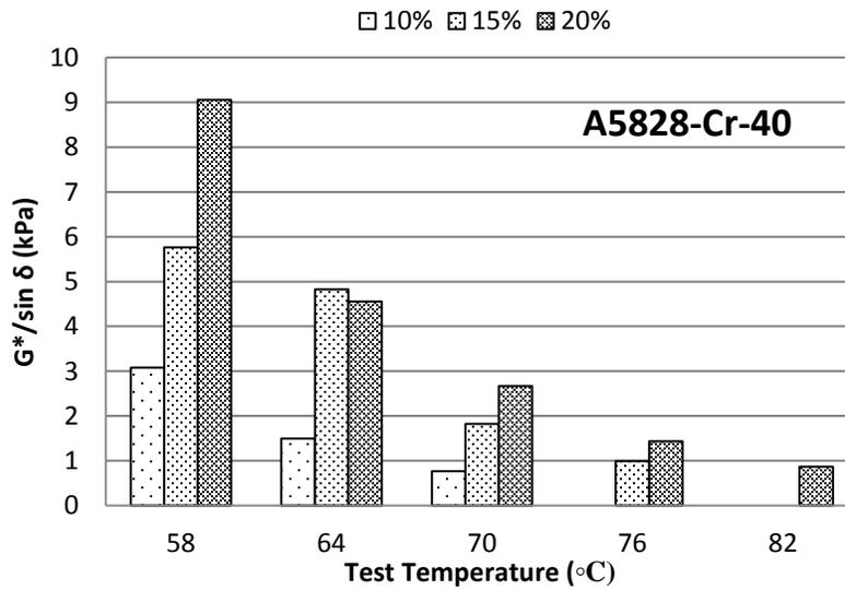
**Figure A-2  $G^*/\sin(\delta)$  at different temperatures for A5828 mixed with CRM Cryogenic #40**
