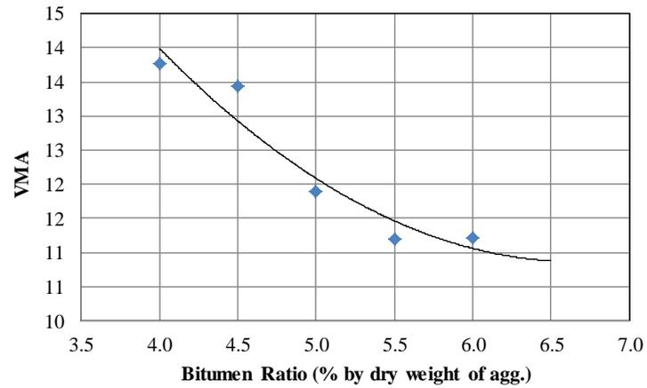
Figure B-3 Variation of mix design properties with binder content for B64-28NV
