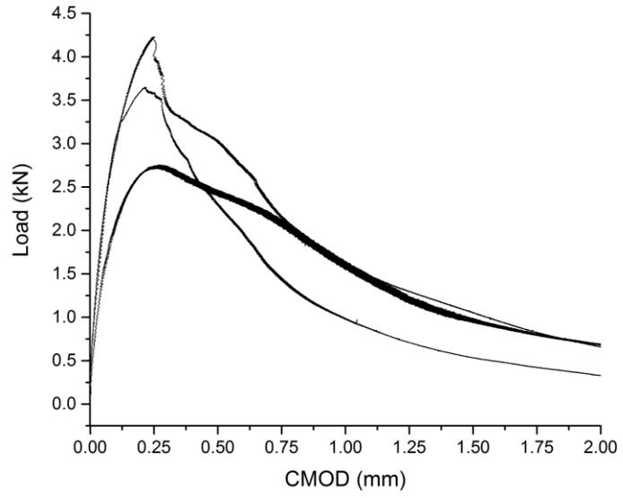
**Figure B-27 The load curves of A7622NV mixtures under DCT test**
