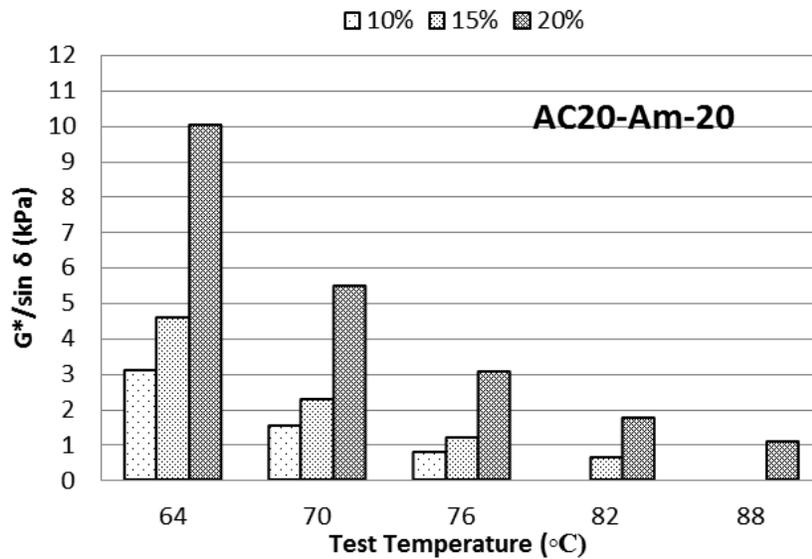
Figure A-11  $G^*/\sin(\delta)$  at different temperatures for AAC20 mixed with CRM Ambient #20
