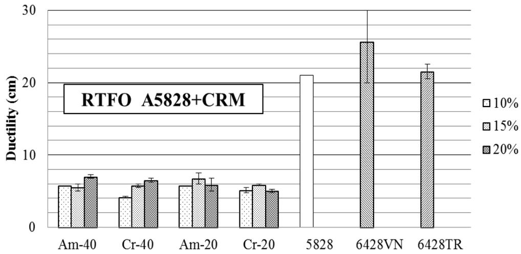
**Figure A-97 Ductility of RTFO A5828 mixed with CRM, polymer modified and terminal blend tire rubber PG64-28**
