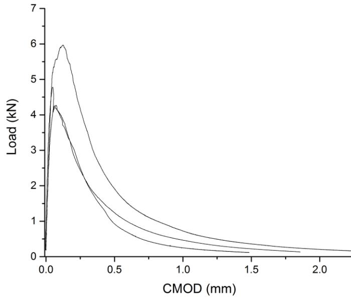
**Figure B-10 The load curves of A7622NV mixtures under SCB test**
