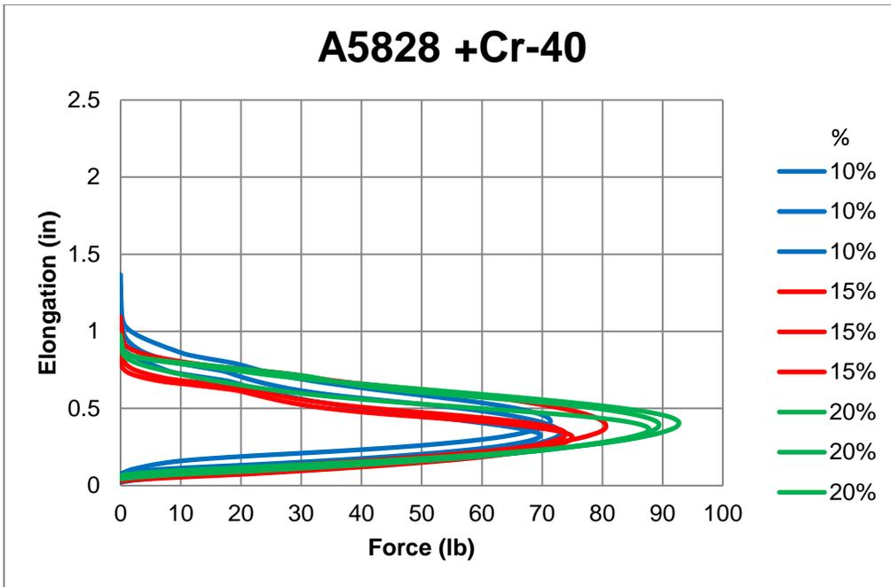
**Figure A-41 Force vs Elongation for A5828 mixed with Cryogenic #40**
