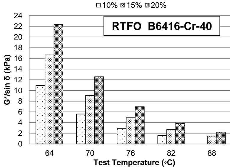
**Figure A-83  $G^*/\sin(\delta)$  at different temperatures for RTFO B6416 mixed with CRM Cryogenic #40**
