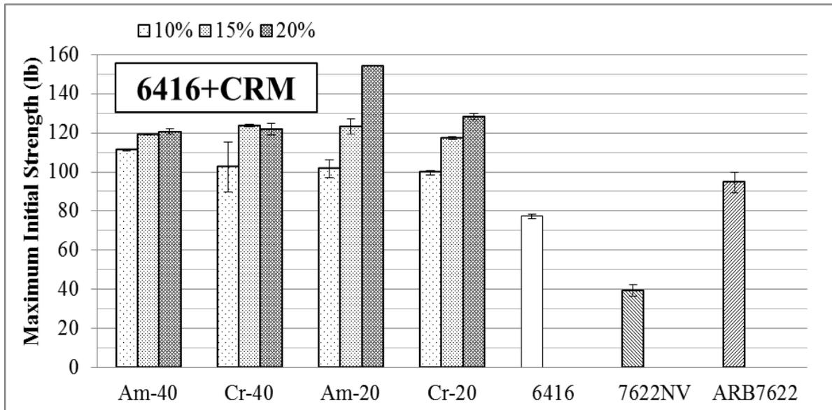
Figure A-64 Maximum Initial Strength of B6416 samples mixed with CRM, polymer modified and asphalt rubber binder
