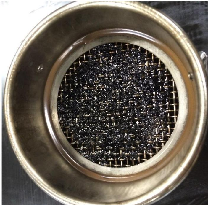
**Figure A-76 particles retained on sieve for AAC20-Cr-40-15**
