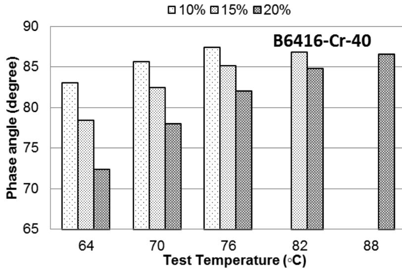
**Figure A-21 Phase angle at different temperatures for B6416 mixed with CRM Cryogenic #40**
