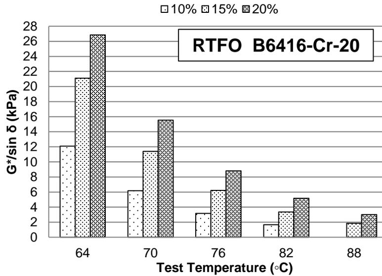
**Figure A-85  $G^*/\sin(\delta)$  at different temperatures for RTFO B6416 mixed with CRM Cryogenic #20**
