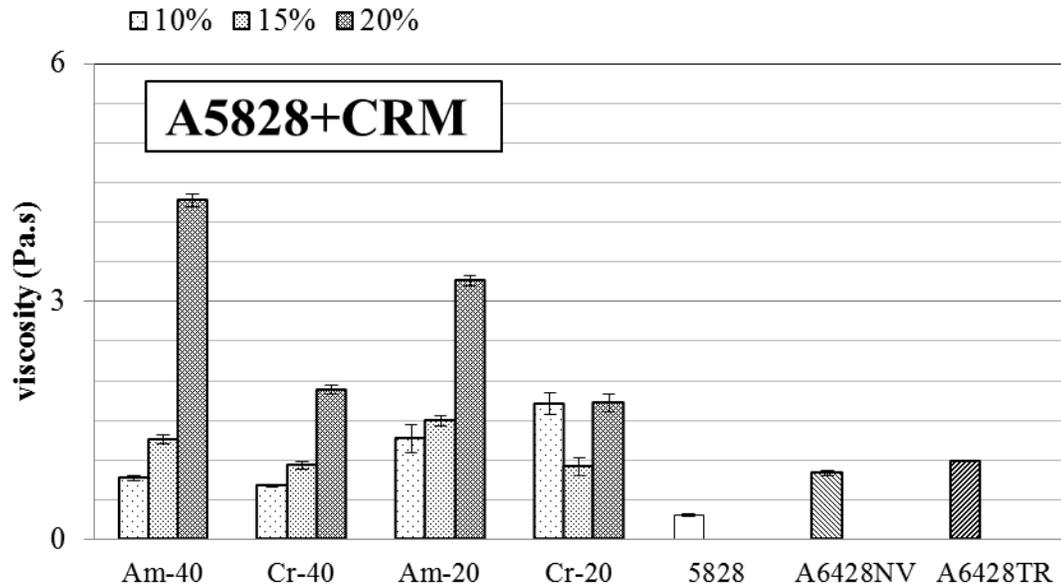
**Figure A-28 Viscosity of A5828 mixed with CRM, polymer and terminally blend tire rubber**
