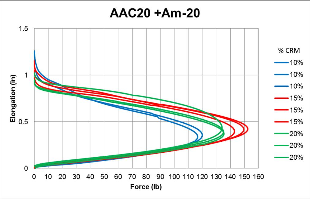
**Figure A-55 Force vs Elongation for AAC20 mixed with Ambient #20**
