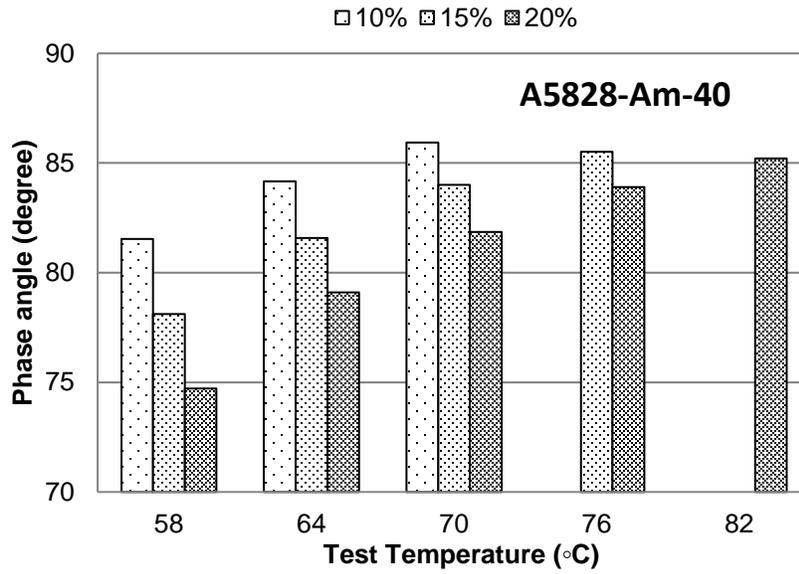
Figure A-16 Phase angle at different temperatures for A5828 mixed with CRM Ambient
