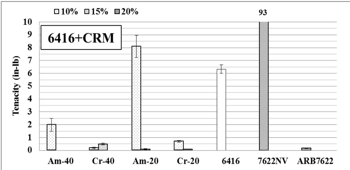
Figure A-61 Tenacity of B6416 samples mixed with CRM, polymer modified and asphalt rubber binder
