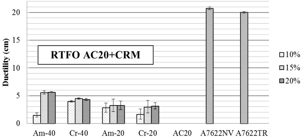
**Figure A-99 Ductility of RTFO AAC20 mixed with CRM, polymer modified and terminal blend tire rubber PG76-22**
