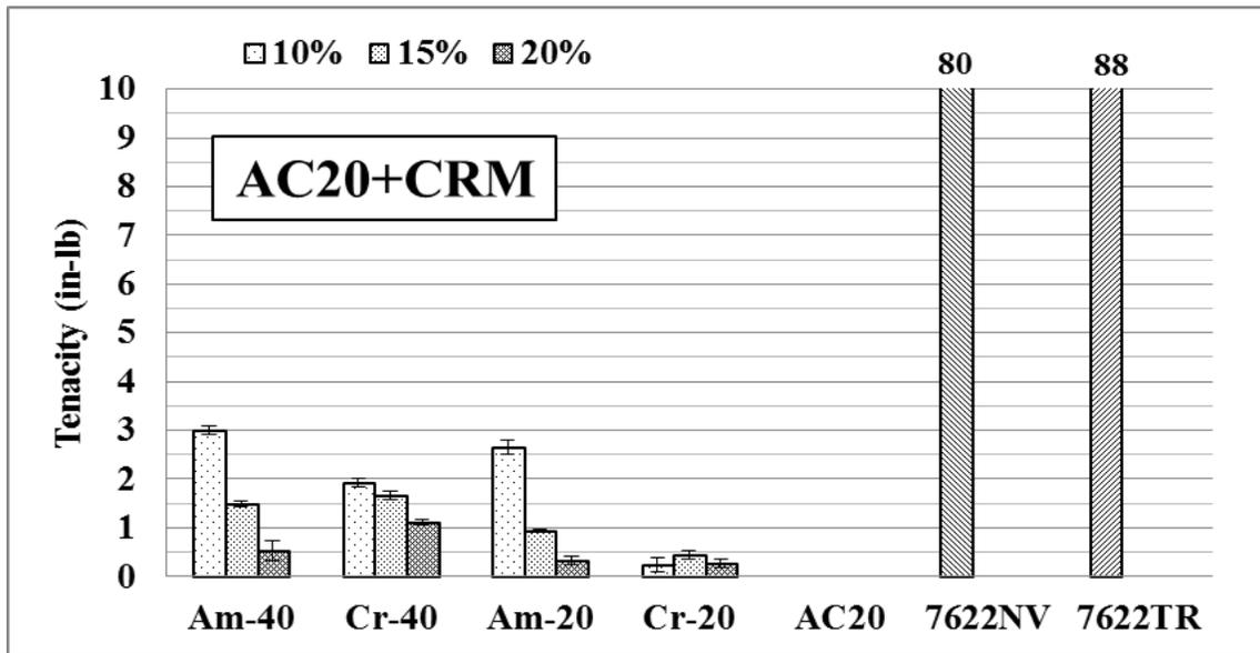
Figure A-62 Tenacity of AAC20 samples mixed with CRM, polymer modified and terminal blend
