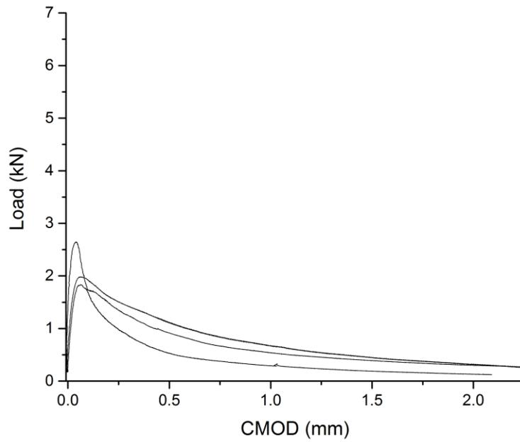
**Figure B-13 The load curves of A6416-AM-20-15 mixtures under SCB test**
