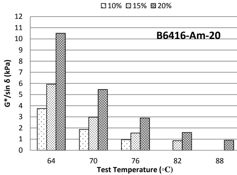
**Figure A-7  $G^*/\sin(\delta)$  at different temperatures for B6416 mixed with CRM Ambient #20**
