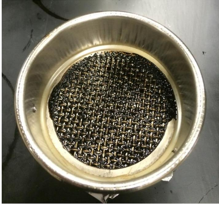
**Figure A-66** Few amount of particles retained on sieve for A5828-Cr-40-10
