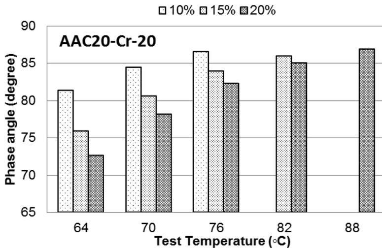
**Figure A-27 Phase angle at different temperatures for B6416 mixed with CRM Cryogenic #20**
