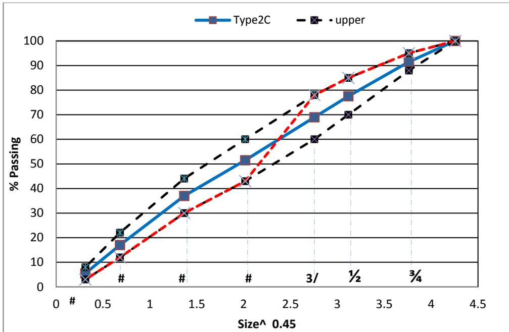
**Figure 5.2 proposed gradation compared to Type 2C mid-point**
