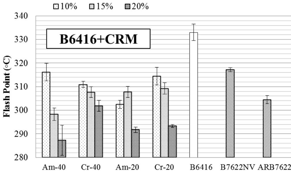
Figure A-35 Flash Point of B6416 samples mixed with CRM, polymer modified and asphalt rubber binder
