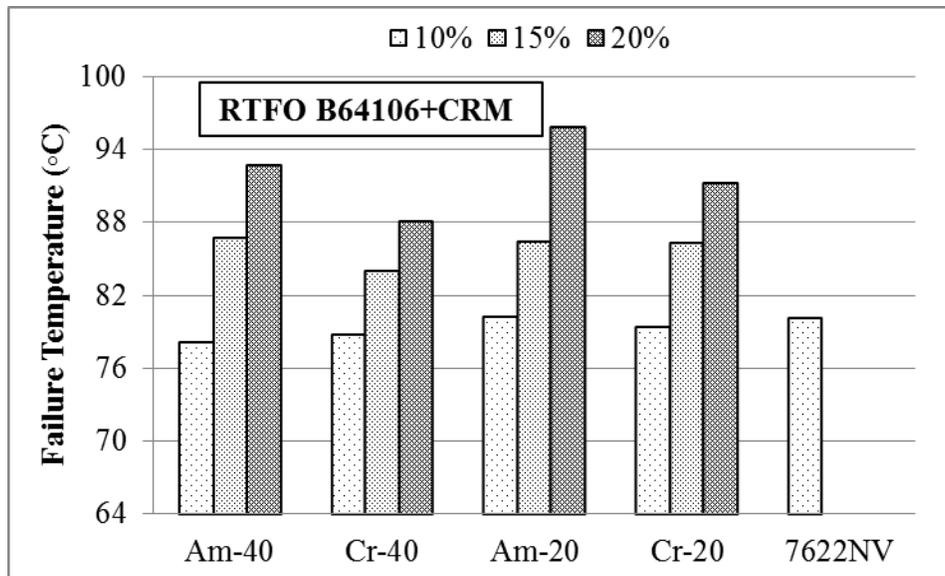
**Figure A-91 Failure temperature for RTFO B6416 and mixed with CRM, and polymer modified 7622**
