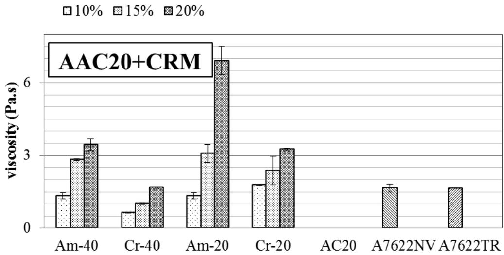
**Figure A-30 Viscosity of B6416 mixed with CRM, polymer and terminally blend tire rubber**
