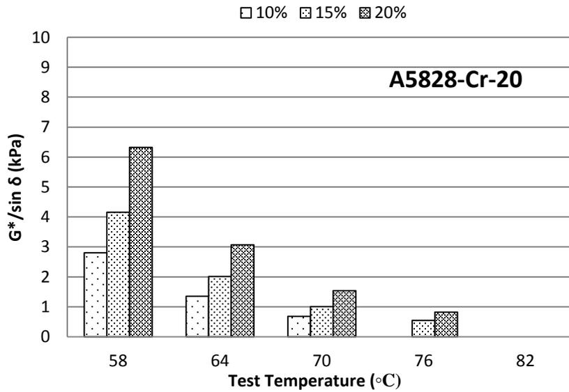
**Figure A-4  $G^*/\sin(\delta)$  at different temperatures for A5828 mixed with CRM Cryogenic #20**
