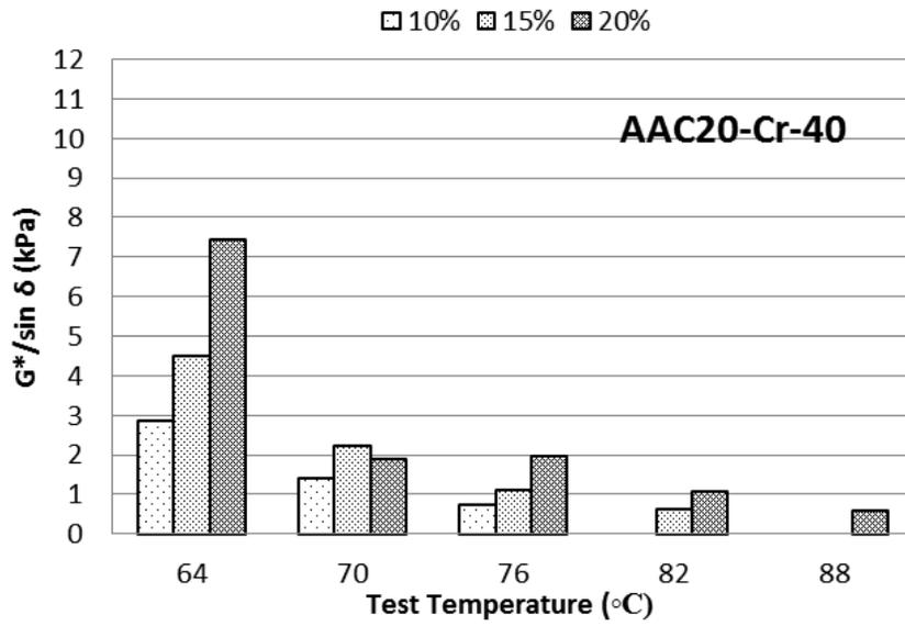
Figure A-10  $G^*/\sin(\delta)$  at different temperatures for AAC20 mixed with CRM Cryogenic #40
