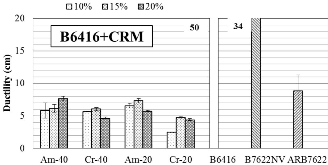
Figure A-32 Ductility of B6416 mixed with CRM, polymer modified and asphalt rubber binder
