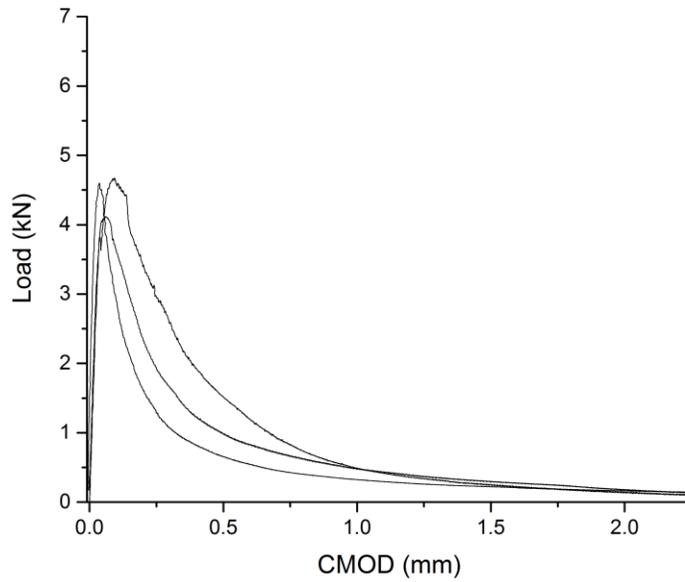
**Figure B-11 The load curves of A7622TR mixtures under SCB test**
