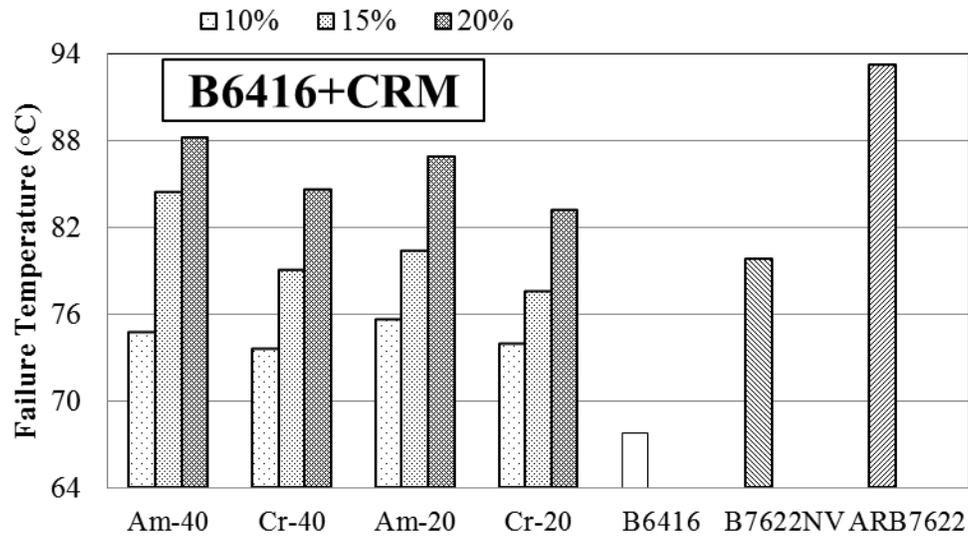
**Figure A-14 Failure temperature for B6416 and mixed with CRM polymer, and asphalt rubber binder**
