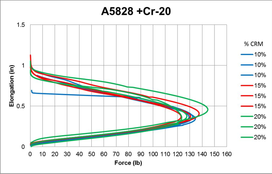
**Figure A-56 Force vs Elongation for AAC20 mixed with Cryogenic #40**
