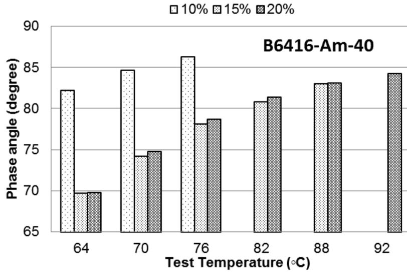
**Figure A-20 Phase angle at different temperatures for B6416 mixed with CRM Ambient #40**
