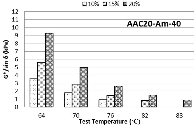
Figure A-9  $G^*/\sin(\delta)$  at different temperatures for AAC20 mixed with CRM Ambient #40
