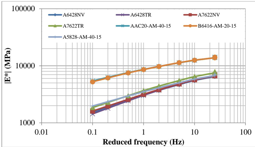
Figure B-20 Dynamic modulus values of various mixtures at 20° C
