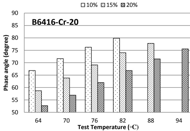
**Figure A-96 Phase angle at different temperatures for RTFO B6416 mixed with CRM Cryogenic #20**
