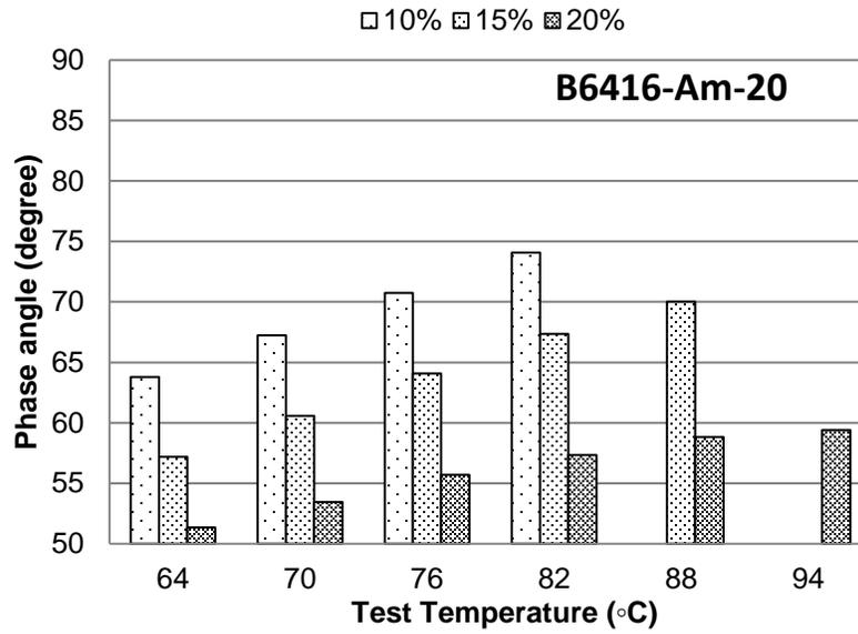
**Figure A-95 Phase angle at different temperatures for RTFO B6416 mixed with CRM Ambient #20**
