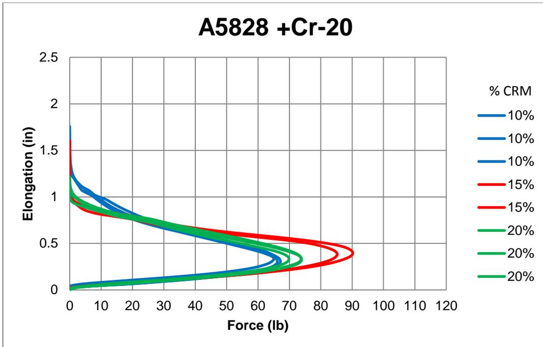
**Figure A-43 Force vs Elongation for A5828 mixed with Cryogenic #40**
