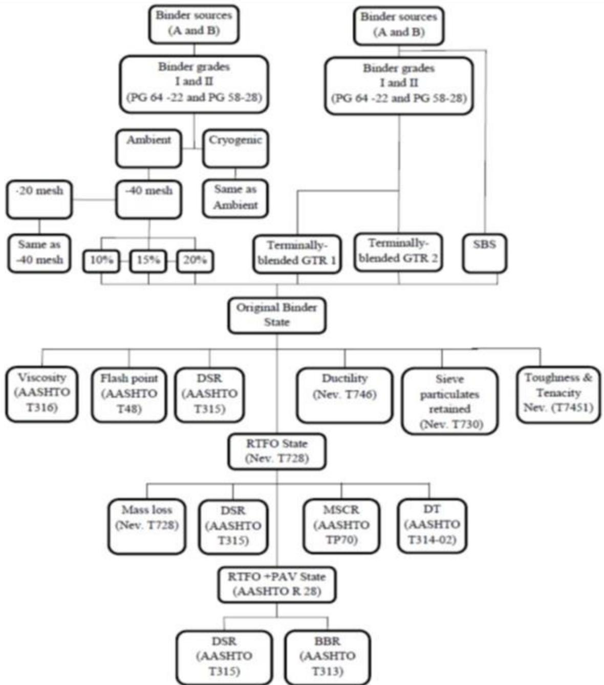
Figure 3.1. Rheological properties of rubberized binders at three aging states
