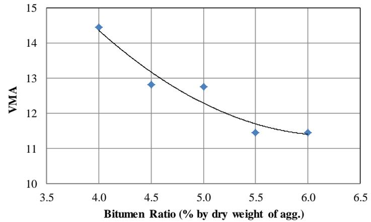
**Figure B-4 Variation of mix design properties with binder content for B64-28NVTR**
