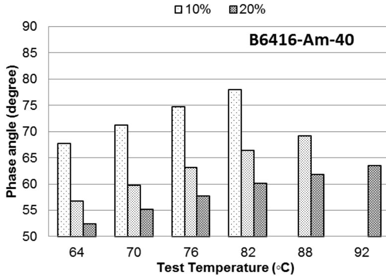
**Figure A-93 Phase angle at different temperatures for RTFO B6416 mixed with CRM Ambient #40**
