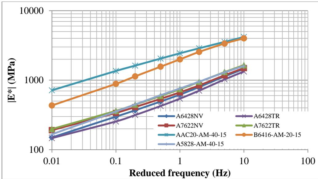
Figure B-22 Dynamic modulus values of various mixtures at 40° C
