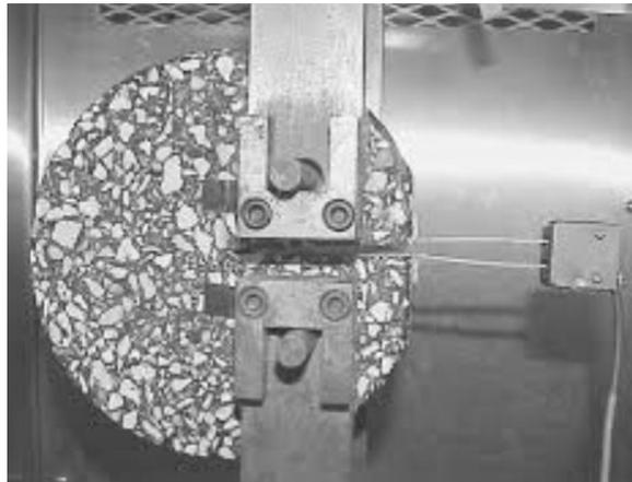
**Figure 5.5. Disk shaped compact tension test**
