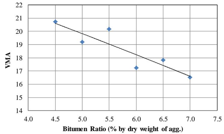
Figure B-5 Variation of mix design properties with binder content for A64-15 + 15%Am#20
