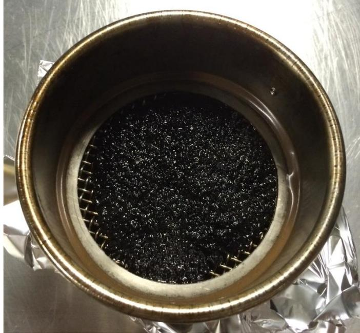
**Figure A-72 particles retained on sieve for AAC20-Am-40-10**
