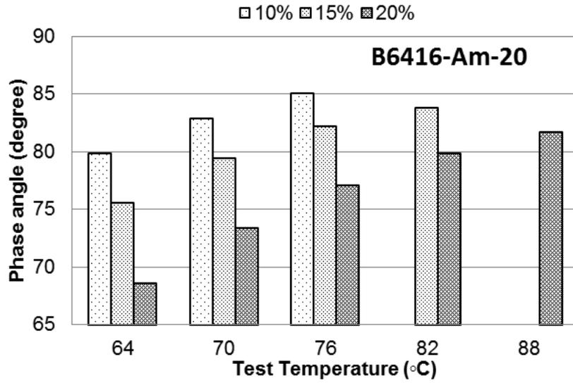
**Figure A-22 Phase angle at different temperatures for B6416 mixed with CRM Ambient #20**
