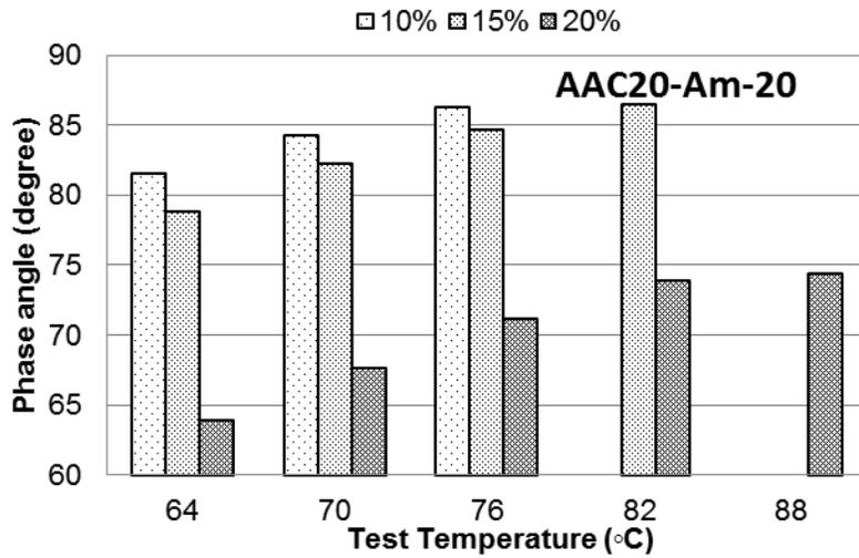
**Figure A-26 Phase angle at different temperatures for AAC20 mixed with CRM Ambient #20**
