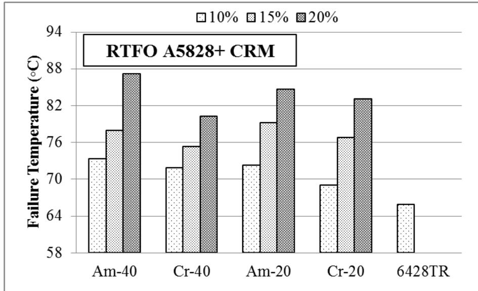
**Figure A-90 Failure temperature for RTFO A5828 and mixed with CRM, and terminal blend tire rubber**
