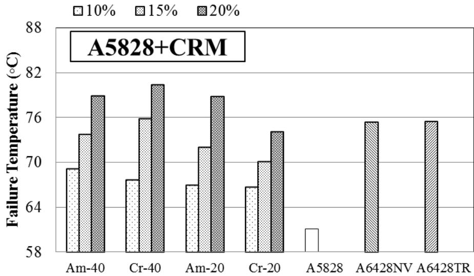
Figure A-13 Failure temperature for A5828 and mixed with CRM, polymer, and terminal blend tire rubber
