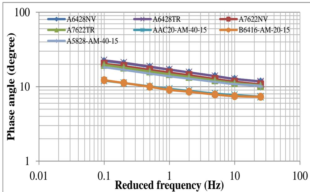
Figure B-19 Phase angle values of various mixtures at 4° C
