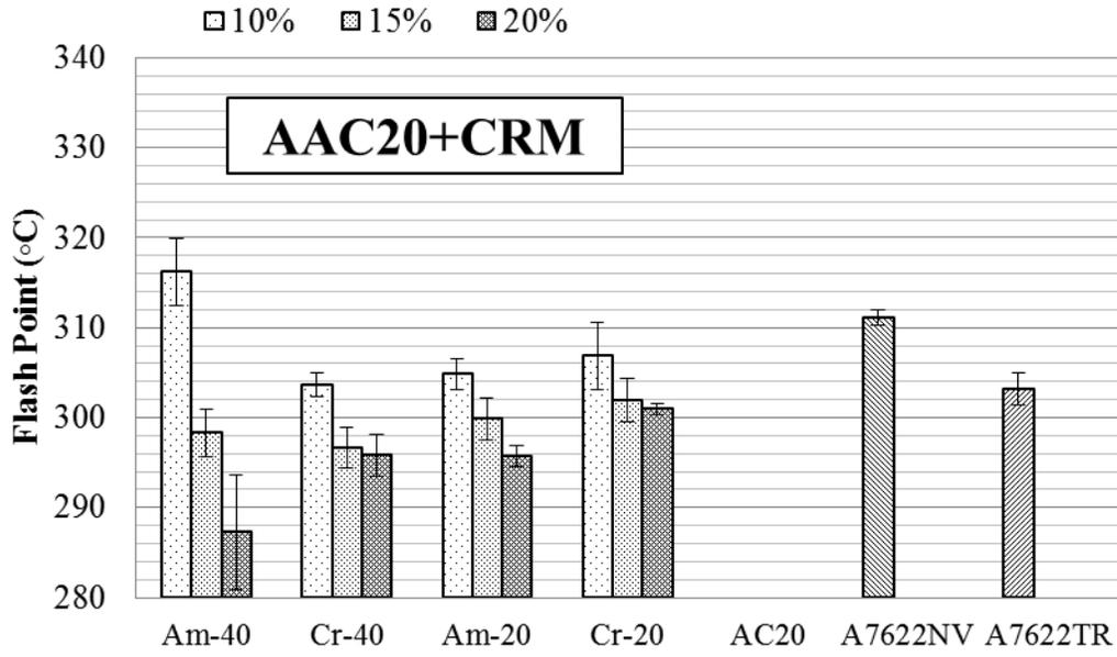
**Figure A-36 Flash Point of AAC20 samples mixed with CRM, polymer modified and terminal blend**
