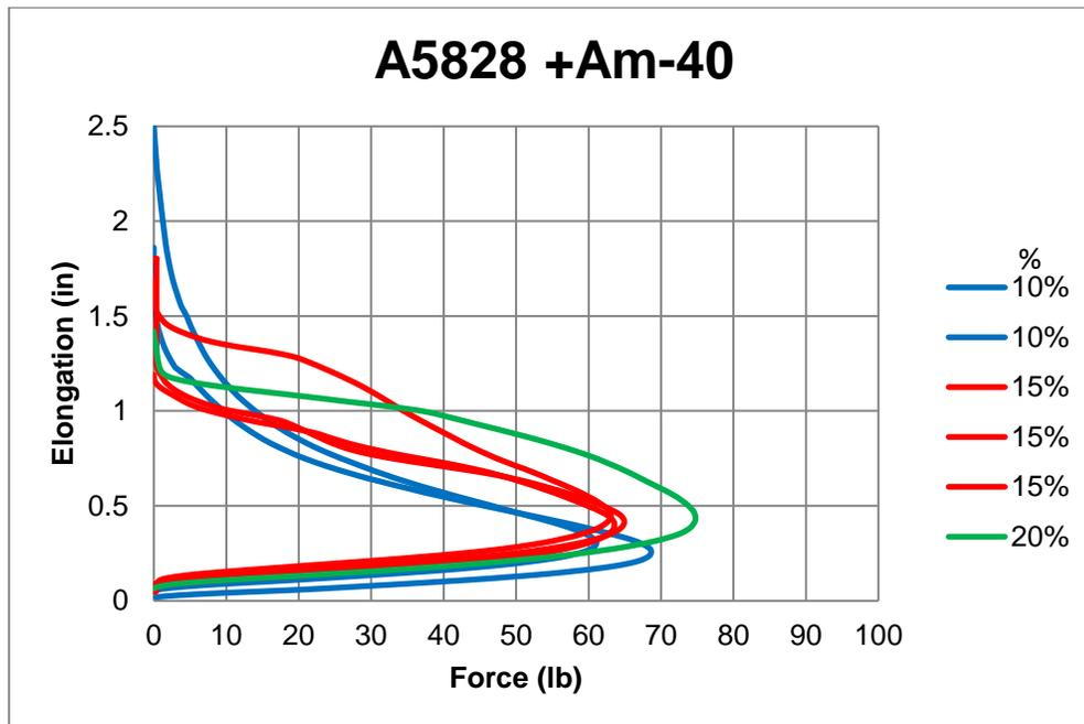
**Figure A-40 Force vs Elongation for A5828 mixed with Ambient #40**
