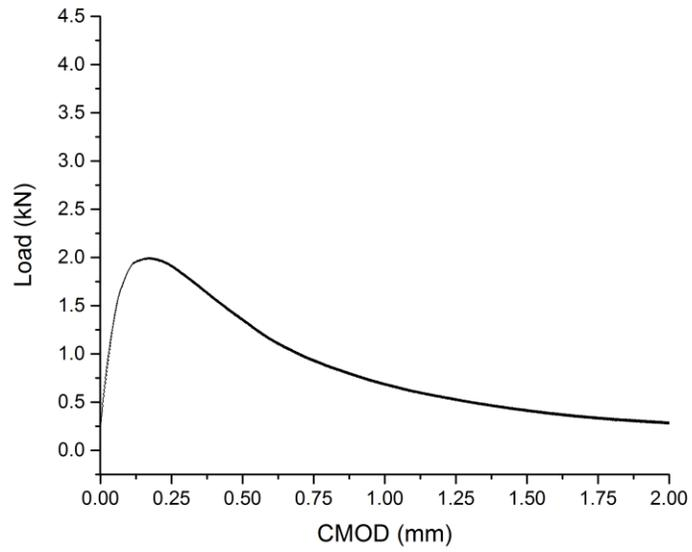
**Figure B-30 The load curves of A6416-AM-20-15 mixtures under DCT test**
