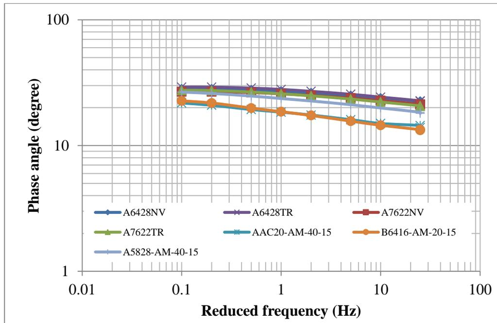
Figure B-21 Phase angle values of various mixtures at 20° C
