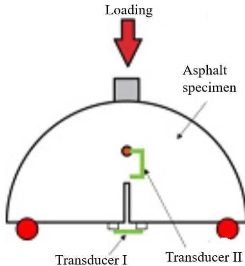
**Figure 5.3. SCB test scheme**
