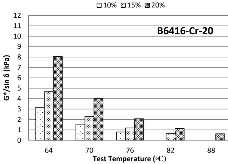
**Figure A-8  $G^*/\sin(\delta)$  at different temperatures for B6416 mixed with CRM Cryogenic #20**
