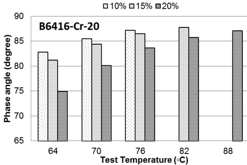
**Figure A-23 Phase angle at different temperatures for B6416 mixed with CRM Cryogenic #20**
