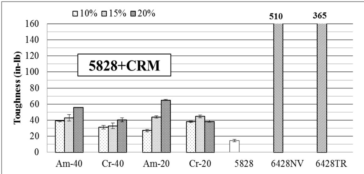
Figure A-57 Toughness of A5828 samples mixed with CRM, polymer modified and terminal blend
