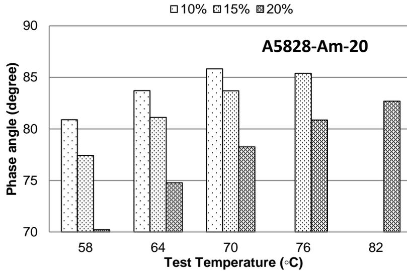
**Figure A-18 Phase angle at different temperatures for A5828 mixed with CRM Ambient #20**
