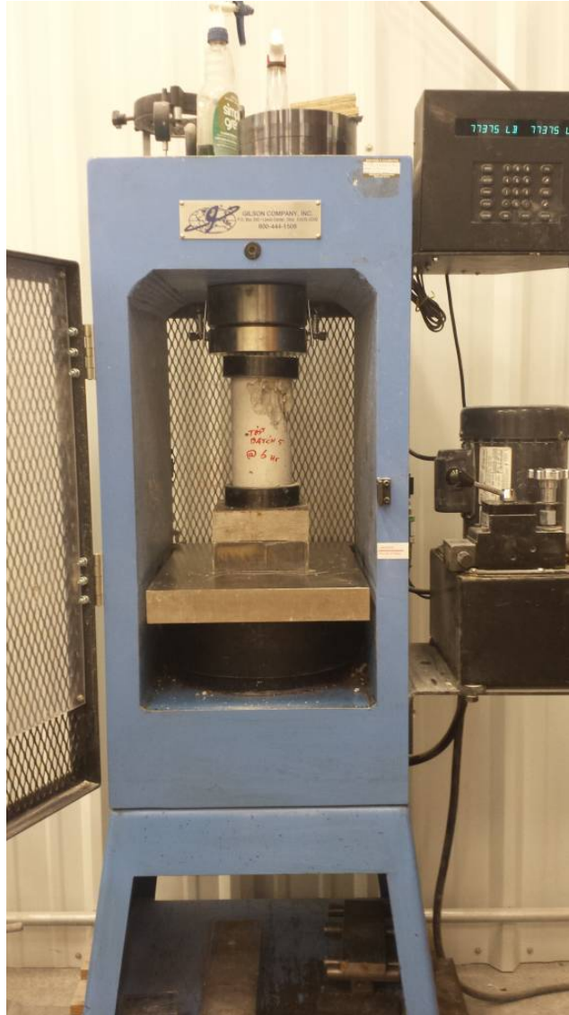
Figure 2-7: Compression Loading Machine
