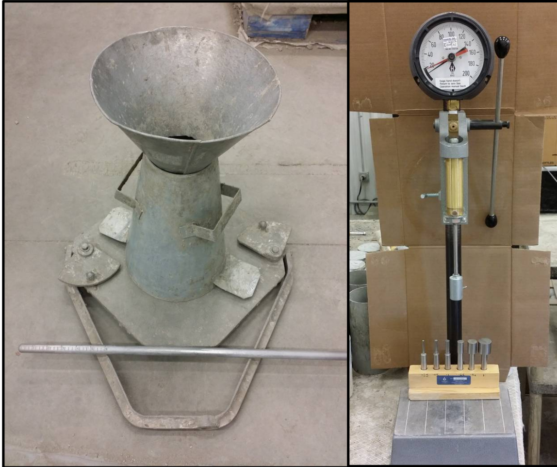
Figure 2-4: (Left) Abrams Slump Cone; (Right) Acme Penetrometer
