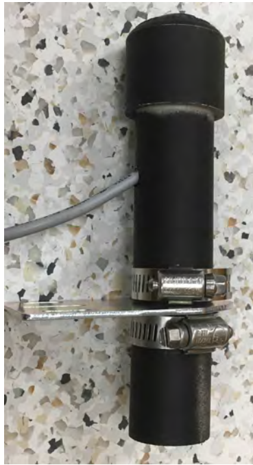
Figure 3.8: The CT1-00-2H capacitive proximity sensor inside its brine protective housing.
