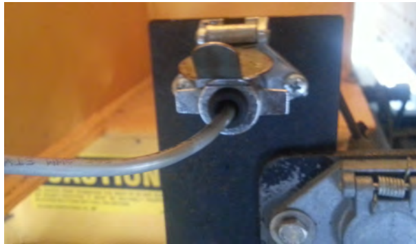
Figure 3.5: A four-pole trailer connector was included in the installation to allow for easy detachment and reattachment of the spreader conveyor motor wiring from the plow truck.
