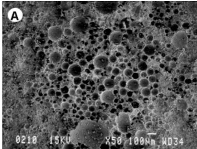
Figure 2-3. SEM micrograph showing air void clustering at aggregate-HCP interface (Cross et al. 2000).
