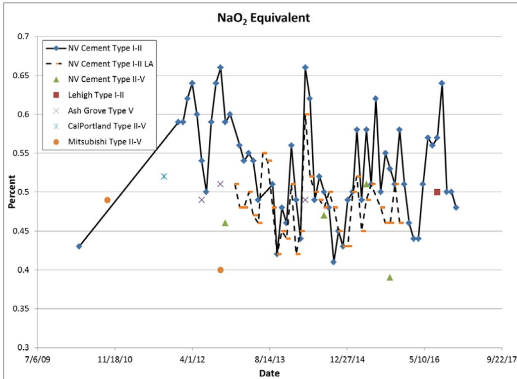
Figure 4-2. Plot of alkali content (in sodium equivalents) for all mill certificates.
