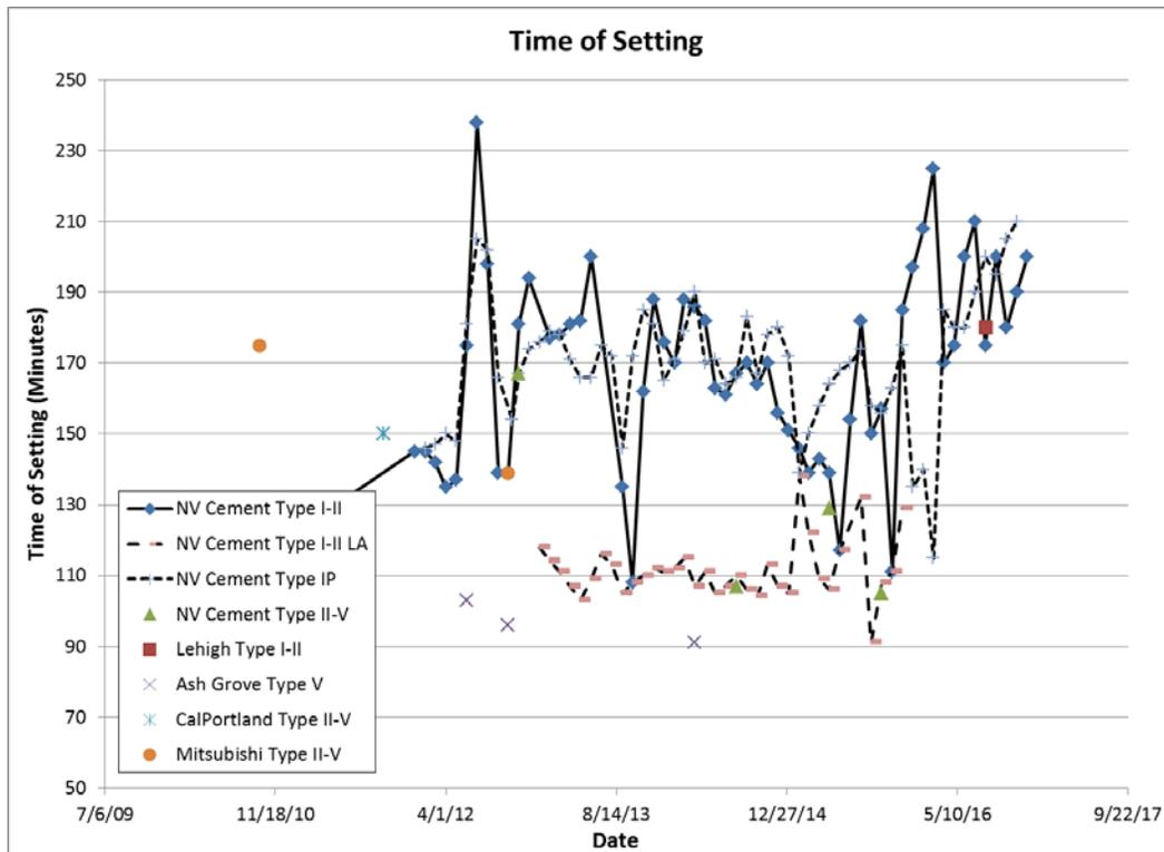
Figure 4-4. Plot of setting time (minutes) for all mill certificates.
