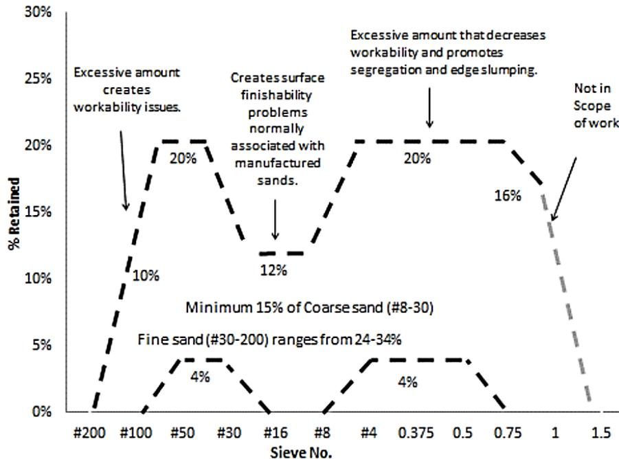
Figure 3-2. Tarantula curve with proposed limits for fine and coarse sand (Cook, Ghaeezadah, and Ley 2013a).
