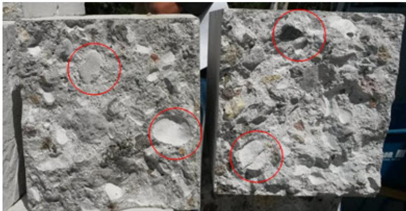
Figure 1-1. Fracture surface in concrete beams tested in flexure. Note multiple aggregate "pull-outs", some circled in red (Van Dam 2015).
