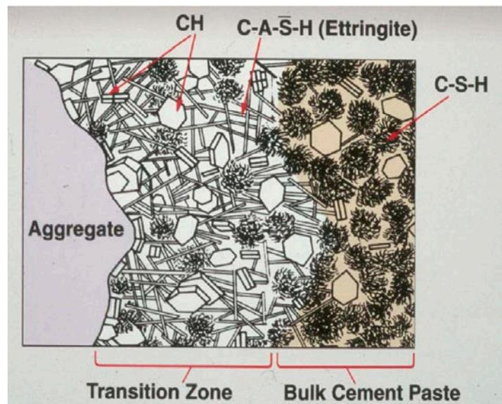
Figure 2-1. Schematic representation of the interfacial transition zone between an aggregate particle and the bulk cement paste. (after Mehta and Monteiro 2006).
