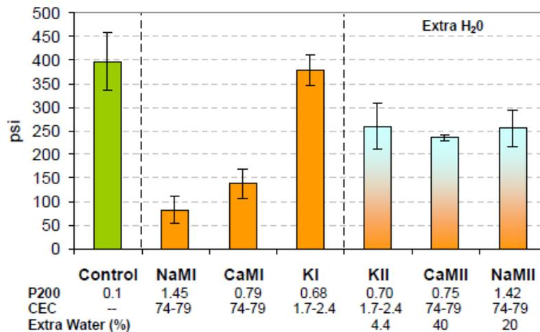
Figure 2-6. Effect of additional mix water on tensile strength of concrete made with aggregates with clay coatings (Muñoz et al. 2007).
