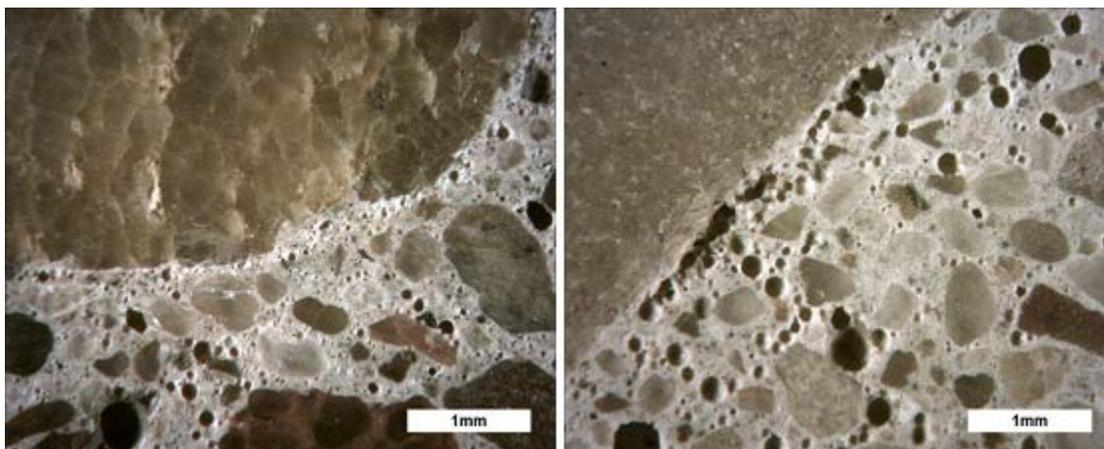
Figure 2-4. Stereo optical micrograph showing air void clustering along coarse aggregate-HCP interface (Ram et al. 2013).
