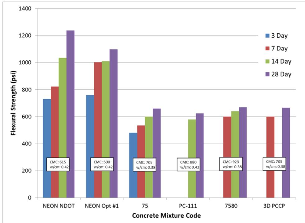
Figure 4-1. Comparison of flexural strength with time for Project NEON trial batch compared to four Northern Nevada NDOT mixtures. Note “CMC” stands for total cementitious materials content in lbs/yd<sup>3</sup>.
