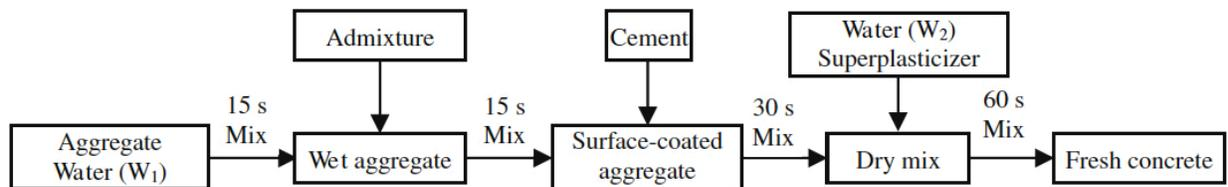
Figure 2-2. Schematic presentation of the triple mixing procedure used by Kong et al. (2010).
