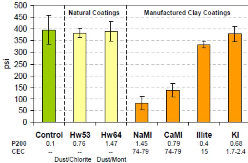
Figure 2-5. Tensile strength for concrete made with aggregates with clay coatings. Note that the yellow bars represent natural clay coating whereas the orange bars represent aggregates coated in the laboratory (Muñoz et al. 2007).
