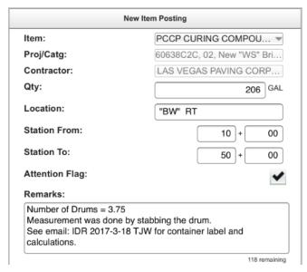
Figure 12-2: IDR Item Posting - Concrete Paving GAL
