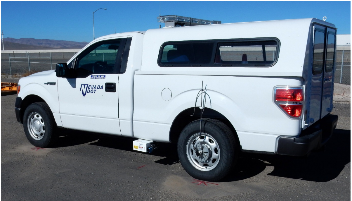
Figure 17: High-speed inertial profiler
