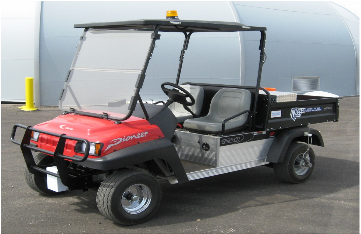
Figure 16: Lightweight inertial profiler
