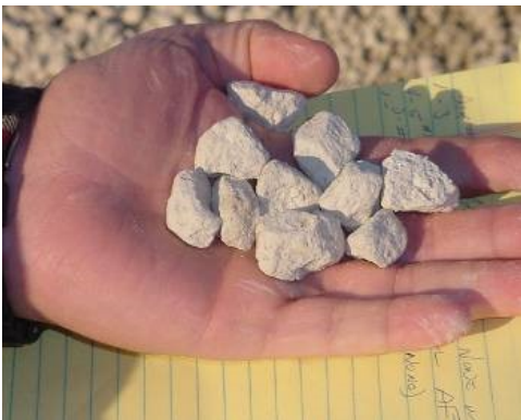
Figure 8: Marinated aggregate uniformly coated with lime
