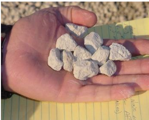
Figure 8: Marinated aggregate uniformly coated with lime
