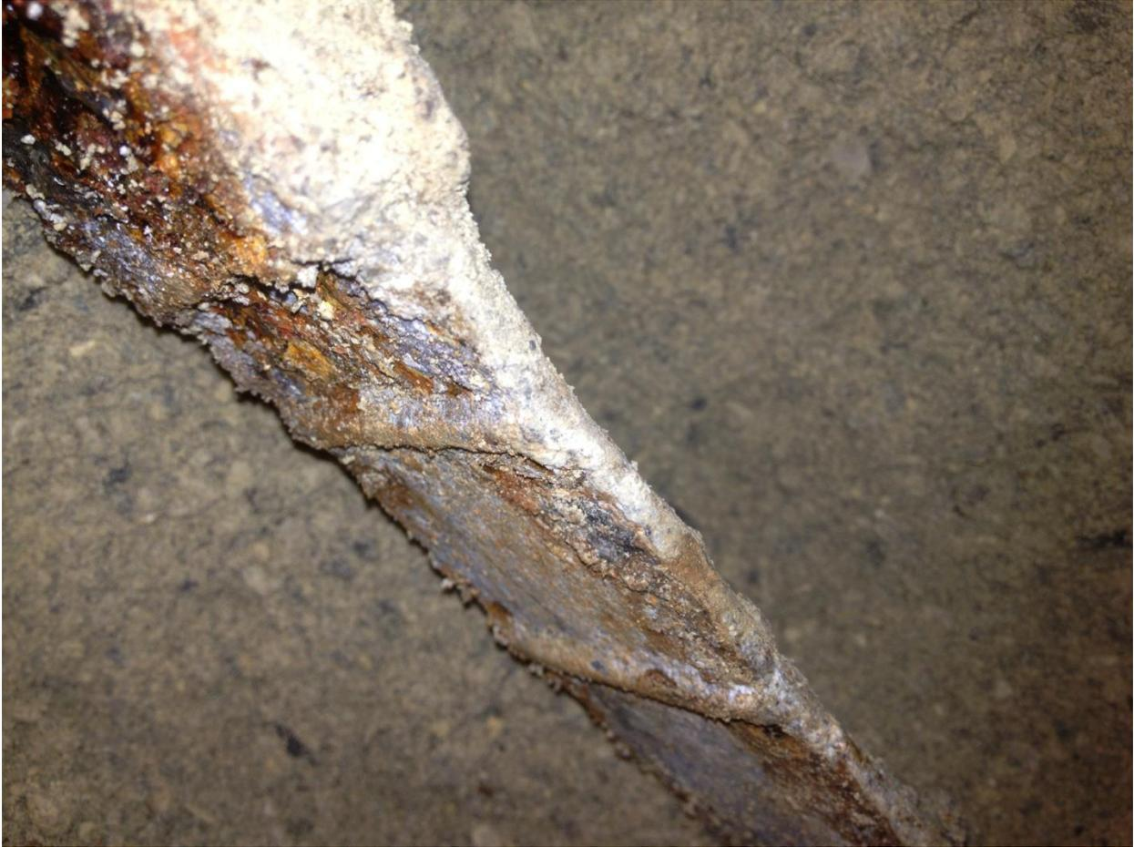
**Figure 5-16:** In-service galvanized soil reinforcement for I-15/ Cheyenne Blvd. Wall 1, 15 years old.
