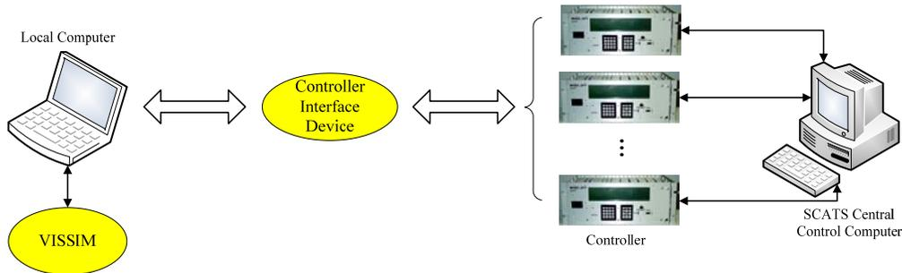
Figure 2.1-1 Hardware-in-the-loop Simulation Environment
