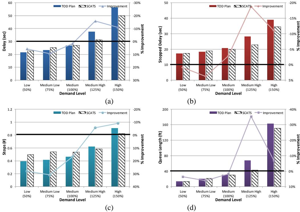
Figure 2.3-13 SCATS Performance for Node Level MOEs – One Direction Detector Failures
