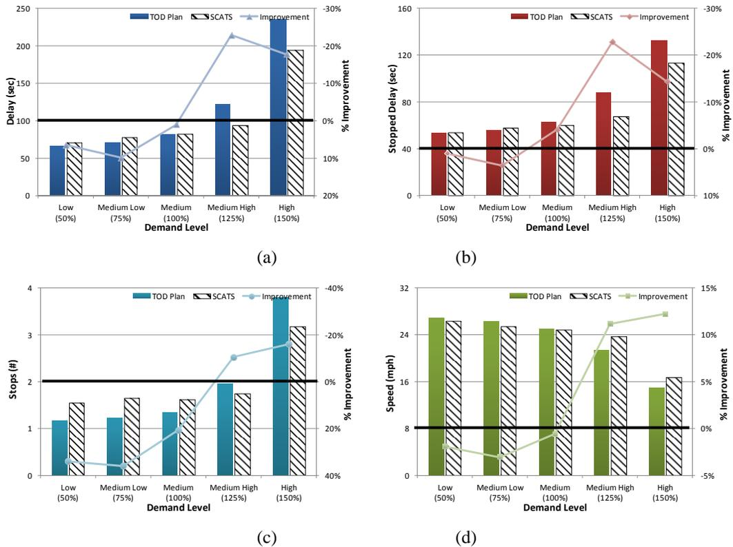
Figure 2.3-12 SCATS Performance for Network Level MOEs – One Direction Detector Failures
