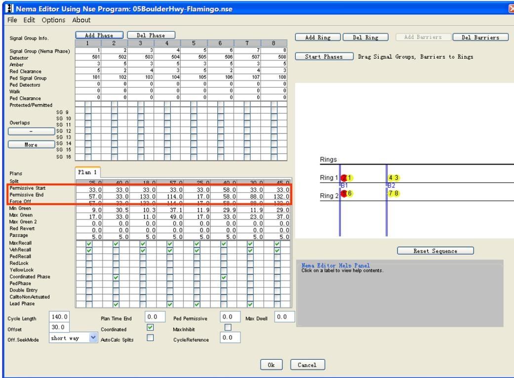
Figure 2.1-7 Signal Timing Parameters in VISSIM
