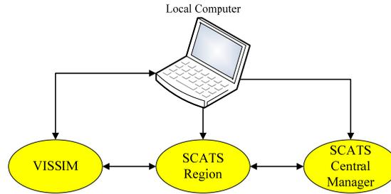
Figure 2.1-2 Software-in-the-loop Simulation Environment
