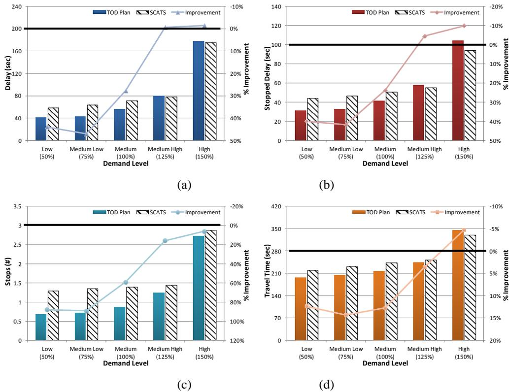
Figure 2.3-17 SCATS Performance for Route Level MOEs – Main Street Detector Failures
