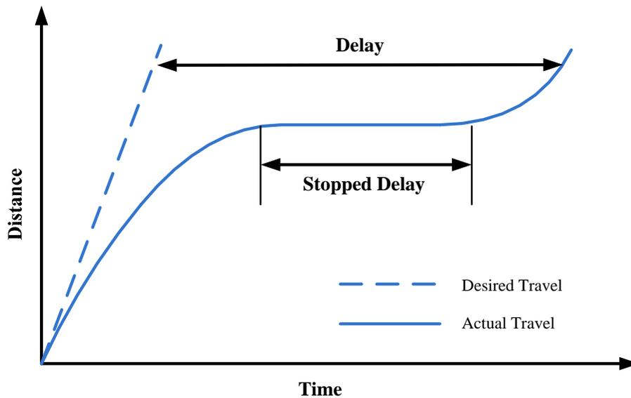
Figure 3.1-2 Illustration of Delay and Stopped Delay
