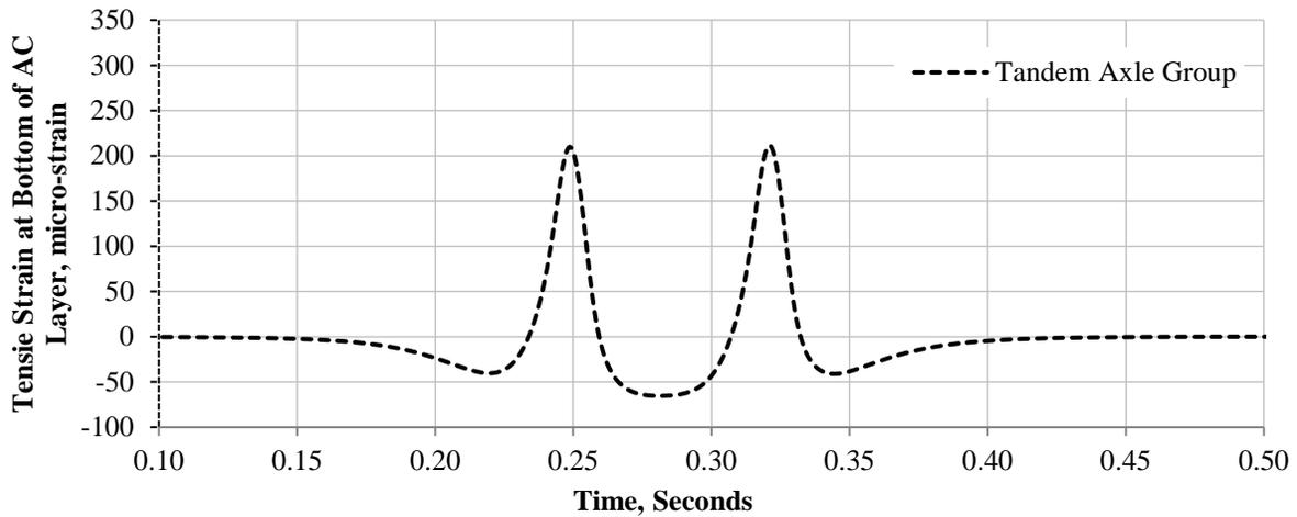
**Figure 2.4. Graph. Tensile strain response history at the bottom of AC layer for axle groups C, D, E, F, and G (tandem axle).**
