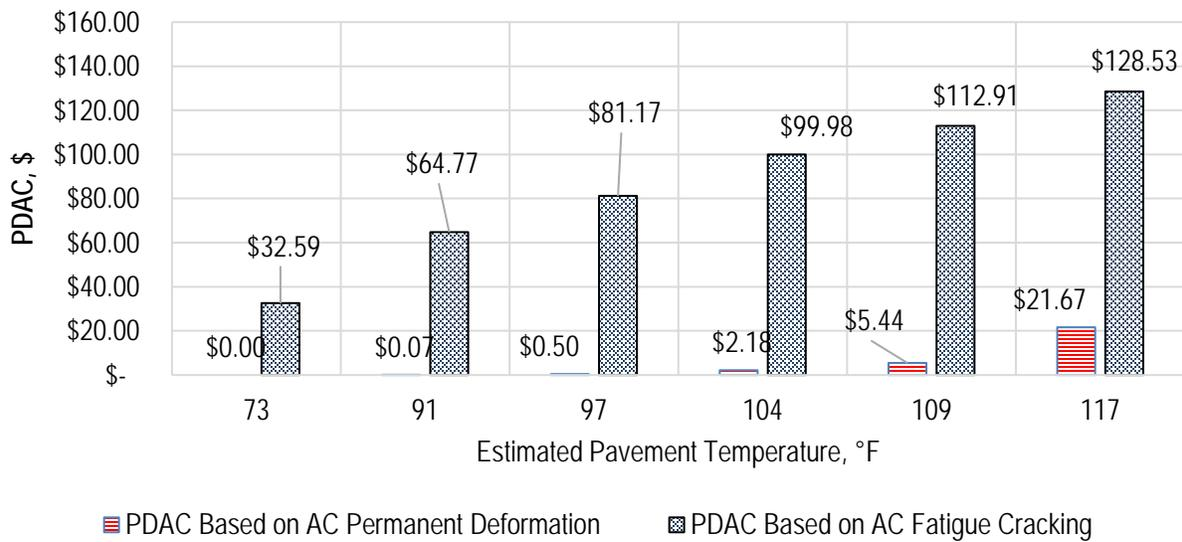
**Figure 7.10. OW vehicle PDAC values in US dollars per trip for Case study II (SR 146 Section).**
