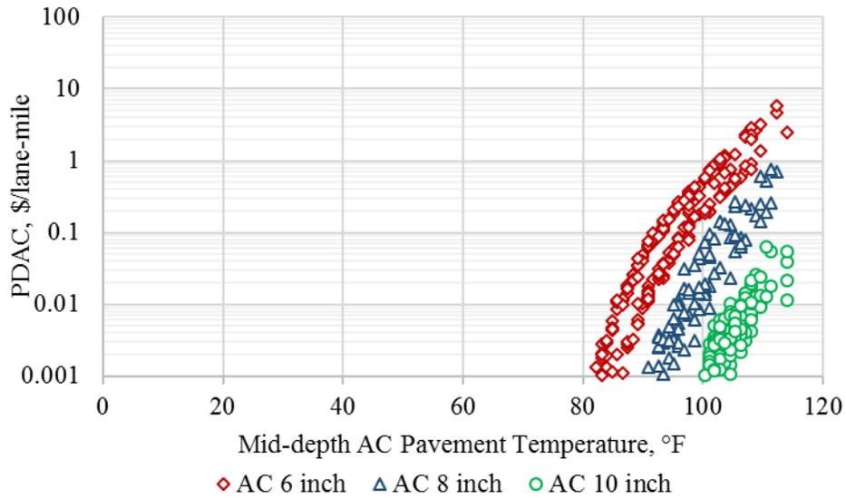
**Figure B.10. AC permanent deformation based PDAC output from Monte-Carlo simulations for Mercury weather station.**
