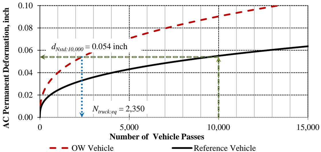
**Figure 2.11. Equivalent number of OW vehicle passes after 10,000 passes of the reference vehicle.**
