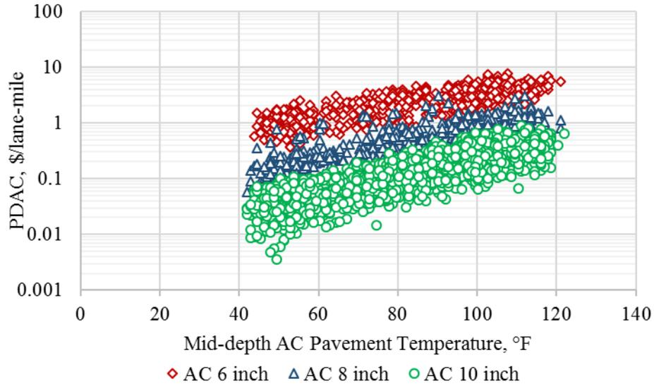
**Figure B.7. Fatigue cracking based PDAC output from Monte-Carlo simulations for Las Vegas weather station.**
