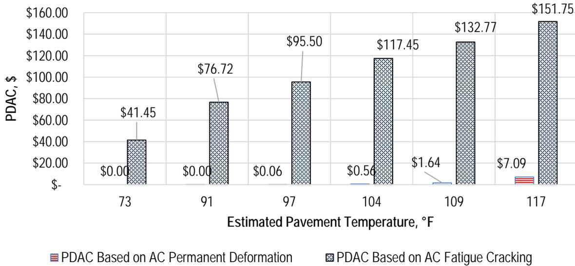
**Figure 7.8. OW vehicle PDAC values in US dollars per trip for Case study II (Interstate 15 Section).**
