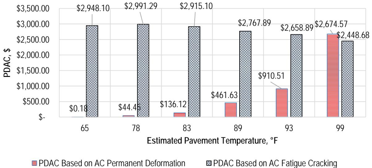
**Figure 7.16. OW vehicle PDAC values in US dollars per trip for Case Study III.**
