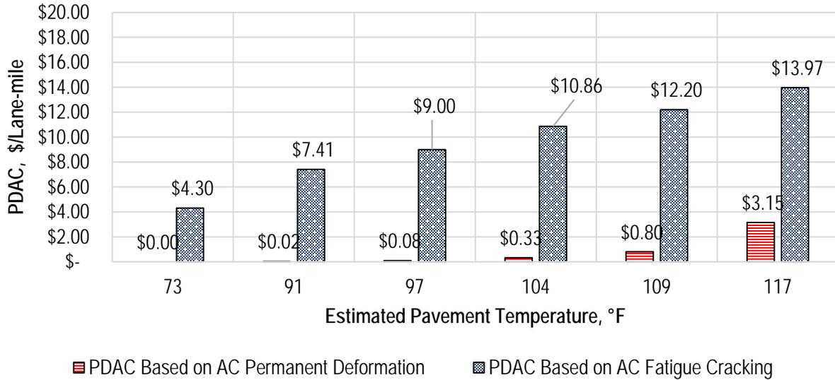
**Figure 7.11. OW vehicle PDAC values in US dollars per lane mile for Case study II (Interstate 215 Section).**
