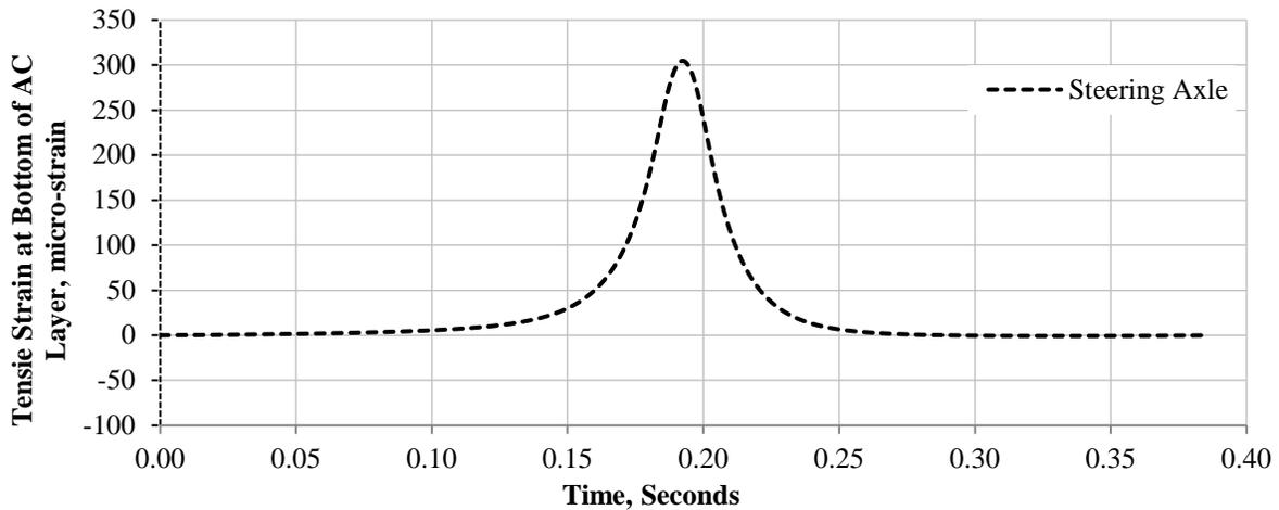
Figure 2.2. Tensile strain response history at the bottom of AC layer for axle group A (single axle).
