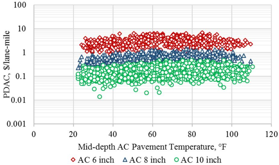
**Figure B.11. Fatigue cracking based PDAC output from Monte-Carlo simulations for Reno weather station.**
