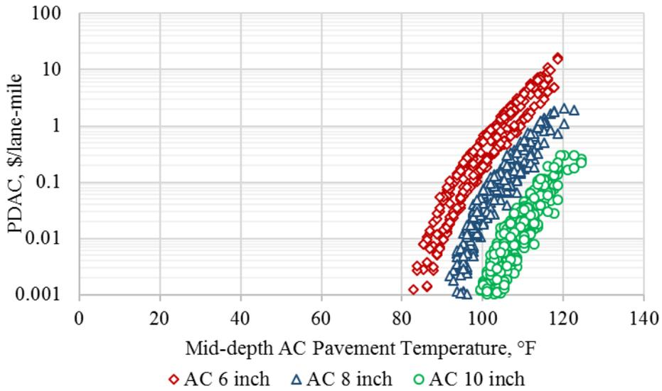
**Figure B.8. AC permanent deformation based PDAC output from Monte-Carlo simulations for Las Vegas weather station.**
