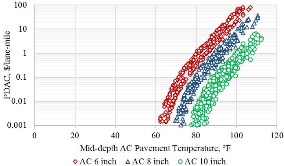
**Figure 5.6. AC permanent deformation based PDAC output from Monte-Carlo simulations for Reno weather station.**
