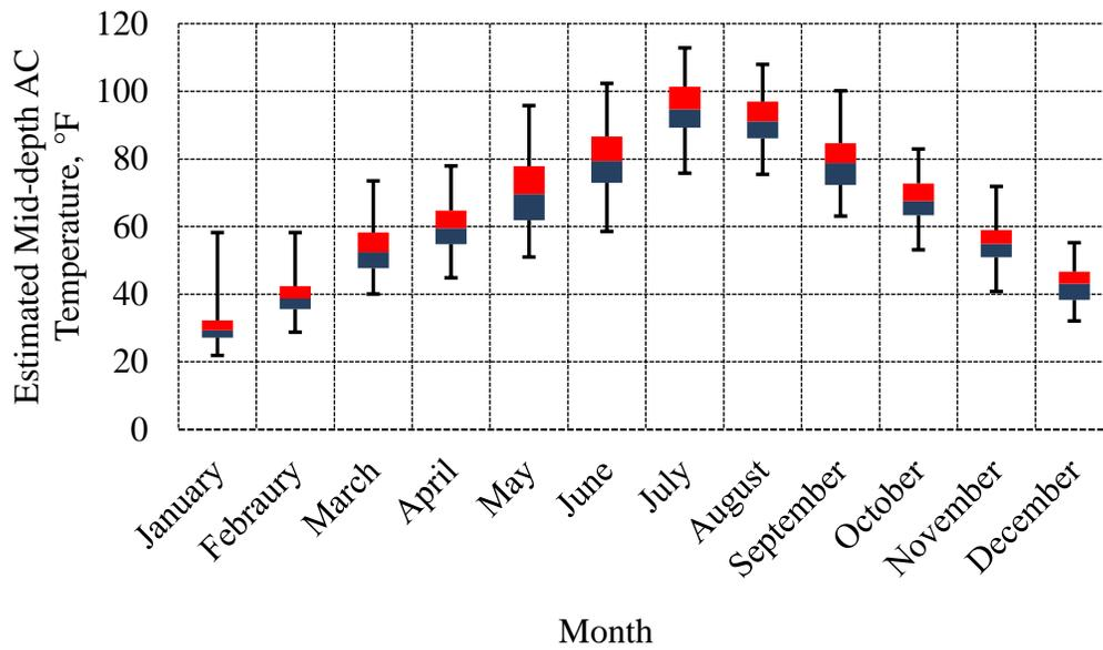
**Figure A. 6: Estimated Mid-depth AC temperature for Reno station.**
