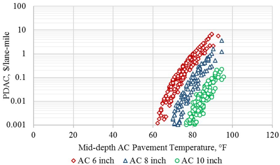
**Figure B.14. AC permanent deformation based PDAC output from Monte-Carlo simulations for South Tahoe weather station.**
