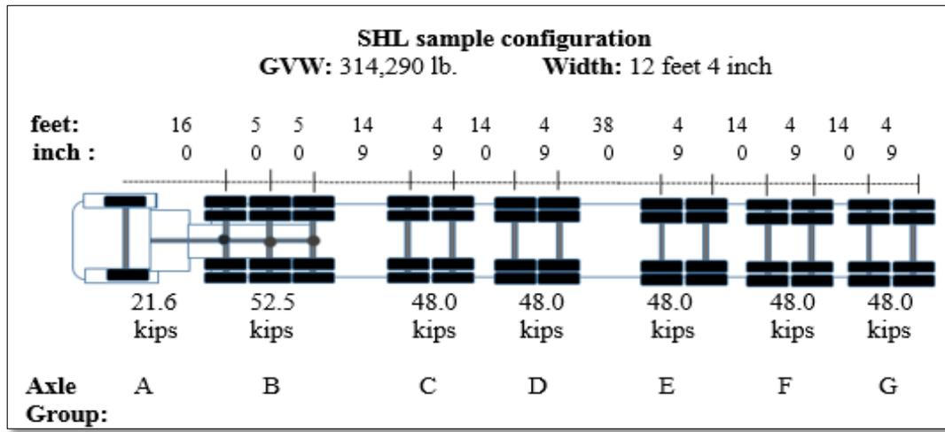
Figure 2.1. Example for an OW vehicle configuration.
