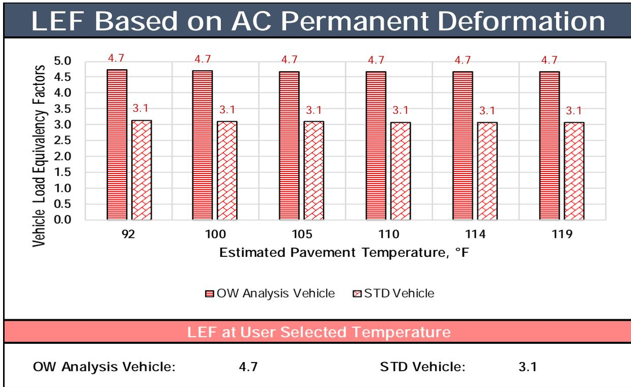
Figure 6.7. AC permanent deformation-based LEFs output result for single trip scenario.
