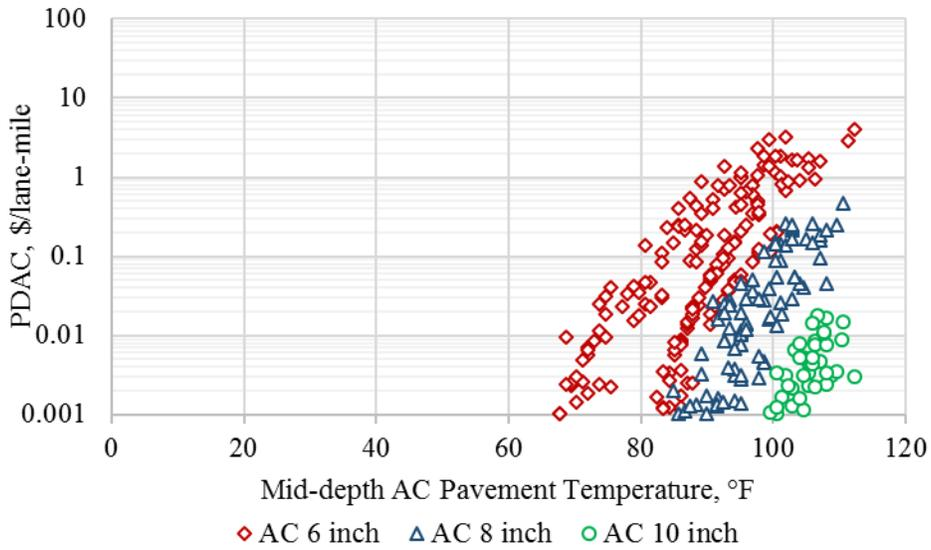
**Figure B.16. AC permanent deformation based PDAC output from Monte-Carlo simulations for Tonopah weather station.**
