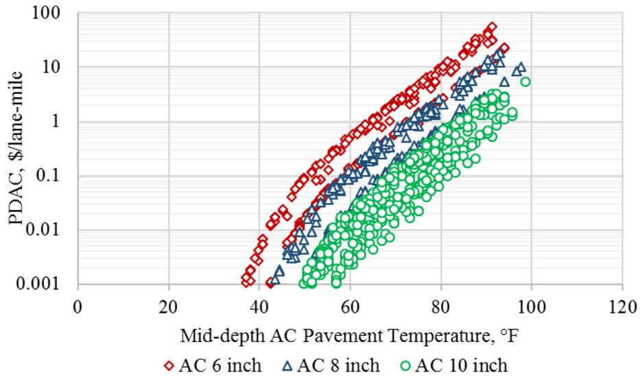
**Figure B.4. AC permanent deformation based PDAC output from Monte-Carlo simulations for Ely weather station.**
