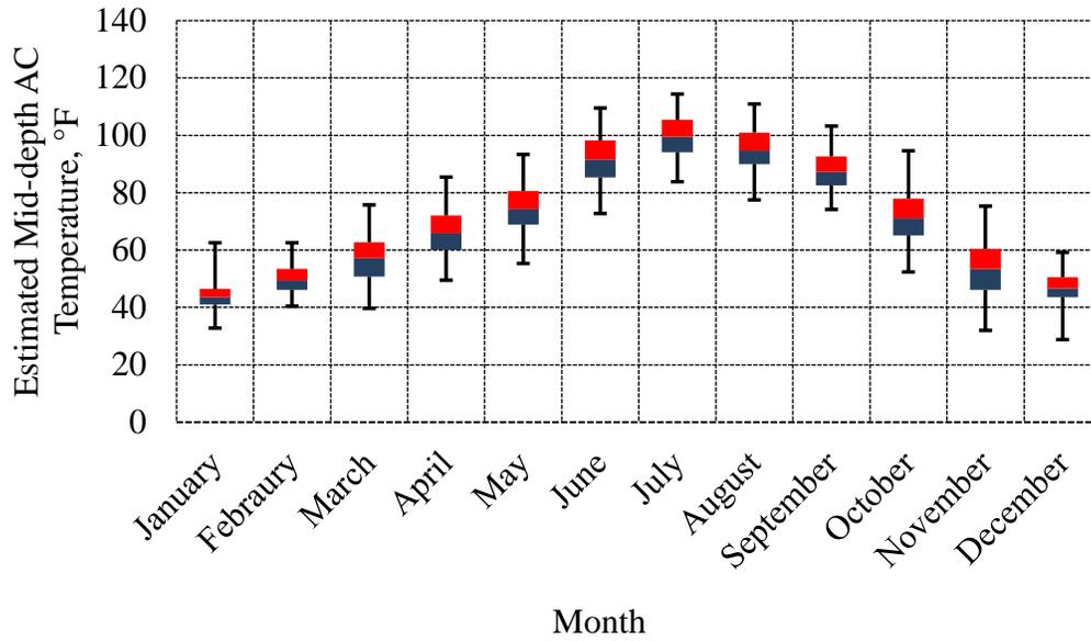
**Figure A. 5: Estimated Mid-depth AC temperature for Mercury station.**
