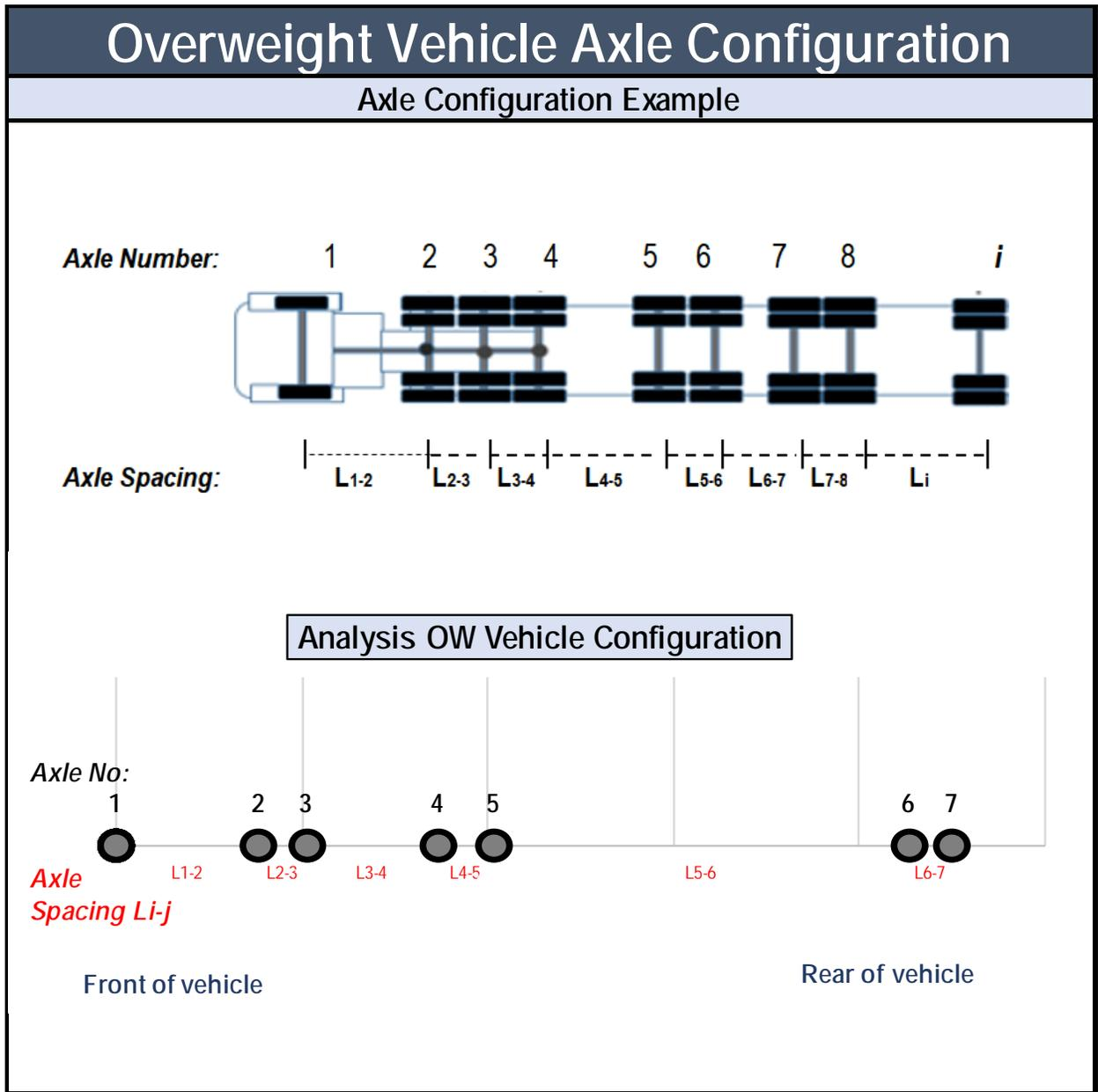
Figure 6.4. Overweight vehicle axle configuration schematic presented in panel No. two.
