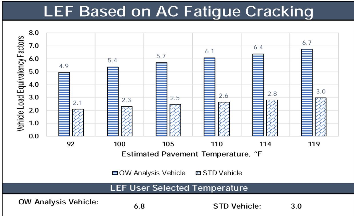
Figure 6.8. AC fatigue cracking-based LEFs output result for single trip scenario.
