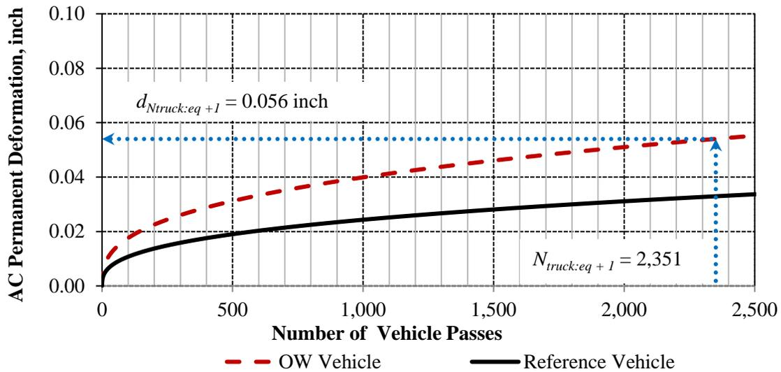
**Figure 2.12. AC permanent deformation after  $N_{truck: eq+1}$ .**
