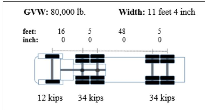
**Figure 2.7. Reference vehicle configuration.**
