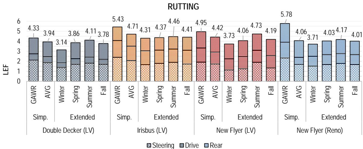
Figure 7.26. LEFs results based on AC permanent deformation.
