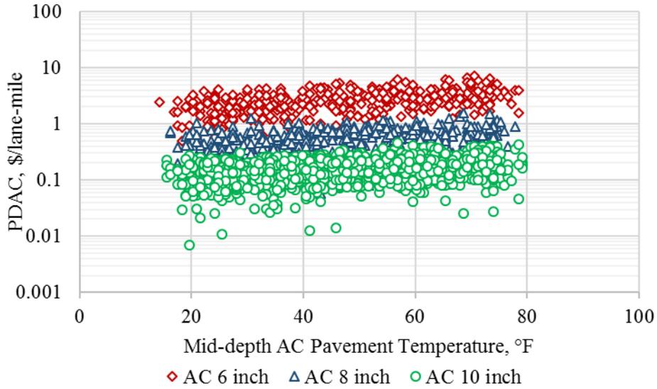
**Figure B.17. Fatigue cracking based PDAC output from Monte-Carlo simulations for Winnemucca weather station.**
