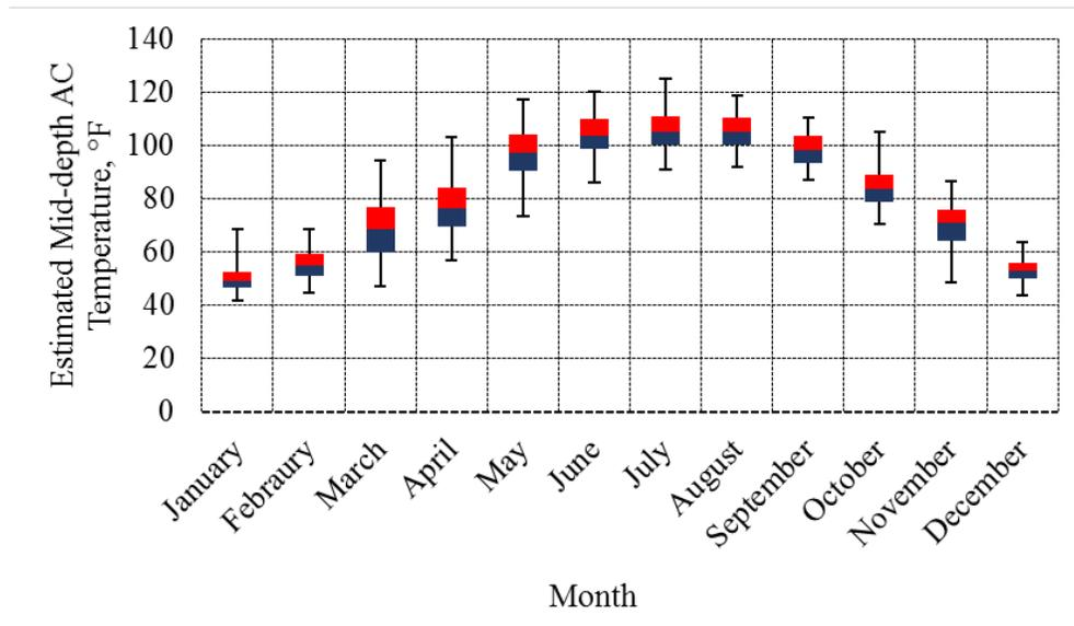
Figure 3.15. Estimated mid-depth AC temperature for Las Vegas.
