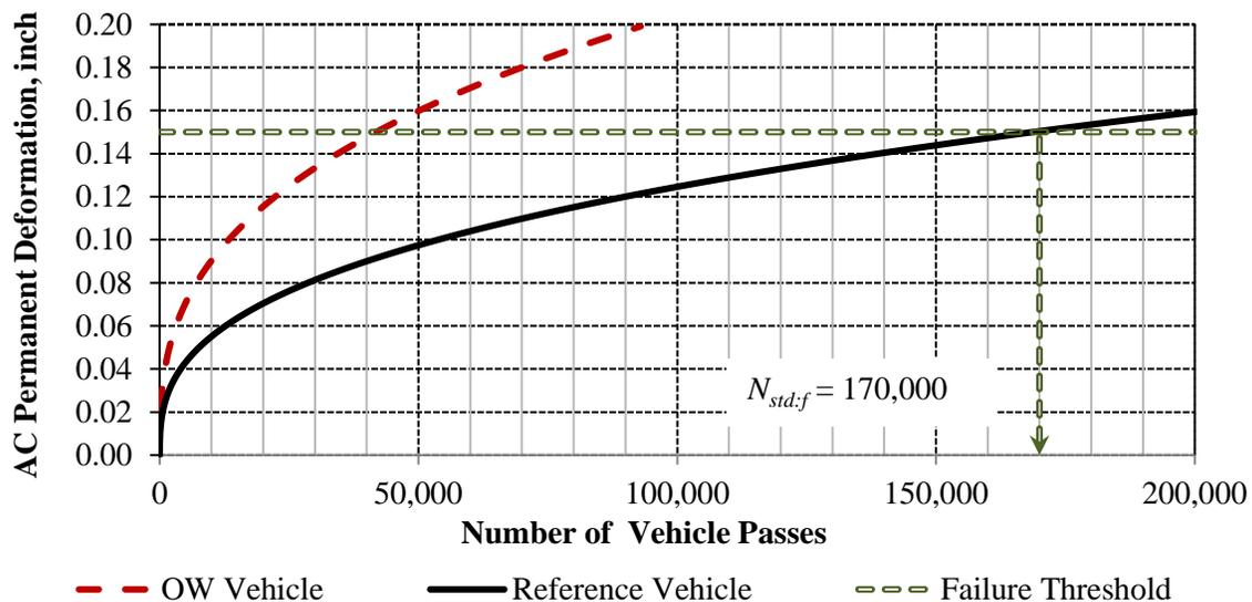
**Figure 2.9. Number of reference vehicle passes to failure.**
