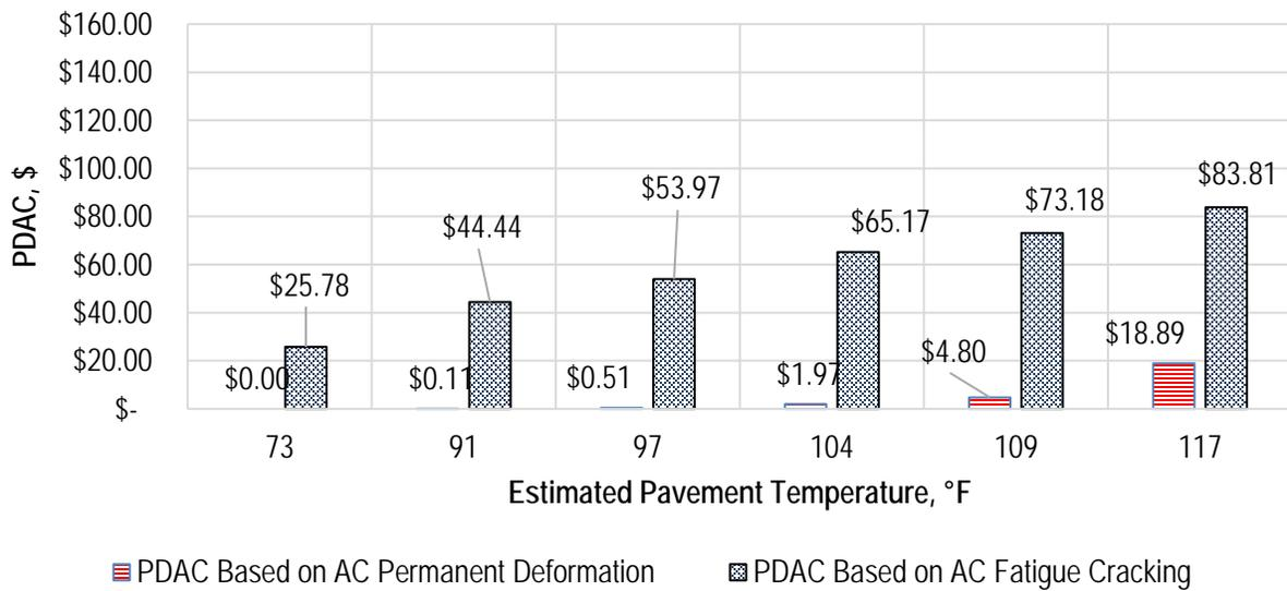
**Figure 7.12. OW vehicle PDAC values in US dollars per trip for Case study II (Interstate 215 Section).**
