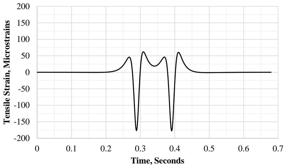
Figure 4.2. Tensile strain history at bottom of AC layer at C location (between adjacent tires).
