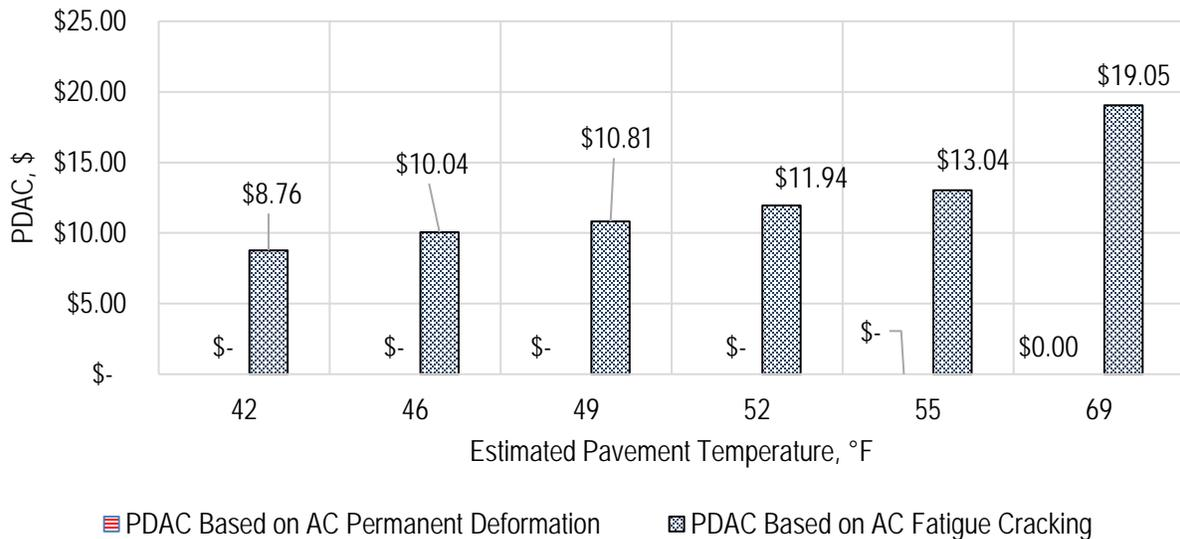
**Figure 7.4. OW vehicle PDAC values in US dollars per trip for Case study I.**
