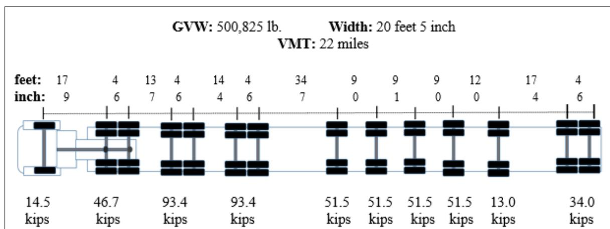
**Figure 2.6. OW vehicle configuration.**
