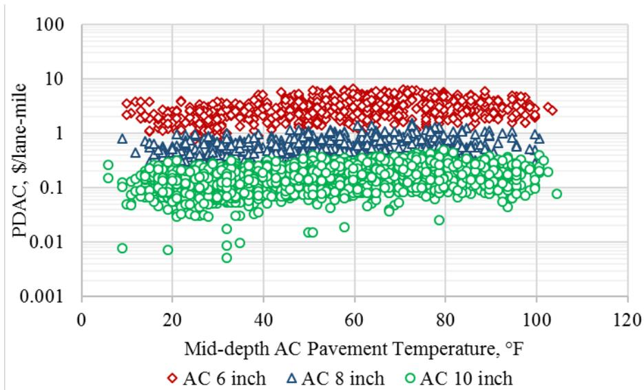
**Figure B.1. Fatigue cracking based PDAC output from Monte-Carlo simulations for Elko weather station.**
