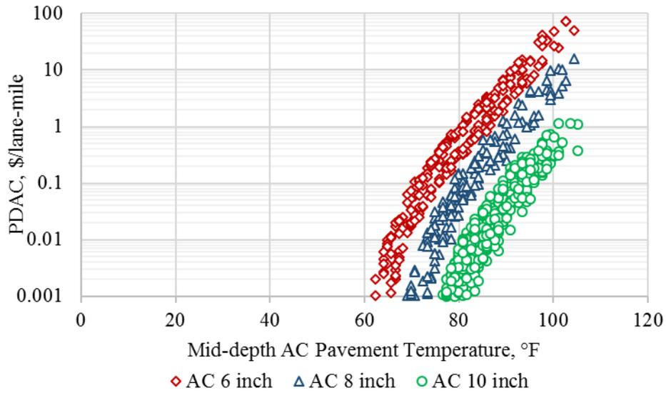
**Figure B.6. AC permanent deformation based PDAC output from Monte-Carlo simulations for Lovelock weather station.**
