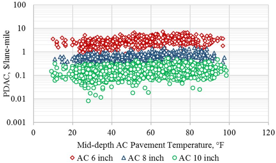
**Figure B.3. Fatigue cracking based PDAC output from Monte-Carlo simulations for Ely weather station.**
