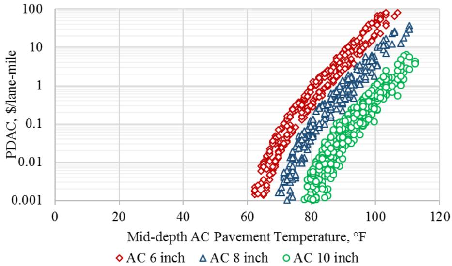
**Figure B.12. AC permanent deformation based PDAC output from Monte-Carlo simulations for Reno weather station.**
