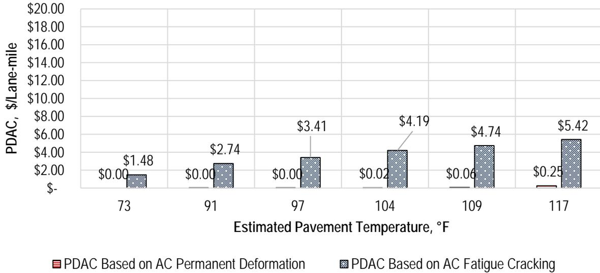
**Figure 7.7. OW vehicle PDAC values in US dollars per lane mile for Case study II (Interstate 15 Section).**
