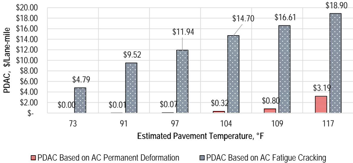
**Figure 7.9. OW vehicle PDAC values in US dollars per lane mile for Case study II (SR 146 Section).**
