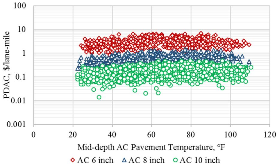
**Figure 5.5. AC fatigue cracking based PDAC output from Monte-Carlo simulations for Reno weather station.**
