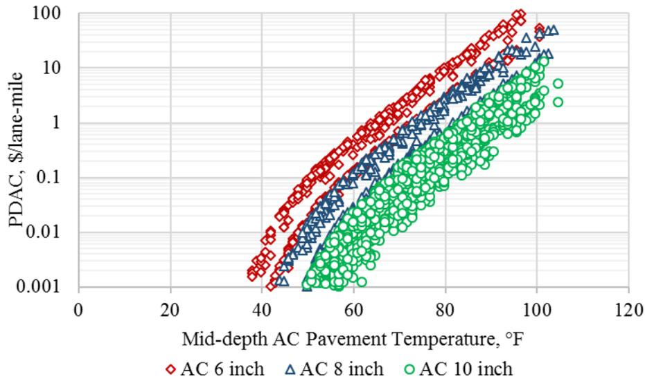
**Figure B.2. AC permanent deformation based PDAC output from Monte-Carlo simulations for Elko weather station.**
