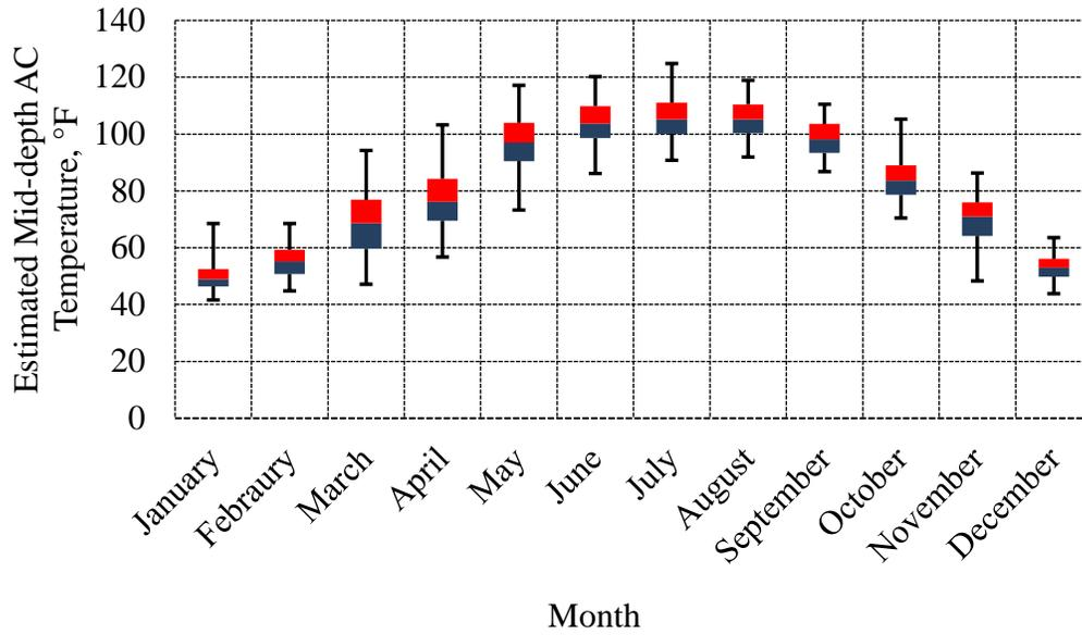
**Figure A. 3: Estimated Mid-depth AC temperature for Las Vegas station.**
