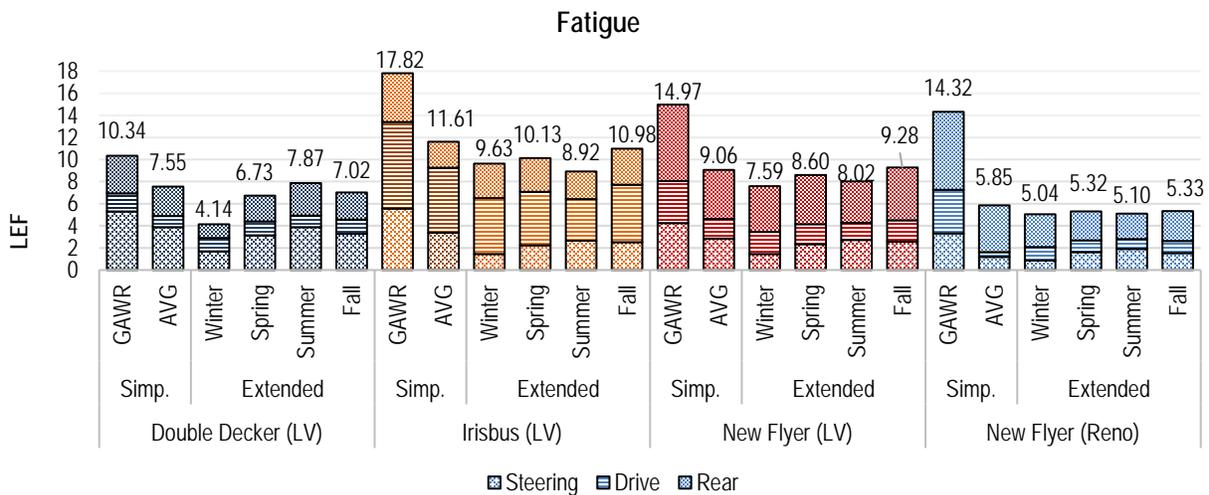
Figure 7.27. LEFs results based on AC fatigue cracking.
