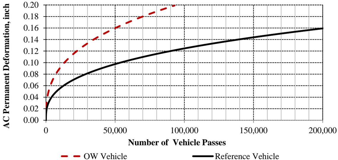
**Figure 2.8. AC permanent deformation damage curves under OW and reference vehicles.**
