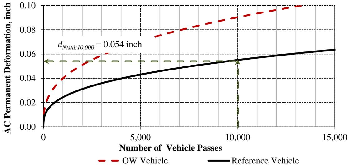
**Figure 2.10. AC permanent deformation after 10,000 passes of reference vehicle.**
