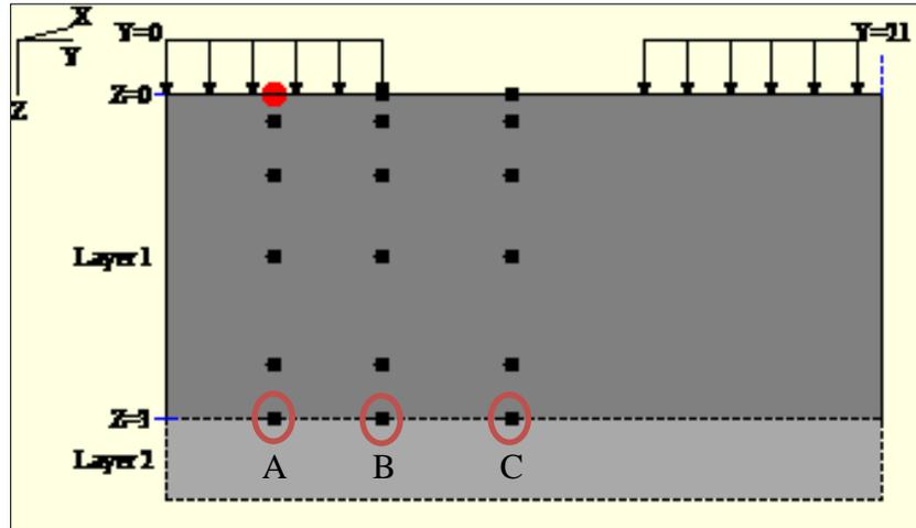
Figure 4.1. Schematic of 3D-Move analysis of a tandem axle group at six different pavement depths.
