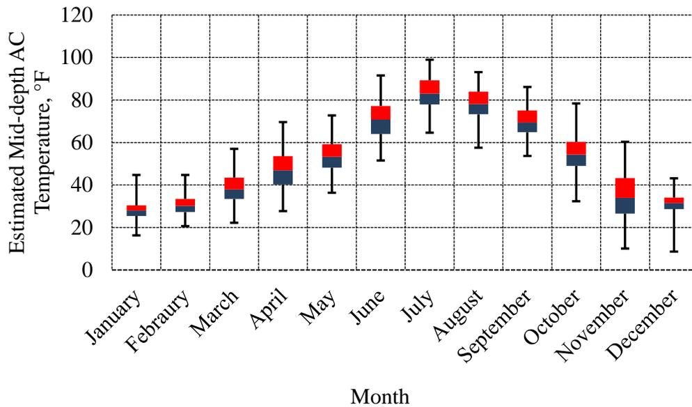
**Figure A. 2: Estimated Mid-depth AC temperature for Ely station.**
