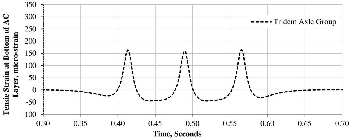
**Figure 2.3. Graph. Tensile strain response history at the bottom of AC layer for axle group B (tridem axle).**
