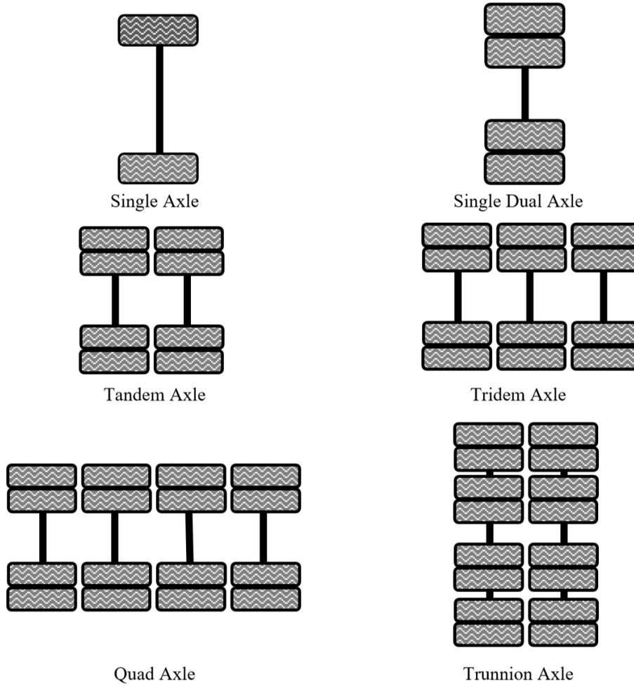
Figure 3.10. Identified axle group types in NDOT OW vehicle permits.
