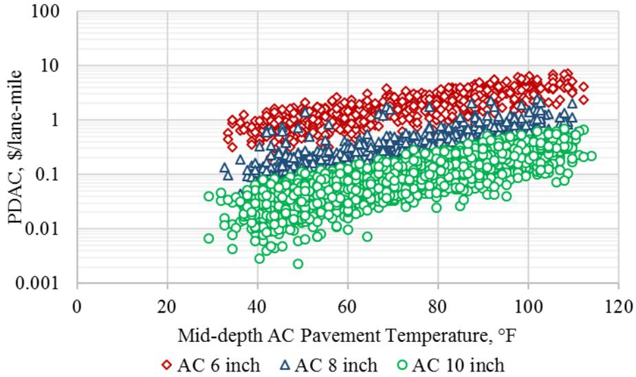
**Figure B.9. Fatigue cracking based PDAC output from Monte-Carlo simulations for Mercury weather station.**
